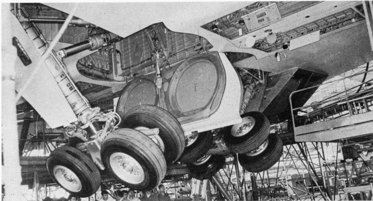
Main landing gear units being test-retracted on the ground.
