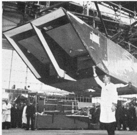
The under-wing variable-geometry engine air intake section monobloc for two of Concorde's Olympus engines on one side of the aircraft.
