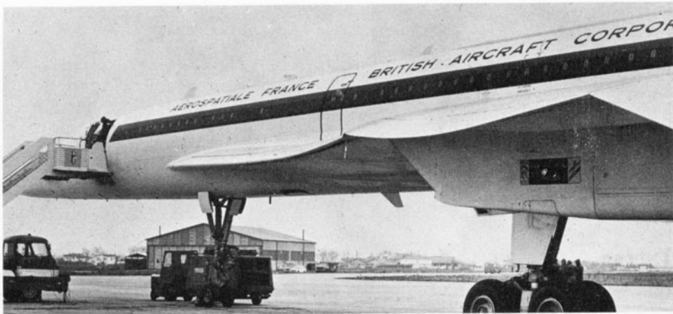
Concorde's sophisticated wing leading-edge shape—twice revised from the original during flight development.
