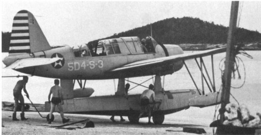
Subject of colour illustration No. 3 on the previous page, this OS2U-2 of Inshore Patrol Squadron VS-5D4 was based at NAS Cape May, N.J., in early 1942. This OS2U displays the rare combination of markings and paint scheme. Non-specular light-grey overall, white unit code letters and red and white tail stripes as directed by the Bureau of Aeronautics in January 1942 but some 2½ months after the grey-overall scheme had been abandoned. (Photo: via Harry S. Gann)
