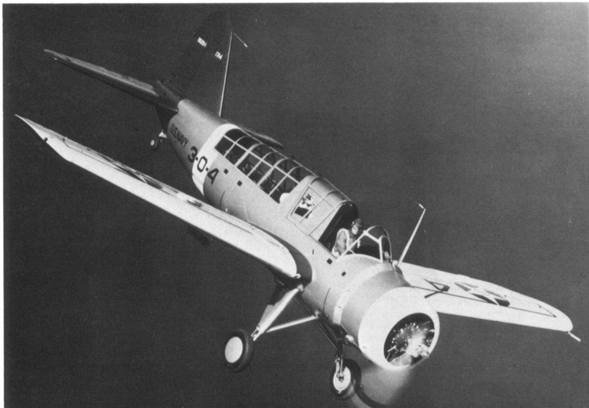
The 34th production OS2U-1 (BuNo.1714) in early 1941 before the change to drabber non-specular (non-reflecting) "warpaint" greys (from March '41) and blues. Markings reveal that this OS2U-1 was allocated to Observation Squadron Three (VO-3) aboard USS Mississippi (BB41) of Battleship Division Three, United States Fleet. VO-3's Disney-like emblem ("Oswald the Lucky Rabbit" riding a 16-inch shell) is located between the cockpits. Colour scheme: aluminium-varnished fuselage, white bands encircling motor cowling and rear fuselage and "True Blue" tail surfaces. Top surfaces to wings were orange-yellow and undersurfaces silver. Hamilton Standard 2-blade propeller silver but anti-dazzle rear faces; normal tri-colour tips (see photo above) with outer red, centre yellow and inner blue. This colourful display was of practical origin providing both ship-to-air identification and facilitating air-search recovery in the event of an out-of-sight emergency alighting. (Photo: Vought Aeronautics via authors)
