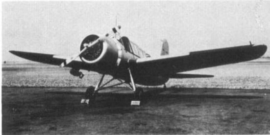
All "first-offs". (Top left, bottom right) Prototype XOS2U-1 (Bureau Number or serial BuNo.0951) in "dry" and "wet" forms and subsequent all-silver finish in 1938. This July 1938 view of the landplane shows Aldis-type telescopic gun-sight has been incorporated; similarly, floatplane now has the additional rear pylon strut to float which became wider on production models. Transparency curve amidships only applied to BuNo.0951. (Bottom left) May 1940 view of first production OS2U-1 (BuNo.1681) showing only one 100-lb. bomb in position on the two Mark XLI Mod.1 racks. (Top right) First production OS2U-2 (BuNo.2189) also in 1940. Aluminium varnish finish provides clear outlines to the Beisel lateral-control spoilers visible immediately aft of national insignia. (Photos: United Aircraft Corp. via Harry S. Gann and Lloyd S. Jones)
