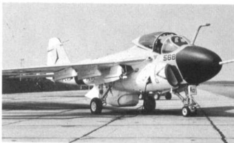
Standard ARM missiles. A-6B carrying General Dynamics Standard Anti-Radar Missiles on inner wing pylons takes off from Lindbergh Field, San Diego, Calif. 'Pock marks' on nose radome are small antennas. (Photo: General Dynamics)
