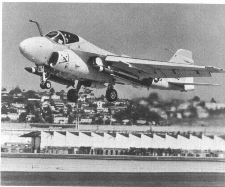
Standard ARM missiles. A-6B carrying General Dynamics Standard Anti-Radar Missiles on inner wing pylons takes off from Lindbergh Field, San Diego, Calif. 'Pock marks' on nose radome are small antennas. (Photo: General Dynamics)
