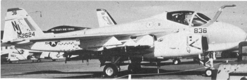
Golden Intruders, VA-128, are flying this A-6A which still has original fuselage speed brakes panels; the brakes no longer operate as is evidenced by paint that remains unburned. (Photo: Bob Labuoy)
