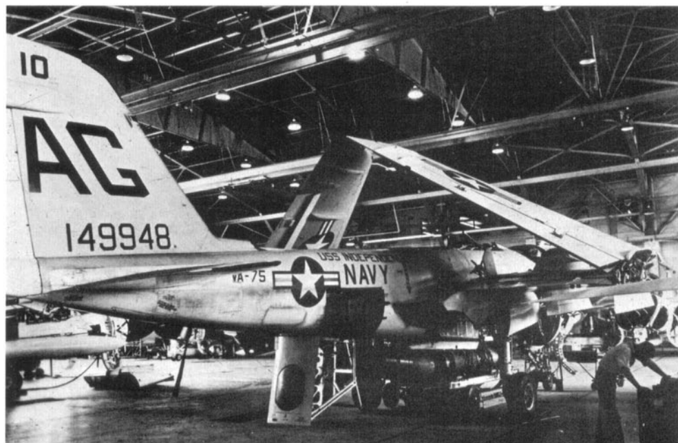
Maintenance. A-6A of VA-75 Sunday Punchers, CVW-7 (AG), with all systems down. Avionics 'birdcage' open below fuselage, starboard engine is out and ram air turbine on top of inside starboard wing is deployed. NAS Oceana 1964. (Photo: Grumman 64820)
