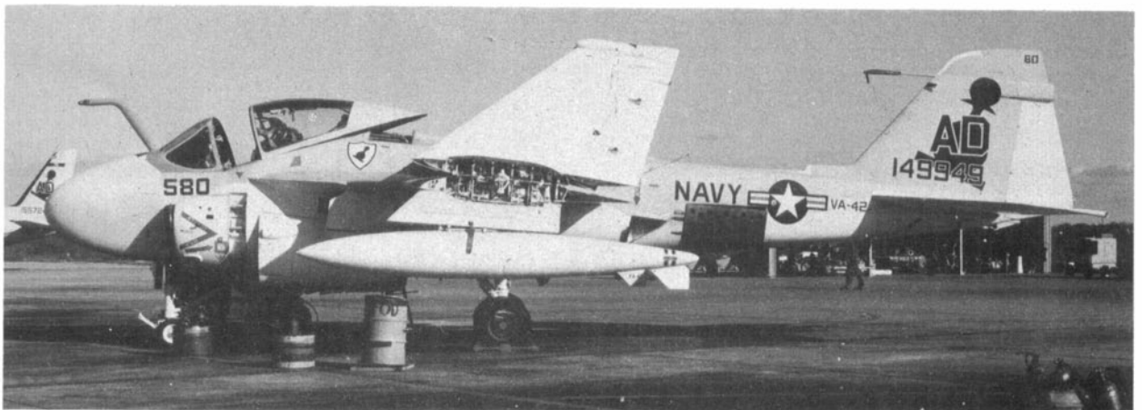
A-6B of VA-42 (AD) at NAS Oceana, Va. in December 1969. Rear fuselage brake is still operative. Drop tanks are 300-gal. units. Code AD is assigned directly to VA-42 Green Pawns since decommissioning of RCVW-4 in 1970. This coding also retained by other ex-RCVW-4 units. These are VA-174 (A-7 Corsairs) and VF-101 (F-4 Phantoms). (Photo: Author)
