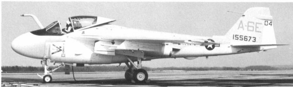
A-6E prototype. BuNo. 155673 is A-6A (shop 404) and was used to evaluate new avionic systems destined for production A-6Es. A-6E marking on fin is Grumman-originated and coloured light blue. (Photo: Grumman)
