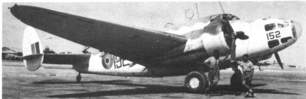
A-for-America and Lend-Lease; a Mark IIIA (FH314) at Fayid in Egypt, 1944. For local operating conditions, extra-large, Martin Baltimore-type, scoops replace the normal carburettor intakes on top of the cowlings. Exhaust flame-damper extensions are in evidence. (Photo: via Air-Britain)
