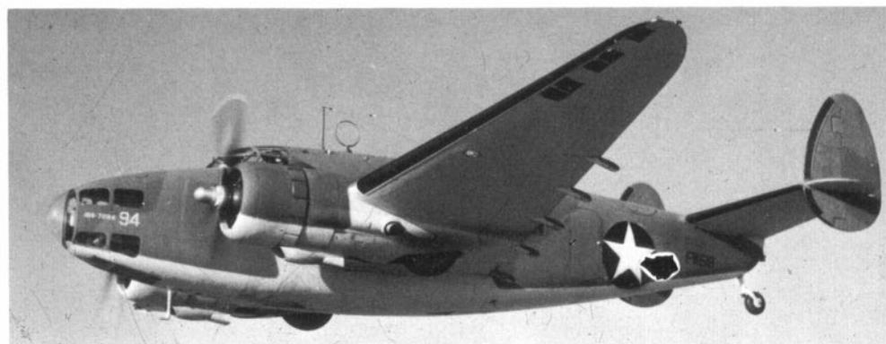
A USAAF-marked Hudson Mk VI (FK618) without turret and for use as a troop transport. The Lockheed assembly No. 414-7094 (with last two digits repeated twice size) appears on the nose section. All the A-28A/Mk VIs went to the RAF, RCAF and RNZAF. (Photo: Lockheed Aircraft Corp.)
