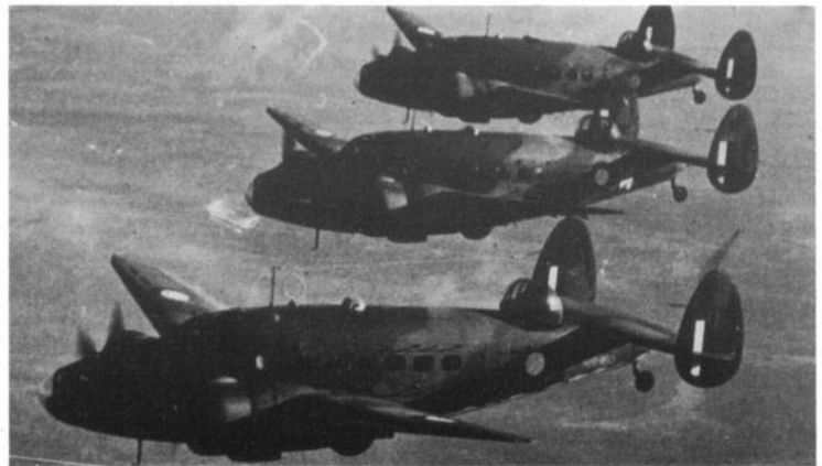
Hudson Mk IIIs of No. 2 Squadron, RAAF, flying over New Guinea in 1942; in foreground is A16-180, then A16-256 called Houdini and A16-236 named Foo. Above and below the last two windows to the rear are the antenna arrays of ASV Mk II; also in evidence in photo on the facing page, top right. (Photo: Frank F. Smith)
