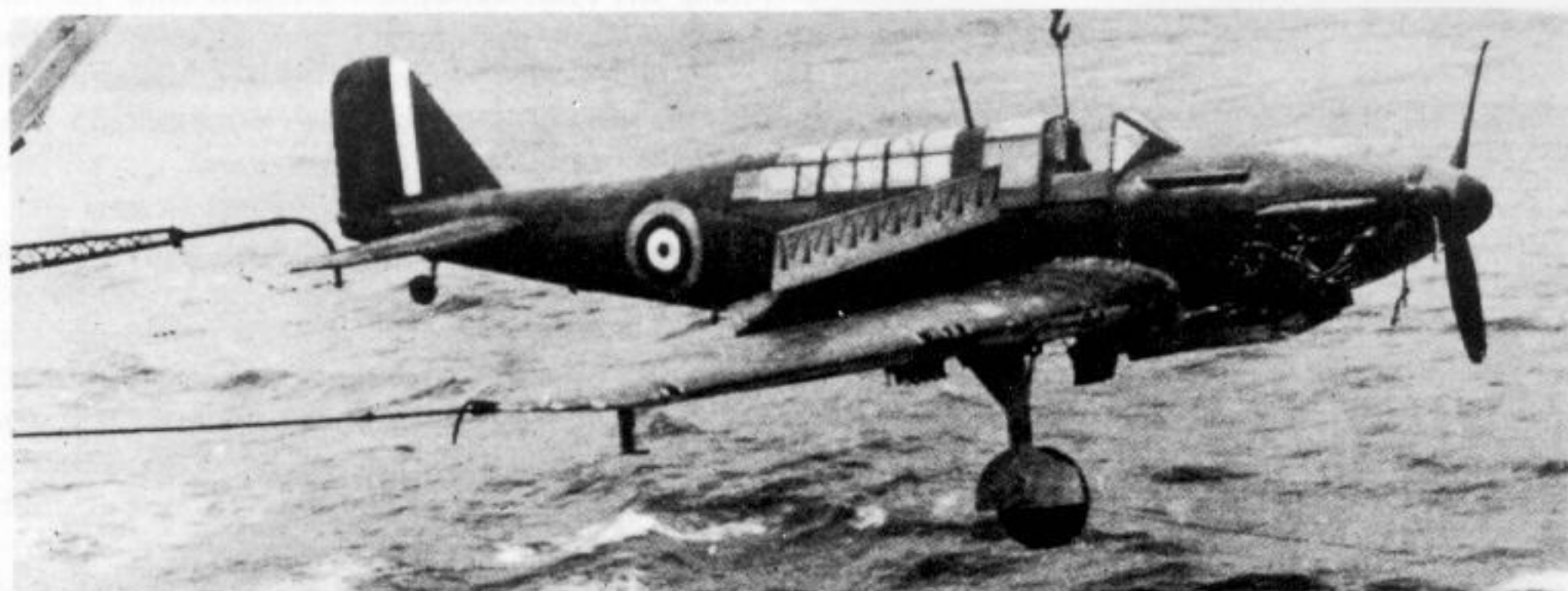
Every picture tells a story: An 808 Squadron Fulmar is suspended over the side by Ark Royal's crane, steadied by lines attached to wing tip and port wheel. The aircraft has been engaged by the barrier—hence the considerable damage to the underside of the engine cowling and radiator—and has been hoisted outboard to clear the landing area for other aircraft. Note that the flaps have not been closed before the trailing edge has been raised for folding. (Photo: via C. F. Shores)
