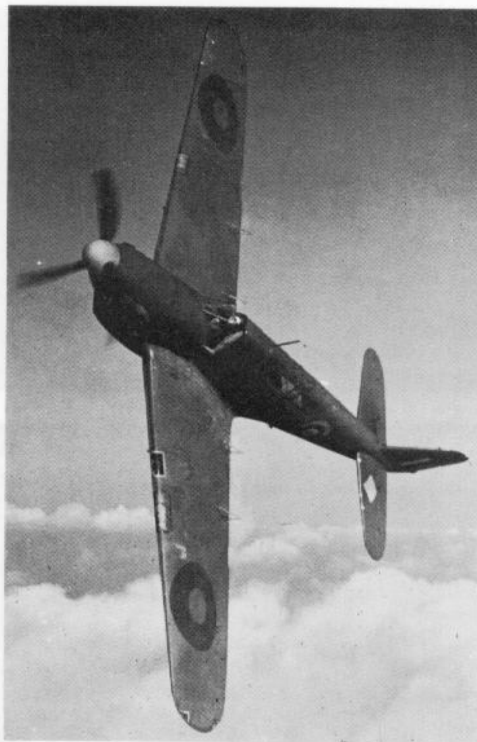
Fifth and final 'pre-production prototype' (N1858) in 1940 (Top view sensitive paint 'diamond' (poison gas detector) on tailplane) and in underside view, the two gun-bays with four cartridge (0.303-in) chutes, each inboard of roundels. The side view reveals the two sets of catapult spools and arrestor hook. This aircraft is fitted with four brackets on the wing trailing-edge connected with a trials installation of a typical Fairey-Youngman cruise/dive-brake flap—deleted by censor. (Photos flight International, ref. 18000-srs.)
