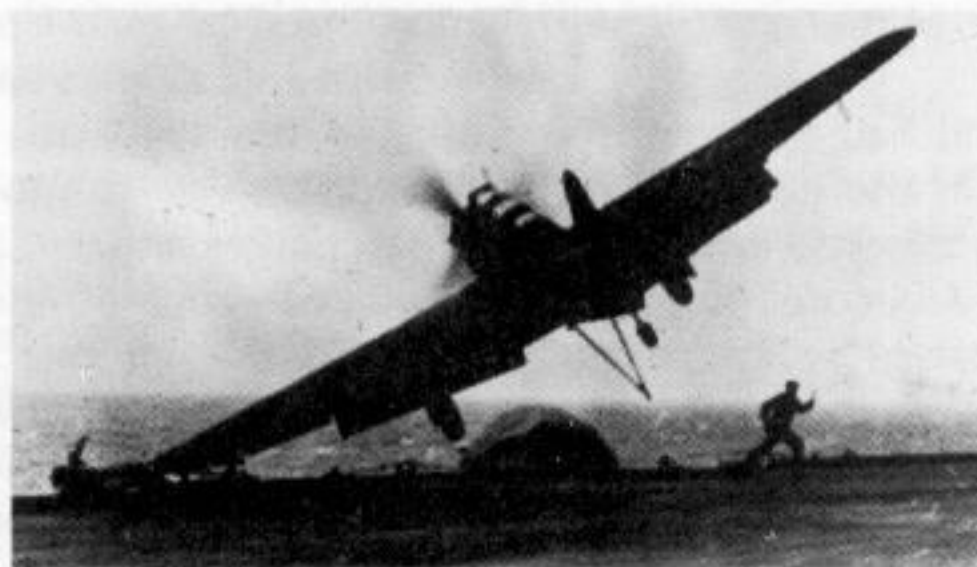
An Ark Royal Fulmar misses the arrester wires and swings to port in executing a 'round again' of which neither the landing signals officer (running clear) nor Commander (F) would have approved. (Photo: IWM, ref. ZZZ53170)
