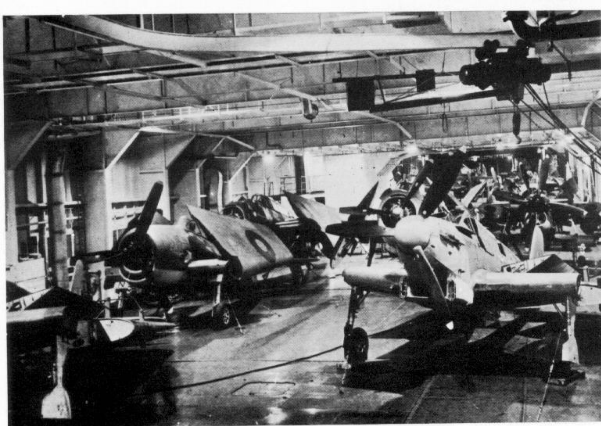
A pair of Fulmar Mk. NF. IIs of 784 Squadron occupy the foreground and assorted Hellcats, Avengers, and Barracudas of 768 Squadron the deck-landing training squadron – the centre and rear ground of Ravager's hangar. The three radar antenna pylons on each out-board mainplane can be seen on both Fulmars, and the two blast-tube openings for the 0.50-in Brownings can be made out on the left hand aircraft's port leading edge. (Photo: via R. Williams)
