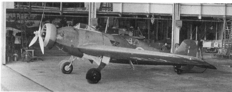
At Weybridge, K7721, the ninth production Wellesley is photographed on April 29, 1937, just inside the shed and showing off an unpainted DH/Hamilton Standard v-p. propeller unit. K7721 ultimately went to No. 148 (Bomber) Squadron and was written-off by crashing into a haystack on final approach, December 16, 1937. (Photo: Vickers, ref. 4955K)
