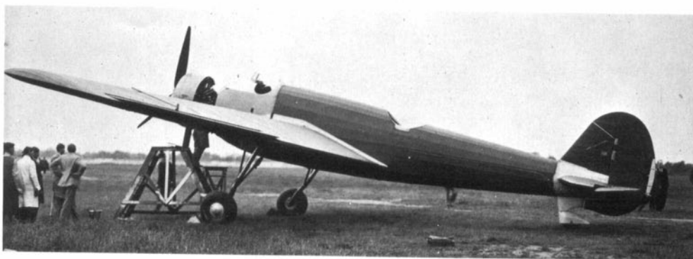
The Vickers PVO-9 or Type 246, the prototype which was to lead to the later Wellesley, is seen here at Brooklands in June 1935 with open cockpits, no markings and covered wheel wells and temporary fixed main undercarriage. (Photo: Vickers)
