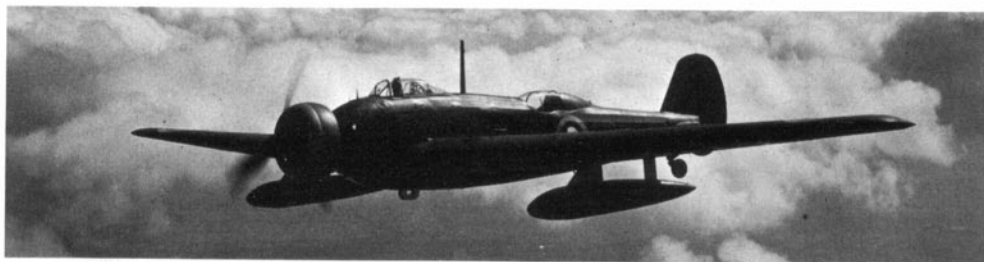
Study in cloudscapes. Previously illustrated in the shed, K7721 now displays the production-standard bomb containers providing space for two 500-lb or four 250-lb bombs in each pannier. (Photo: Charles E. Brown, ref. 5693-14)
