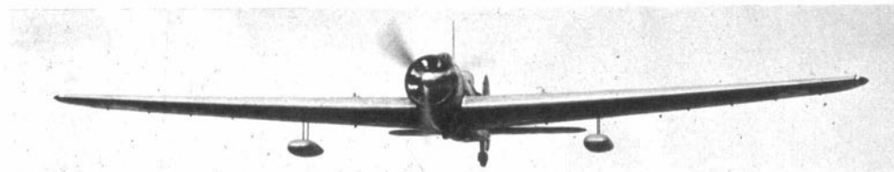
K7556 showing off the wide sweep of the high-aspect ratio wings which now support the earlier form of bomb panniers under the mainplanes. (Photo: 'Flight' ref. 12782S)
