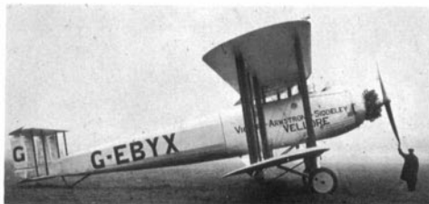
G-EBYX was a 2-seat freight and mail-carrying prototype, the Vickers Vellore, of 1928 which suggests the origins of the fuselage shape of the later, monoplane G.4/31 and Wellesley. (Below) The newly (1932) completed Vickers M.1/30 torpedo-bomber at Brooklands before application of military markings and RAF serial S1641. (Photos: Vickers (Aviation) Ltd.)
