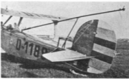
D-1189, a DVS-operated Flamingo, shows off the aero-towing rig which was tested at Brunswick in October 1931 by Robert Kronfeld. Special equipment was installed to measure glider-towing drag. For these tests, D-1189 was re-engined with a 175/95 h.p. Sh 14, to BFW U-12b standard. (Photo: "Der Segelflieger")
