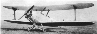
Of-POG (later Of-TOG) is an example of the Austrian-developed, Hammerle-designed U-12a. Most noticeable are the relatively small-diameter main wheels, the divided-axle undercarriage and more rounded fuselage. (Photo: via Ing. Fred Haubner)
