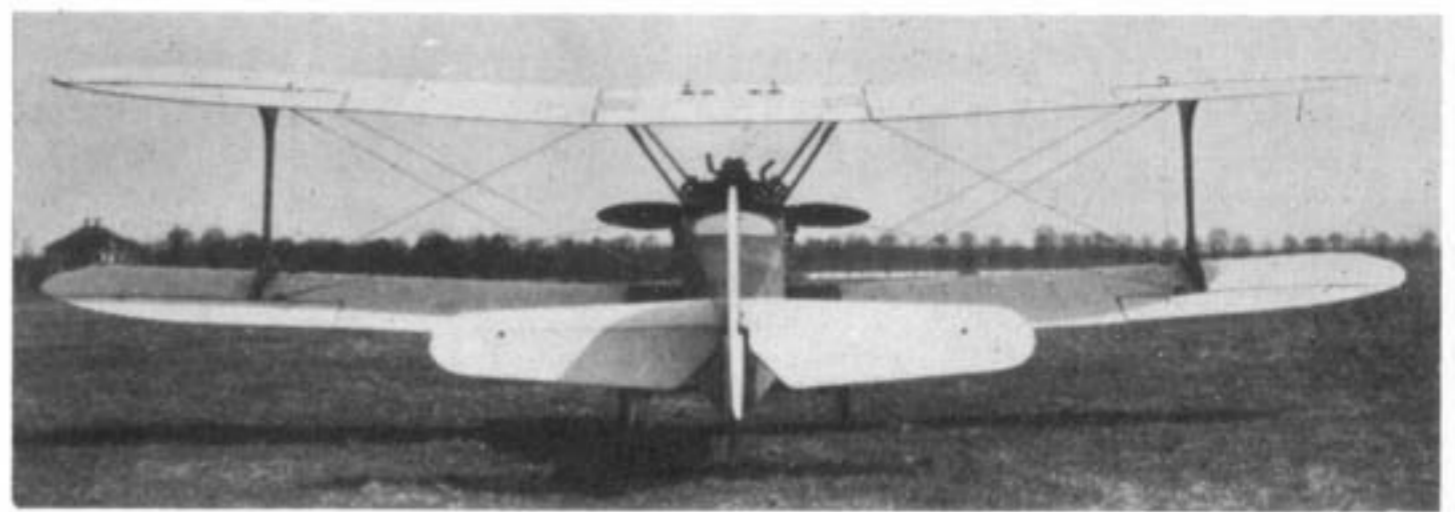
Udet U-12 prototype at Munich-Schleissheim, April 1925. The original small-area rudder and short-nose fuselage are apparent. (Photos: Udet Flugzeugbau GmbH, via Peter M. Bowers and Author's archives)
