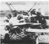
Hungarian Flamingo as a "lighter". Two nose-mounted, 8-mm machine-guns are clearly visible in this view of the locally-built Hungarian Variant V which was a basic lighter-trainer. (Photo: Aero Archiv Winkler-Budapest)
