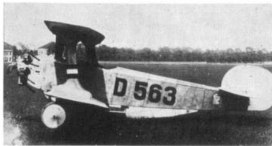
With Author's reservations, D-563 is believed to have been the prototype U-12, seen here with the bigger-area (elongated) rudder. The experimental container under the fuselage was used in supplies-dropping tests. (Photo: via Deutsches Museum)
