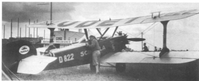
Udet in England, July 25, 1931. He was invited to give an exhibition of his aerobatic prowess at London's Heston Airport on the occasion of the annual King's Cup Race. Note the bench-type tabs above the ailerons for increased response in display flying. Man looking into cockpit is Udet's trusted mechanic, Erich Baier. (Photo: R. S. Allen)
