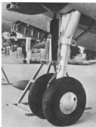
1 A close-up view of the revolutionary Kubicki main undercarriage leg of the P.37 bomber. (Photo: A. Morigala)
