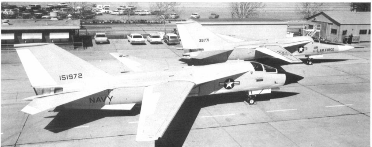
Longer nose wins! Meeting on the ramp in June 1967 in Texas at the Fort Worth plant of General Dynamics—the long-nose Air Force version, the sixth F-111A (AF:63-9771) meets the 7-ft. shorter Navy F-111B (BuNo. 151972), the third built. (Photo: GD/FW, ref. 30-30659)
