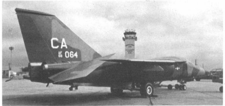
A TAC F-111E (AF-68-0064; 74th built) photographed in 1971 and wearing the old tail coding of "CA" (now "CC") of the Cannon AFB, New Mexico-based 27th TFS, 20th TFW, TAC. From the rear, the massive tail assembly including one-piece "slab" horizontal surfaces are impressive; "064" is merely visiting Bergstrom AFB, Texas. (Photo: Jay Miller)
