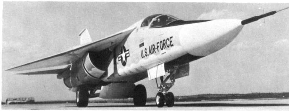
Low-angle portrait of an early GD/FW F-111A reveals the variable-geometry intake "spike" or quarter-circle centrebody which controls air flow to face of the jet engine compressor as a function of Mach No. Translating cowl is also partially open. (Photo: GD/FW, ref. 30-27337)
