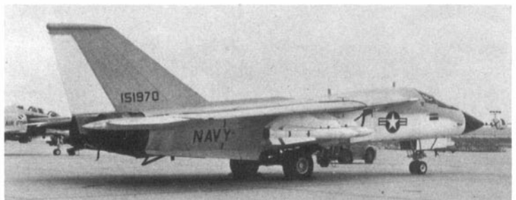
The US Navy prototype GD/Grumman F-111B (BuNo. 151970) was still going strong on May 19, 1968 at Edwards (now Flight Research Center) three years and one day after its first flight. Underwing ordnance comprises experimental-prefixed Hughes XAIM-54A Phoenix missiles. (Photo: Duane Kasulka)
