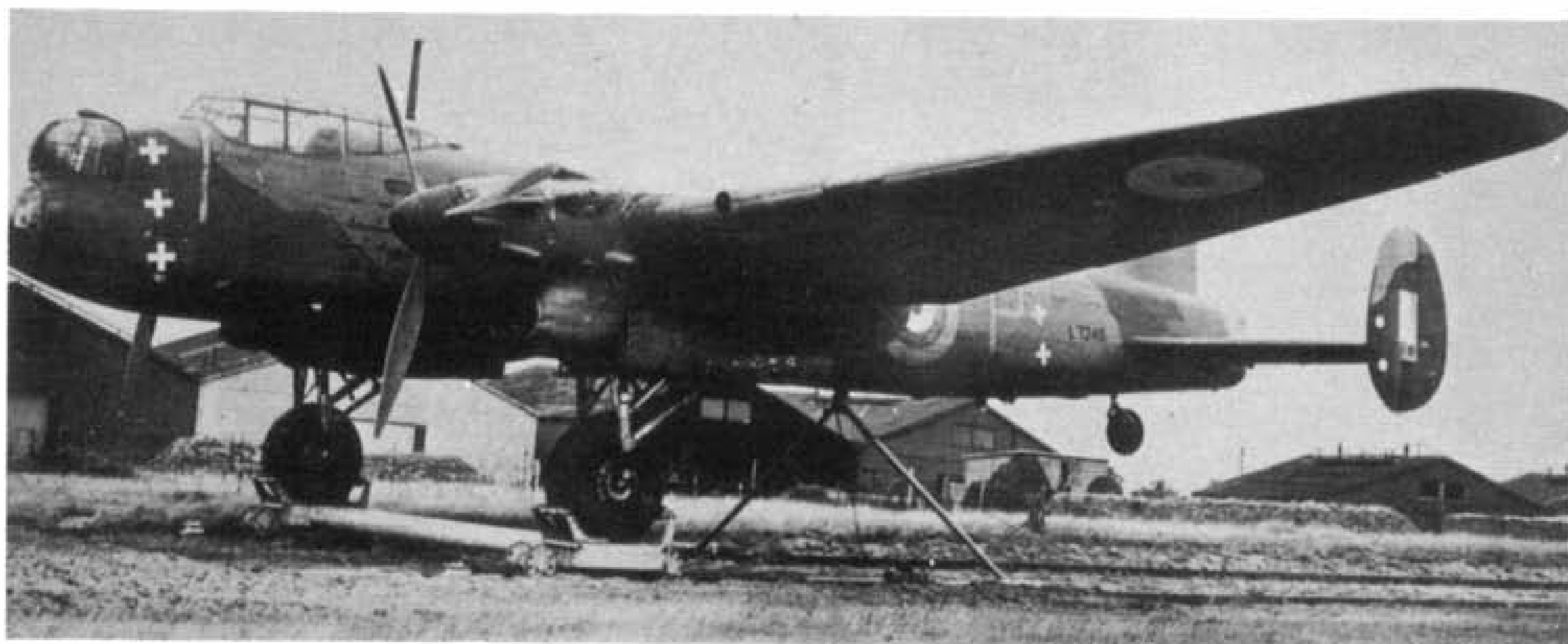
Prototype (L7246) now fitted with nose and tail power-operated gun turrets and rigged for catapult-assisted take-off trials at RAE, Farnborough (Hampshire) where it became resident in August 1940. Behind the fuselage roundel is the obligatory yellow "P" (prototype) in a thin yellow circle. Fore and aft series of crosses were applied for photo-measuring purposes. (Photo: via R.C.B. Ashworth)
