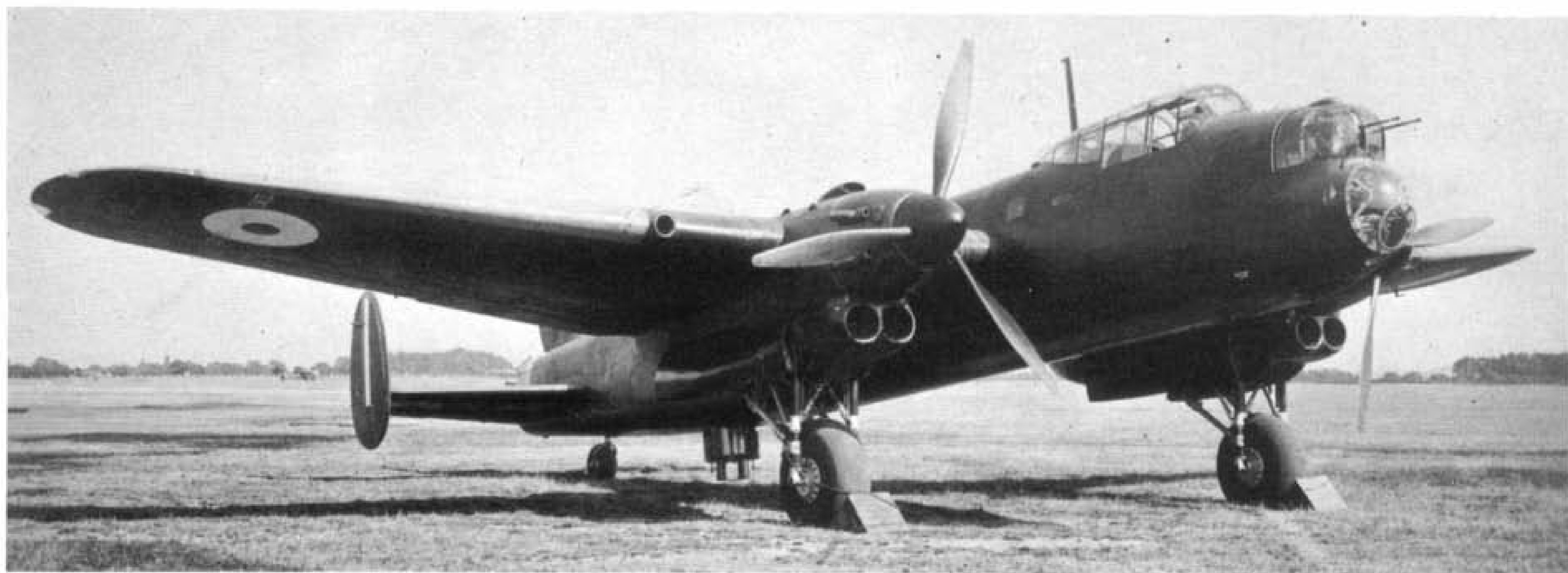
Number two prototype (L7247) shortly after its first flight on May 26, 1940. The FN21A ventral "dustbin" is shown in the fully extended position. Photo taken at A&AEE, otherwise RAF Boscombe Down. (Photo: Crown Copyright Reserved, ref. 10336A)
