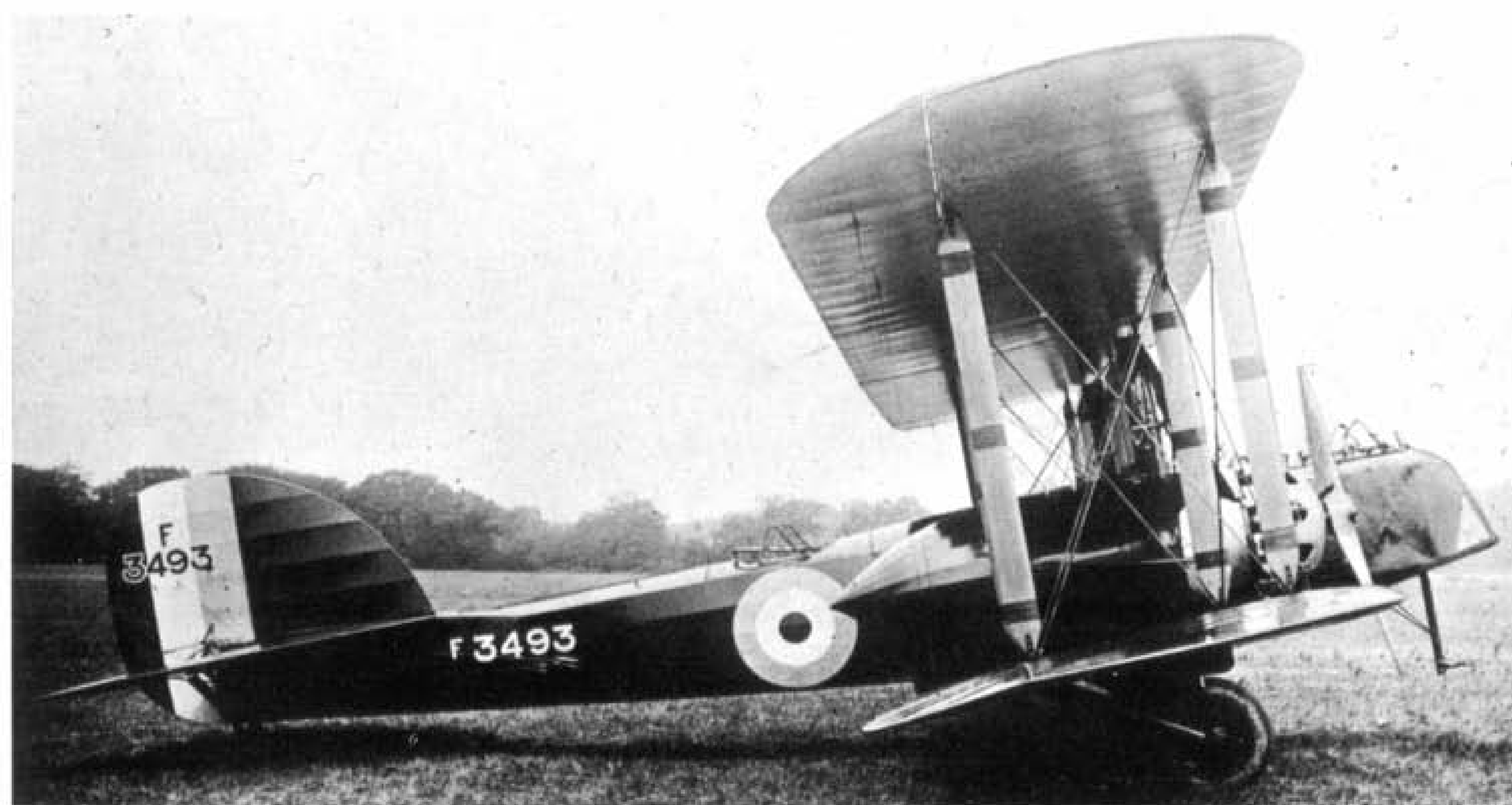
One of the original Avro Manchesters, the Type 533 of 1918, powered by two 320 h.p. ABC Dragonfly engines. Because of the Armistice only two of these power variants were completed, F3493 illustrated and F3494. The first, however, was a Puma-powered prototype, F3492. (Photo: Avro via Author)
