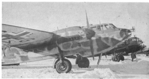
Lack of flame dampers on the Do 217 N's exhaust ports suggests the aircraft was employed in a training role. On the nose is the Lichtenstein aerial array. Behind the Do 217 N is a Do 217 K.
