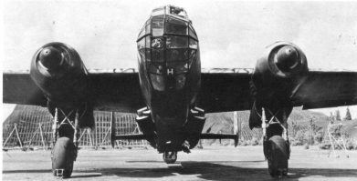
Head-on view of the Do 217 E-2, coded "HN", illustrated at the foot of the facing page. The Bomberklappen (bomb doors) show their unusual method of "sandwiching" in the open position. (Photo: Bundesarchiv, ref. 483-2882-6a)
