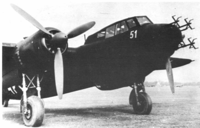
The big-span Do 217 K-2 with extra wing area required to fit the "Fritz-X" guided-bomb. Along the mainplane leading-edges are the total of six supporting posts for the horizontal wire aerials of the Lichtenstein radar. The fixed, forward-firing battery comprised four each of 20-mm MG FF cannon and 7.9-mm MG 17 machine-guns. Because the performance compared unfavourably with other night-lighters, most Do 217s became operational trainers. (Photo: Dornier)
