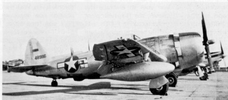
Outwardly the P-47N-20-RE was identical to aircraft in the previous production block. This one has 300 US gallon drop-tanks on the wing bomb racks, doubling the fuel load for long range flights. (Photo: Roger F. Besecker)
