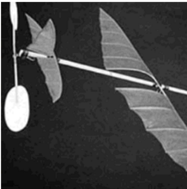
Model with automatic rudder. a a , elastic aero-plane; c c , aerial screw centred at f ; d , frame support; e , india-rubber, in a state of torsion, attached to the aerial screw. By holding the aero-plane ( a a ) and turning the aerial screw, the rudder is obtained by torsion. (M. Pénauud, 1872.)
