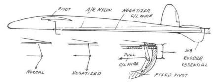
Pull on tow line causes toggle to straighten up and thus lift stabilizer up 1/16 to 1/8 in. IMPORTANT; Auto Rudder must be centralised before NEGATISER begins to act, i.e., negatising cable is slack when Auto Rudder cable is tight.
