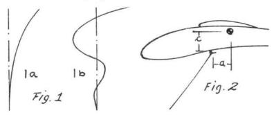
Sketch 1a shows divergencies. The model veers off to one side and just keeps going to the same side at an increasing rate. (Note that if the model is trimmed to go straight it could fall off on either side. If there is a warp or slight circle remaining it will usually go in that direction.
