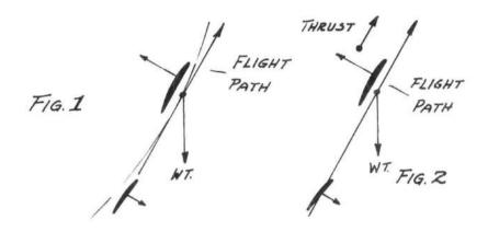
The position of the wing relative to the tail will be determined by the best gliding performance, when the wing is up at 10<sup>9</sup> or 12<sup>°</sup> degrees, of course. Now we seem to have the forces and moments balanced in the longitudinal plane.
