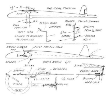
On the tow the Sorbo Rubber Pad interrupts the clockwork motor, i.e. impinges on the light balance wheel. On release of model at end of tow, the clockwork starts. Original timer is ex W/D and can be slowed down by soldering extra weight on the flywheel arms. Up to 4 min. possible.
