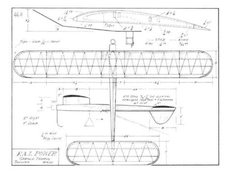
Most fellows have trouble with VTOs. I found that very consistant take-offs can be had by pointing the right wing into the wind (with model having right climb adjustments). This minimizes the tendency of the model to flip on its back. The wind tends to lift up the right wing rather than letting it come in the right with its power circle.
