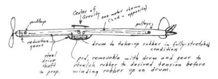
In either a tension-drive or the customary direct torque-drixemodel, the propeller will experience a considerable variation in driving torque. Since the propeller is basically most efficient at "one" operating speed (but what is it?) it might be desirable to reduce the initial torque or "power burst" and stretch out timewise and prop turnwise this initial unwinding or unloading of the rubber motor. For the direct torque drive we might use the following device:
