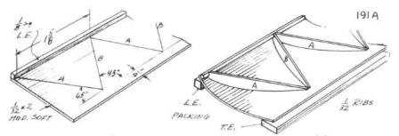
NOTE: PIN L.E. & T.E. PACKING DOWN WHEN A RIBS ARE INSERTED. THEY ARE PINNE RIGHT THRU THE 32 SHEET. THIS ESTABLISHES THE CONTOUR & HOLDS DOWN THE SET-UP
