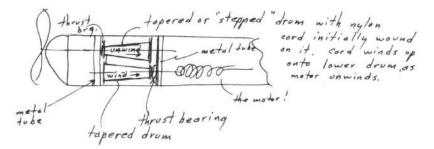
A similar scheme could be incorporated in the tension drive ship by using a stepped drum.
