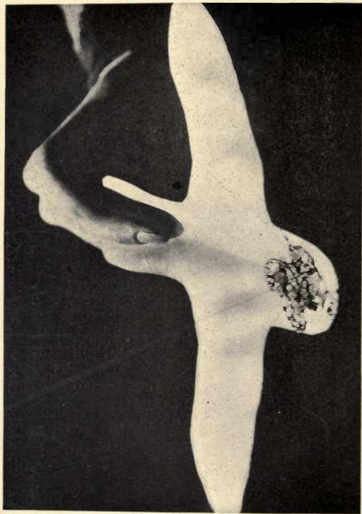
The First Glider Weighted at the Front.
