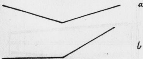
FIG. 19A. A dihedral supporting surface. In this case the two halves of the "plane" are set at an obtuse angle to one another. FIG. 19B. The dihedral aerofoil resists the torque of a single screw by giving more lifting effect on the wing which the torque, due to the reaction of the screw, tends to depress.
