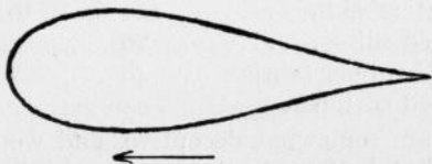
FIG. 77. Aerostat of approximately correct form.
