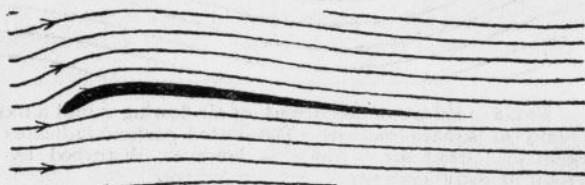
FIG. 10. Effect of flow round a body of a shape approximating to stream-line form.
