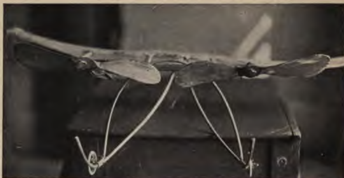
Illustrating the proper position of right and left propellers
