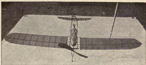
Schober pusher type compressed air driven monoplane
