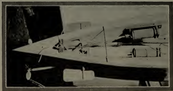
Fig. 212—The complete rudder mechanism, showing the solenoids
