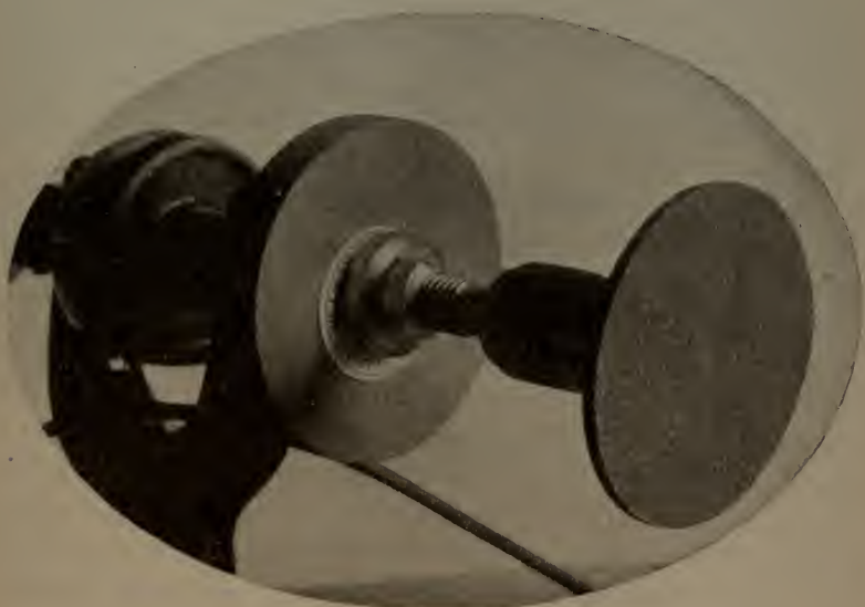
Fig. 61—The grinding disc shown in Fig. 57 attached to a grinding head
