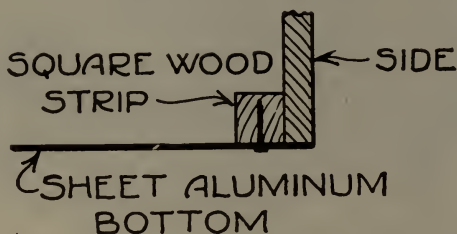
Fig. 165—Showing how the aluminum bottom is held to the sides of the hull
