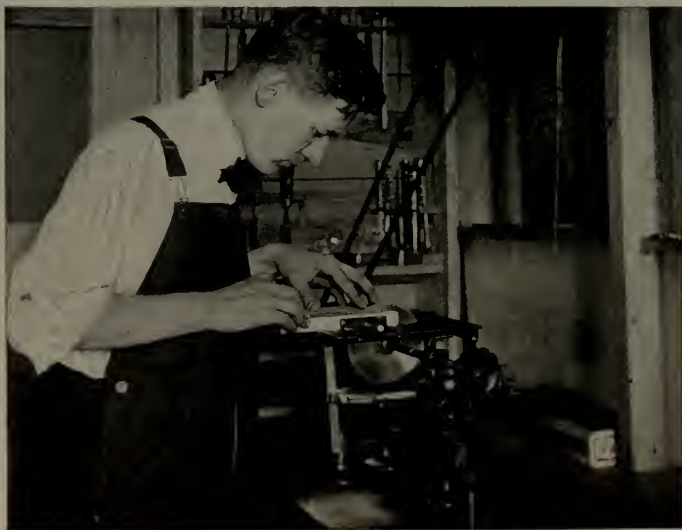
Fig. 8—Using a sawing attachment on the lathe shown in Fig. 7
