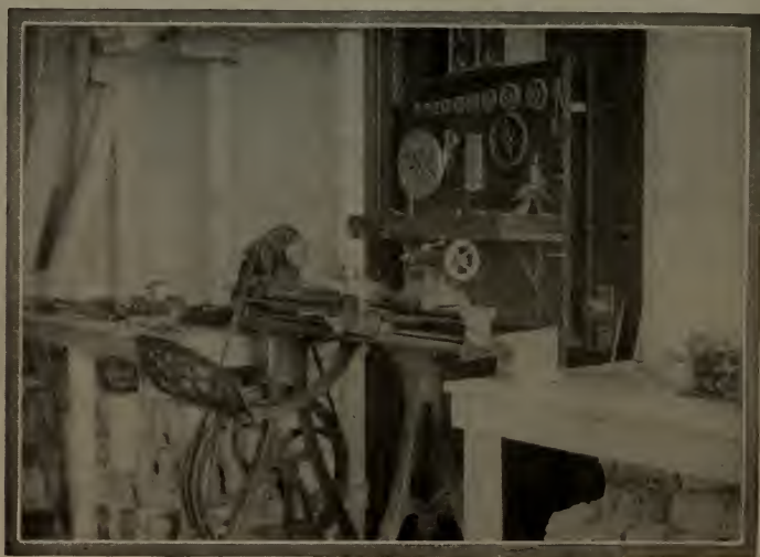
Fig. 5—A small engine lathe with attachments mounted on the wall where they will be convenient
