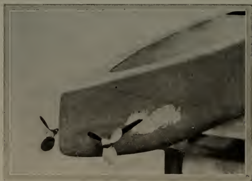
Fig. 205—The stern of the hull, showing propellers in place
