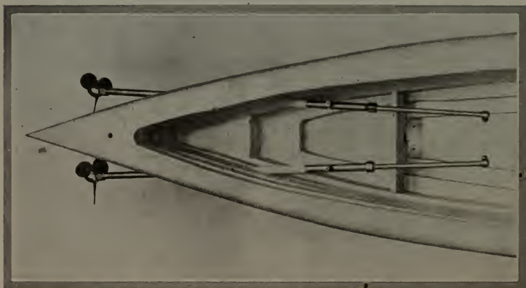
Fig. 204—The stern of the hull, showing how the propeller shafts pass through
