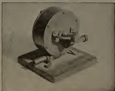
Fig. 135—The turbine, showing the exhaust port
