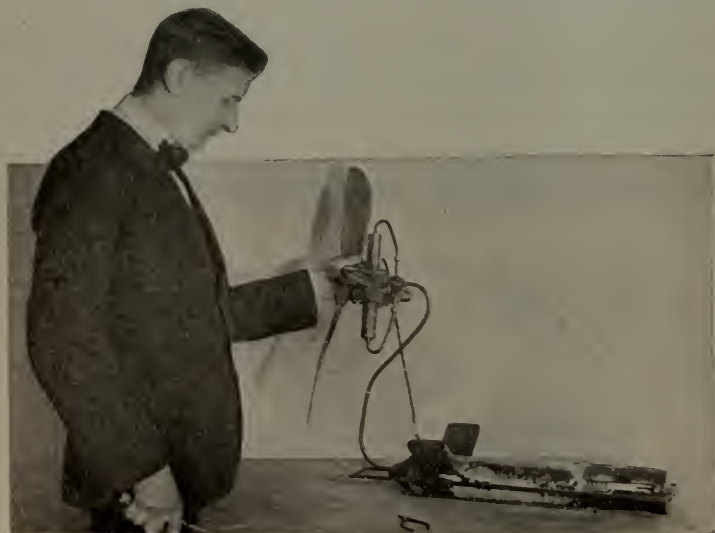
Fig. 117—The four-cylinder engine and its flash boiler
