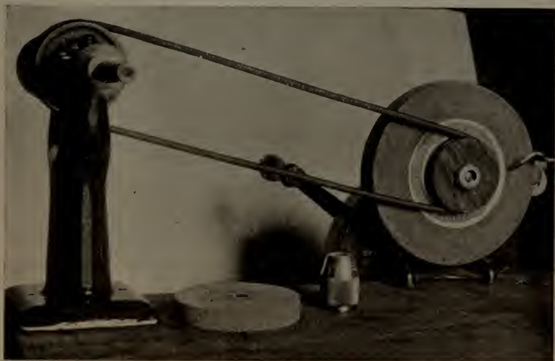
Fig. 60—Driving a grinding head with a hand grinder
