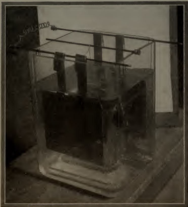
Fig. 88—A glass storage battery jar used as an electro-plating vat
