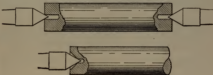
Fig. 12—Two examples of improper centering
