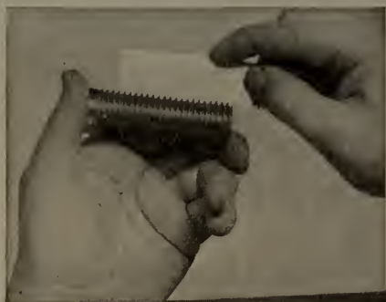
Fig. 28—Testing threads with a small pocket gauge
