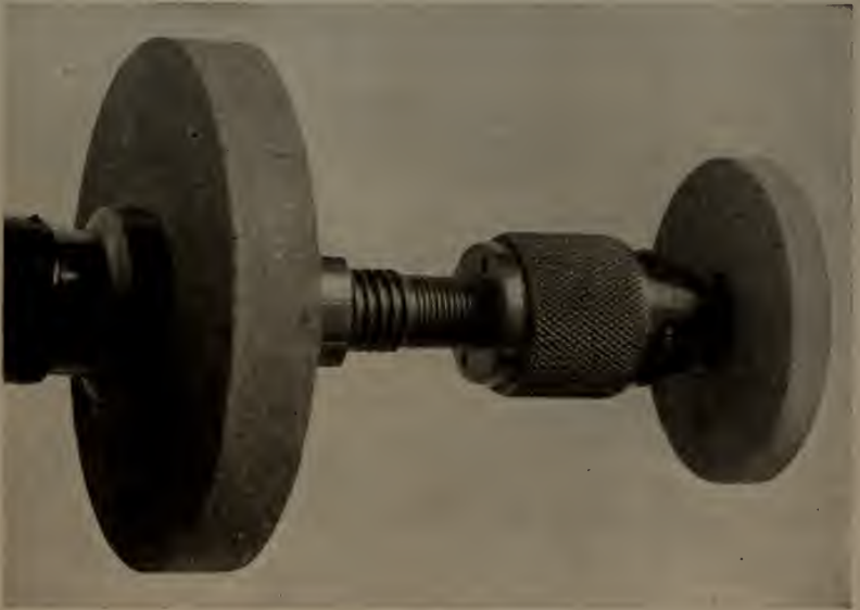
Fig. 56—How a jeweler's wheel can be used in the chuck of a small grinding head
