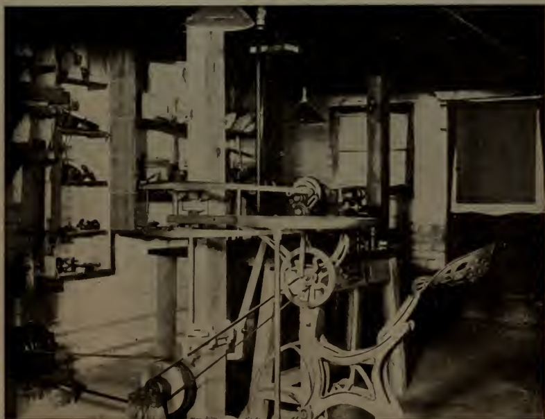
Fig. 2—A power-driven jig-saw in a workshop
