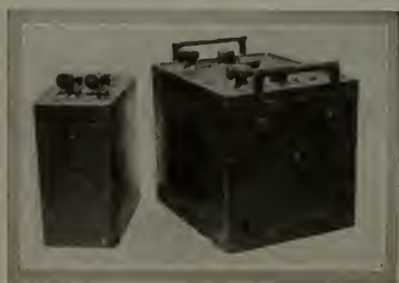
Fig. 198—The storage batteries used on the submarine
