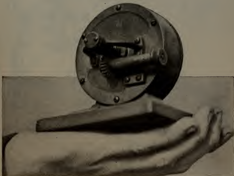
Fig. 133—The complete steam turbine, showing its comparative size
