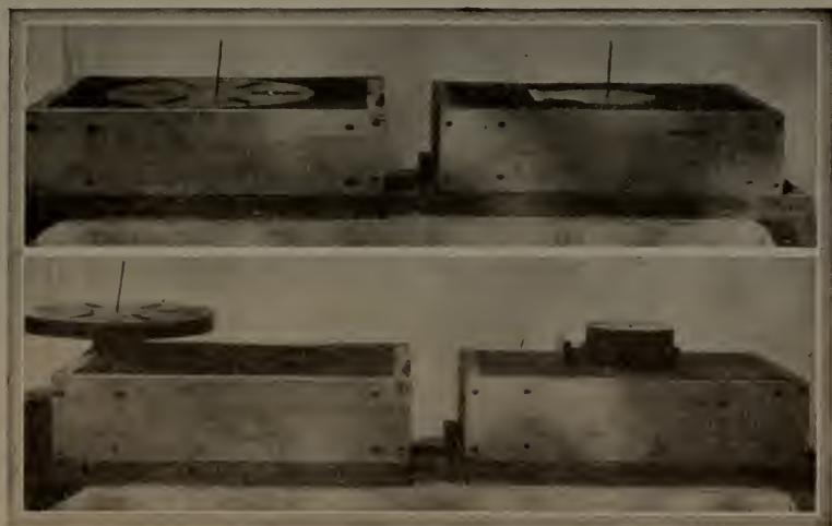
Fig. 64—(Above). Pattern exposed and piece moulded in place
