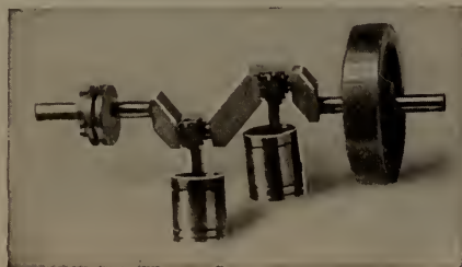
Fig. 98—The completed crankshaft for the engine, with flywheel, pistons and eccentric mounted in place
