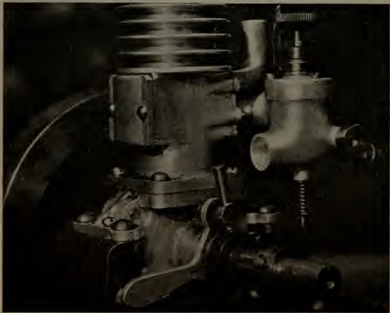
Fig. 275—A close-up view of the timing device and carburetor
