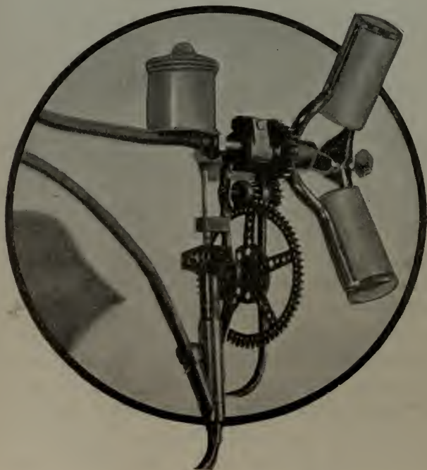
Fig. 125—The three-cylinder engine mounted on a model airplane
