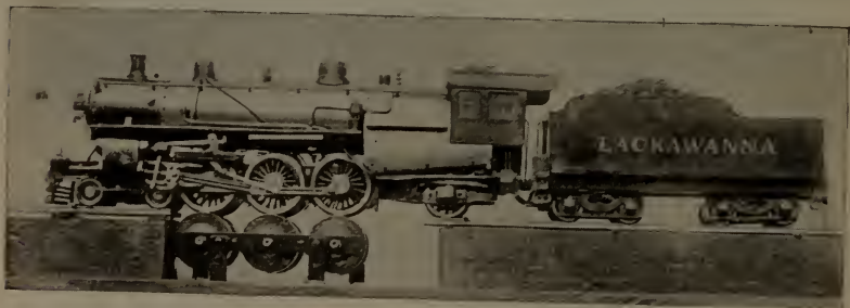
Fig. 283—The locomotive mounted upon its testing stand
