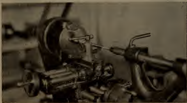
Fig. 16—Turning down a small steel rod
