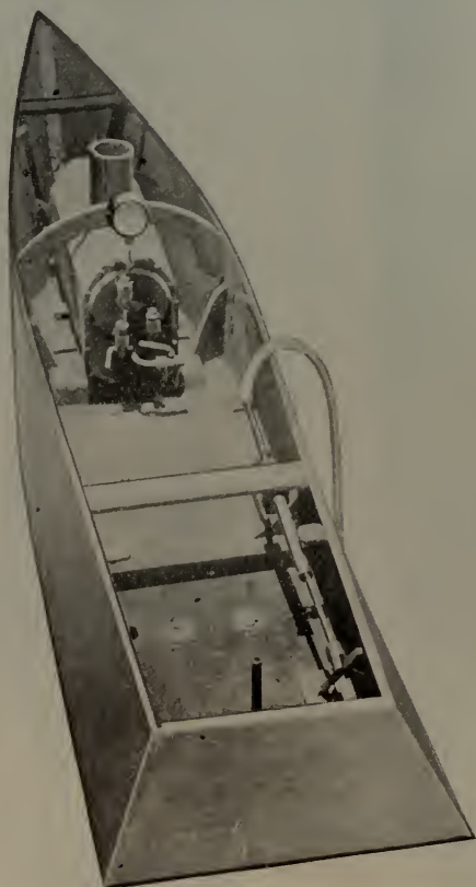
Fig. 179—The boat with the deck removed. The hand water pump is shown at the right
