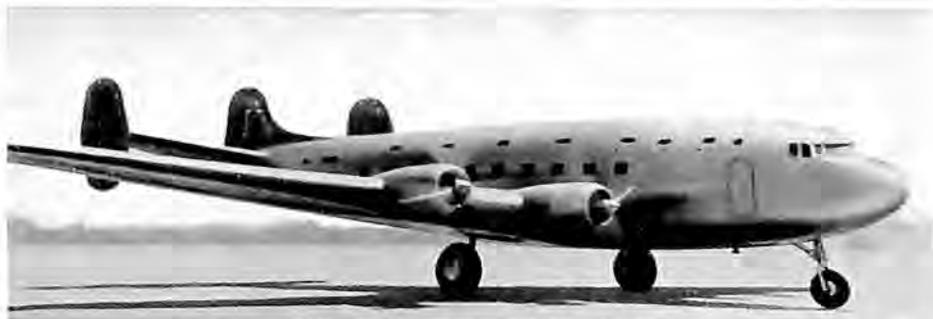
This small model of the new four-engine air liner shows the tricycle landing gear. The prototype will be powered by Pratt & Whitney Twin Hornets.
