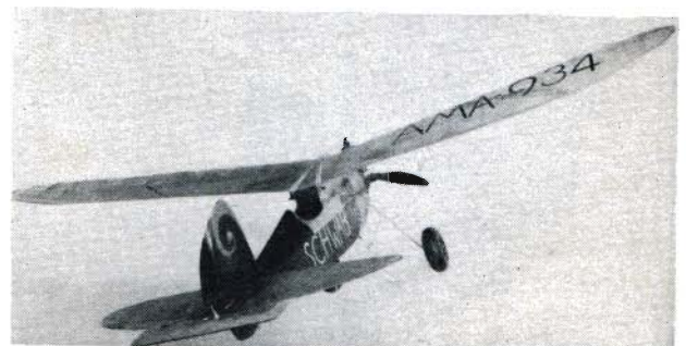
Controls on the tail operated by wires
