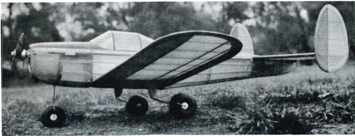
A three wheel landing gear provides fine takeoffs and landings
