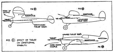
under power, which may make the model stall on the glide, or, if adjusted for glide, may cause a dive under power. Slight upthrust is indicated here to cure this fault.
