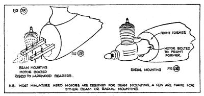
The whole motor mount unit, which is shown built up from ply and birch in the diagrams, can be cast in light metal, such as electron, or can be of mixed wood and metal construction. For example, the webs, shown of ply, could be of aluminium with pressed flanges for greater rigidity.
