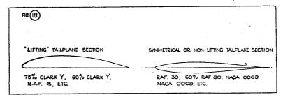
Structurally a tailplane with an aerofoil section having a flat undersurface is to be preferred, since this can be built flat on the working board and easily checked for warps, etc. Thus even with a "nonlifting" tail a section with a flat undersurface and cambered upper surface should be used, rigged as shown in Fig. 3/2.
