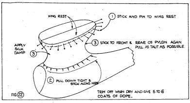
For fairing-in the pylon on such types silk is the only suitable medium, although other materials can be used in an emergency. The application of silk covering to a pylon wing mount is shown in Fig. 22. The silk should be applied damp, one piece for each side, and stuck to top and bottom with thin Durofix. Make sure that it remains securely stuck whilst drying. By applying five or six coats of dope to this covering the result is an amazingly strong and rigid structure.
