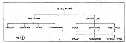
There are two main classes of petrol models:—(i) free flying models and (ii) control line models, of which only the former concern us here Free flying petrol models generally fall into one of four types, viz.:—
