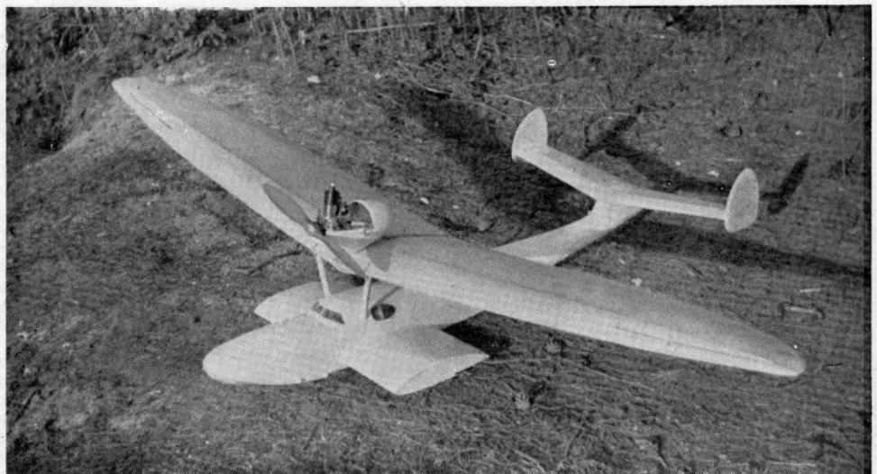
FIG. 78 (above).—The Author's 7 ft. 6 in. span experimental float plane with 9 c.c. Brown Junior Engine.
