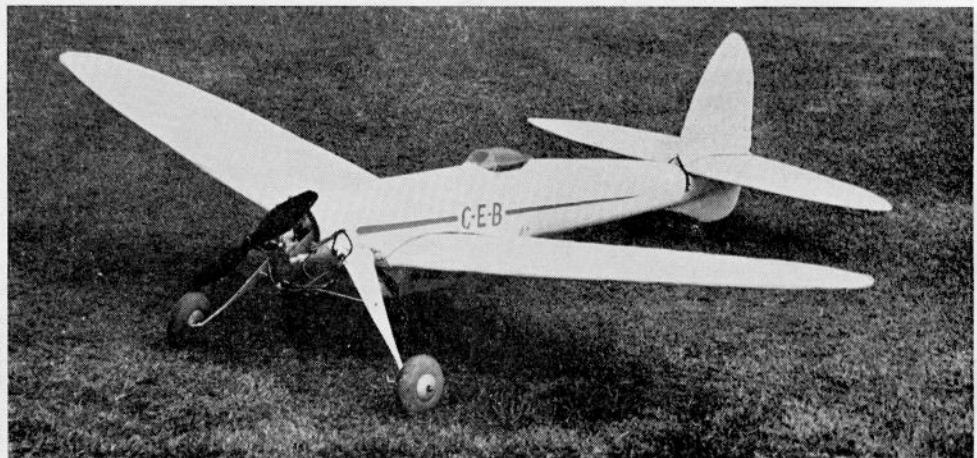
Fig. 85.—A Small low wing petrol model made by the author with dummy radiator containing all the electrical gear slung beneath the centre section.
