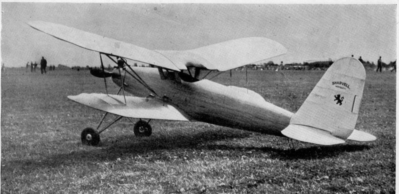
FIG. 91.—Mr. Sharwell's balsa planked petrol model biplane.
