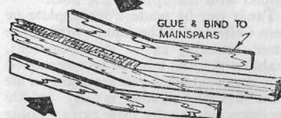
Fig. 8.—Plywood spar braces are essential, and on larger models may also be fitted to leading and trailing edges.
