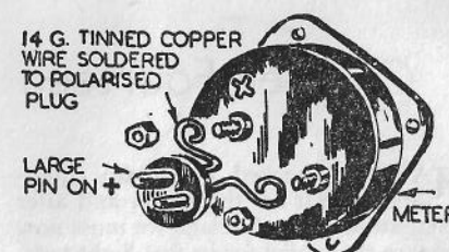
FIG. 3.—Simplest method of adapting the ordinary 0.5 millimeter is by means of two short lengths of 14 gauge tinned copper wire. The ends are soldered directly into a two pin polarised plug, the rigidity of the wire being sufficient to keep the meter in position.
