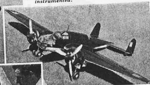
Below: Z. Wojda's highly detailed Championship Cup winner, a c.l. version of the Polish PZL 37. U.c. is fully sprung and working. Flaps operate and cockpit is instrumented.
