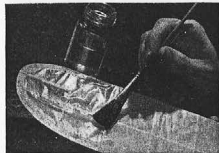
Doped with a mop brush, the fine taut wing covering looks slack, but soon shrinks again.
