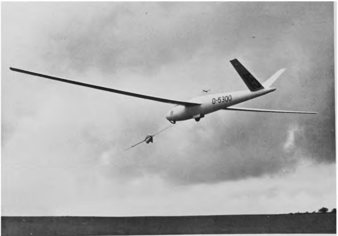
The German H.K.S.I. An experimental high performance glider with laminar flow wings, and tail parachute instead of air brakes. Flown by E. G. Haase in the World Gliding Championships, 1954.
