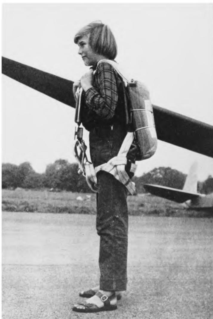
11. He clips the four straps into the locking box. This box has a quick-release mechanism in case the pilot is dragged by the wind on landing and wants to get rid of his parachute urgently. All that is necessary is to twist and bang the box, and the parachute harness will fall off. The rip-cord handle for opening the parachute can be seen below the left shoulder.
