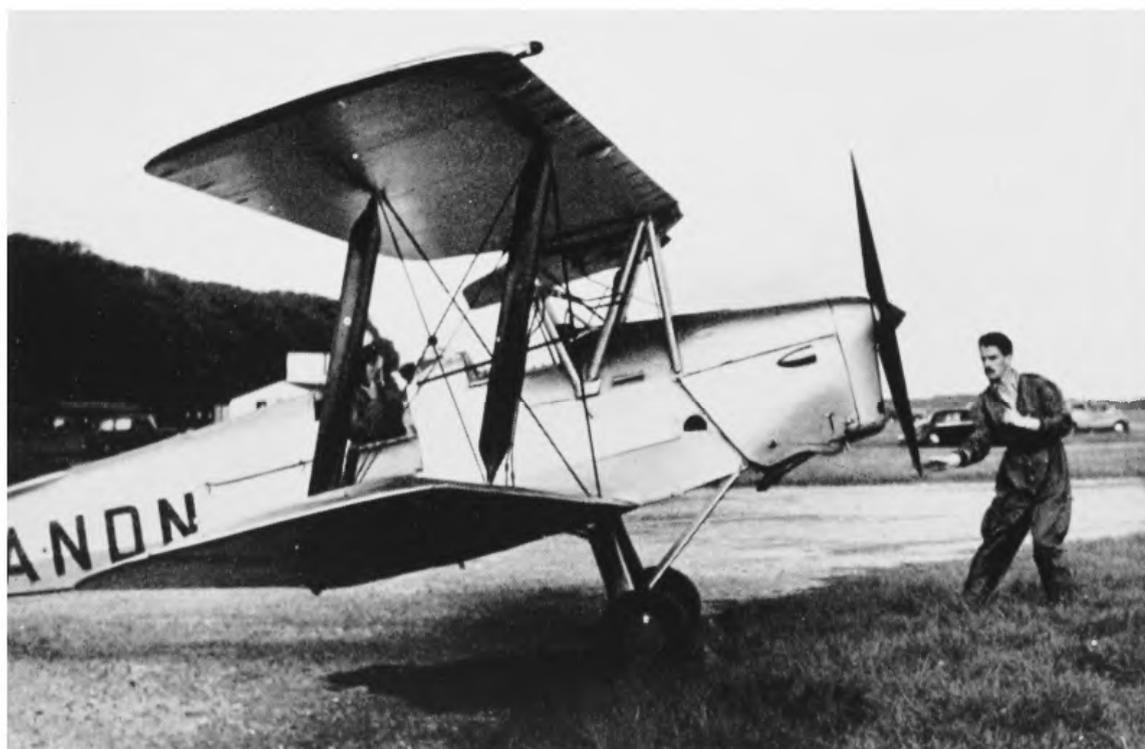
65. With the tug pilot in the cockpit, and chocks in front of the wheels, the prop is swung, and the Tiger Moth will then be taxied out to tow up the gliders waiting to fly.
