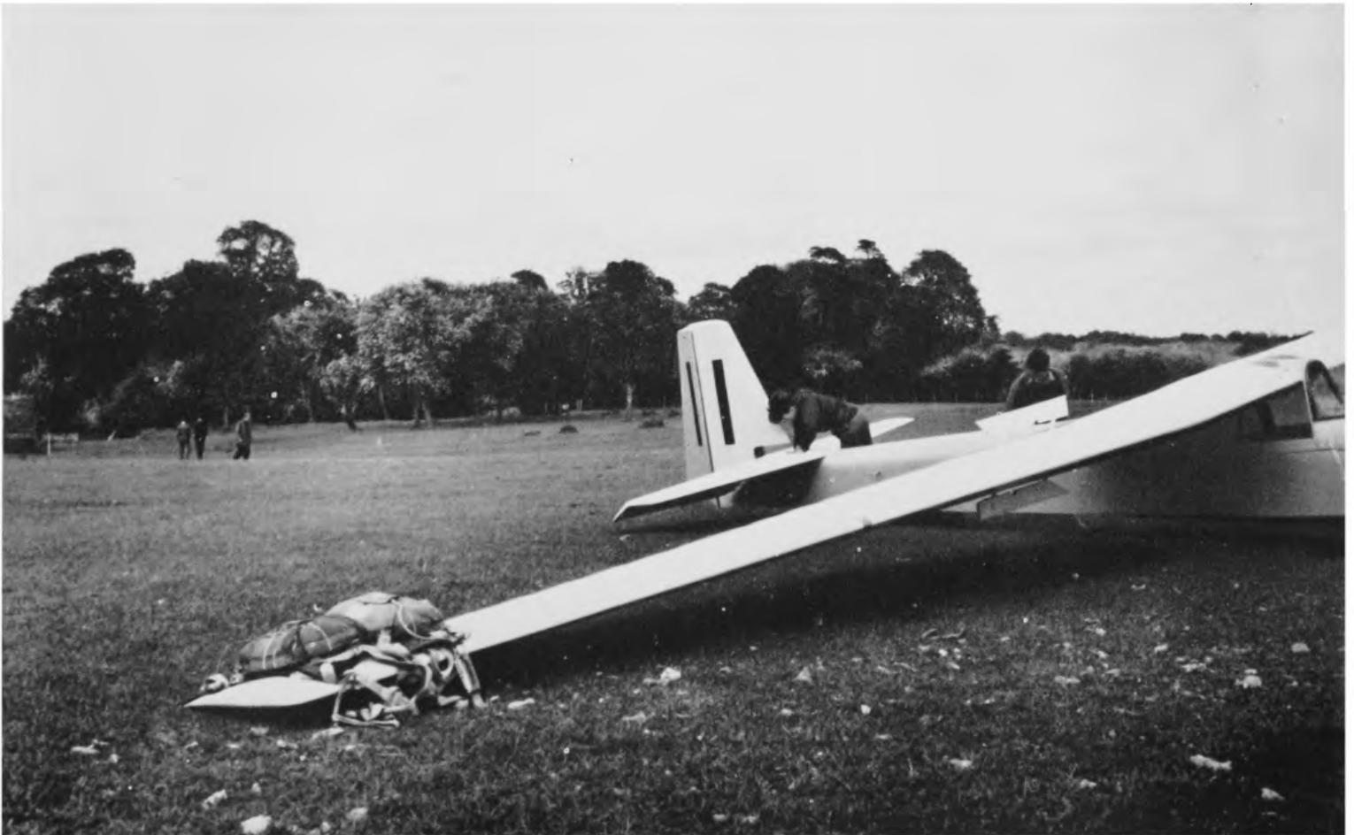
90. The first thing is to park the glider. There are no spare tyres in strange fields so the parachutes are laid carefully on the into-wind wing instead.
