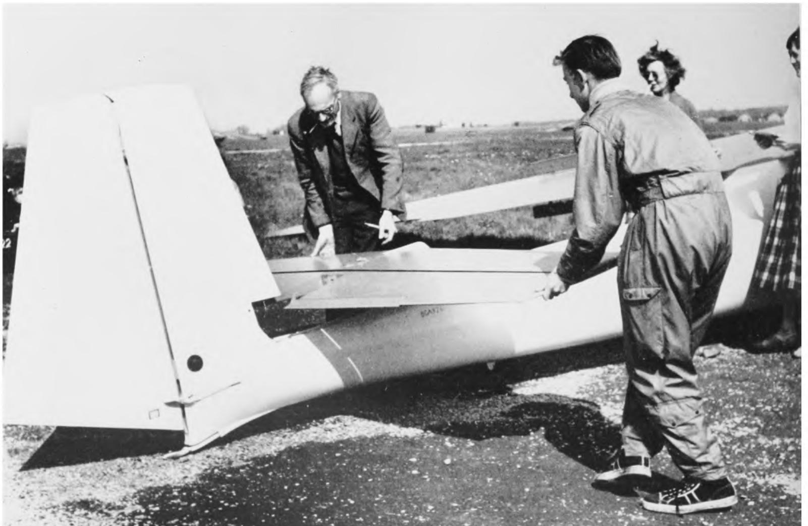
7. Now for the tailplane. Philip and Bob lower this carefully into place. They will screw down the special holding nut and then connect the elevator control. Before take-off the pilot must always check his controls, as a final safeguard against forgetfulness.
