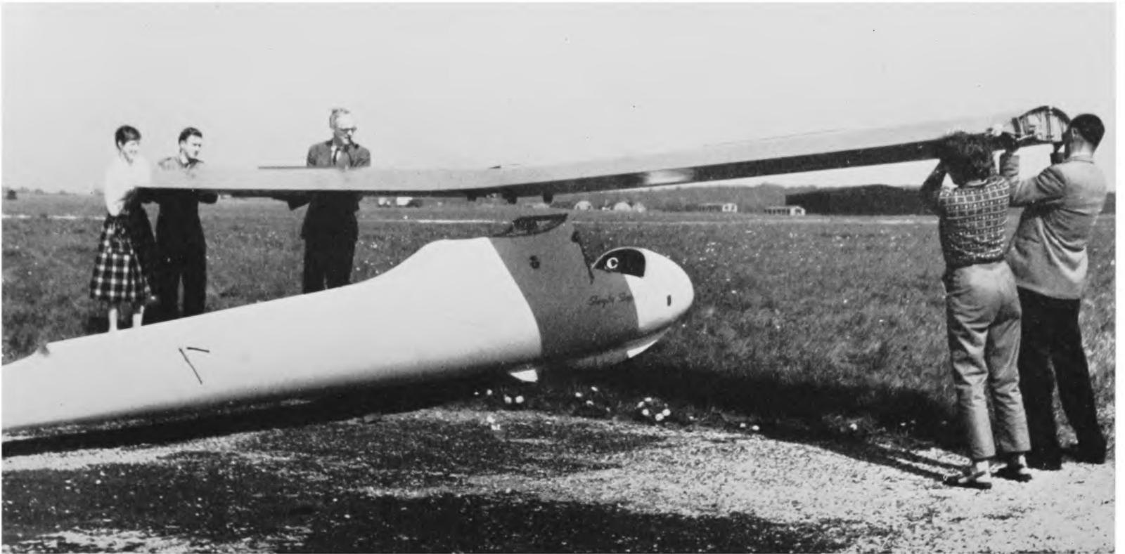
3. *The fuselage is not standing up on its own. Elizabeth (unseen) is holding it up, but is crouching down while the centre part of the wing is lowered into place. Two long pins will then be put in the fittings to fix the two together. This centre section is the heaviest part.*
