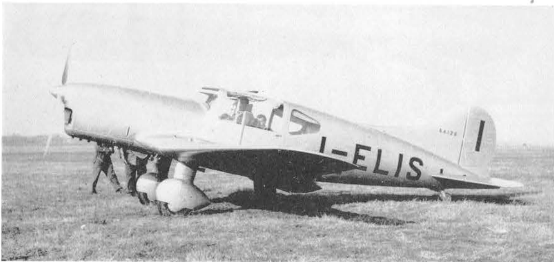
Shown here is the extended dorsal fin fitted to some examples of the S.A.I. 2 S. (I-ELIS)
