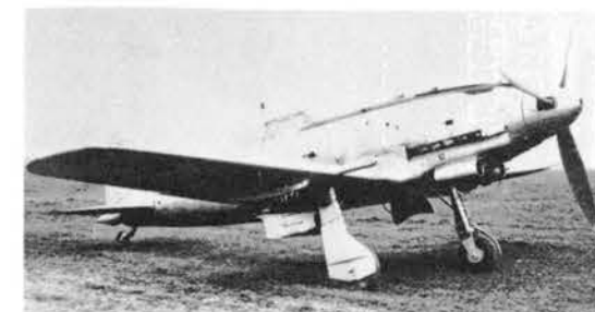
Above, the MC.205N-2, incorporating wing cannon. Below, a postwar MC.205V for Egypt. (MM 92166)
