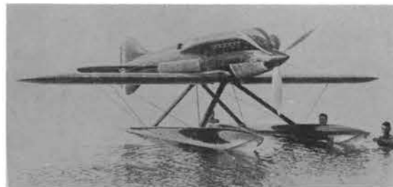
The M.67, powered by a 1400 h.p. Isotta-Fraschini W-type engine, had a maximum speed of 348 m.p.h.
