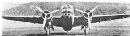
Above and below left, the P.32-II. This version had Piaggio P.XI R.C.40 radial engines in place of the Assos, plus a revised nose incorporating a gun turret above the bombardier.
