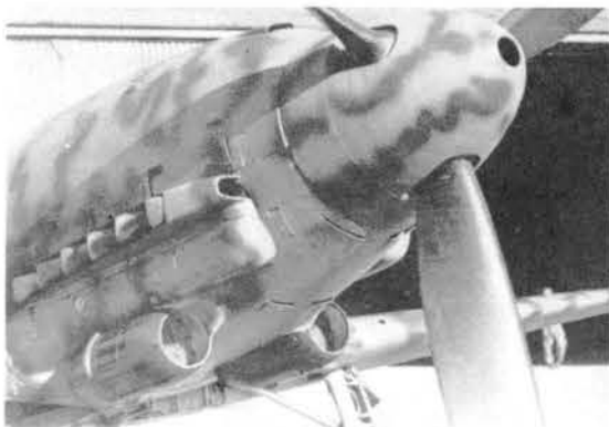
Above, an MC.205V Serie I at Guidonia in company with an MC.202, MC.200, and Ro 58. Below, a close-up showing twin oil coolers. (MM 9268)
