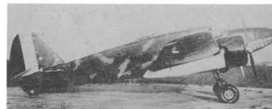
Above and right, the military version of the Ca 310 Libeccio featured extra nose transparencies and dorsal turret, plus two guns in wing roots.
