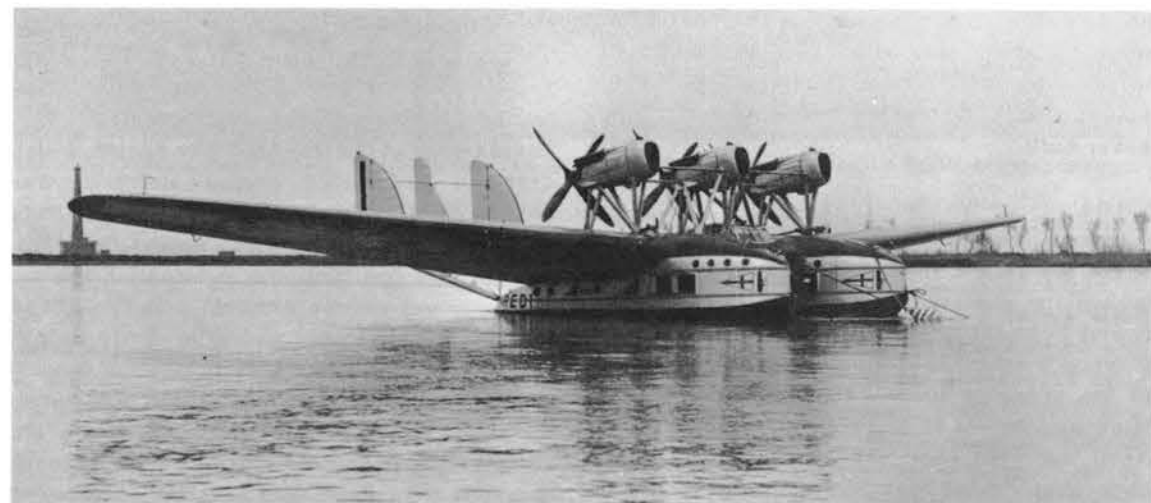
The SM.66 was a larger three-engined eighteen-passenger commercial version of the SM.55. (I-REDI)
