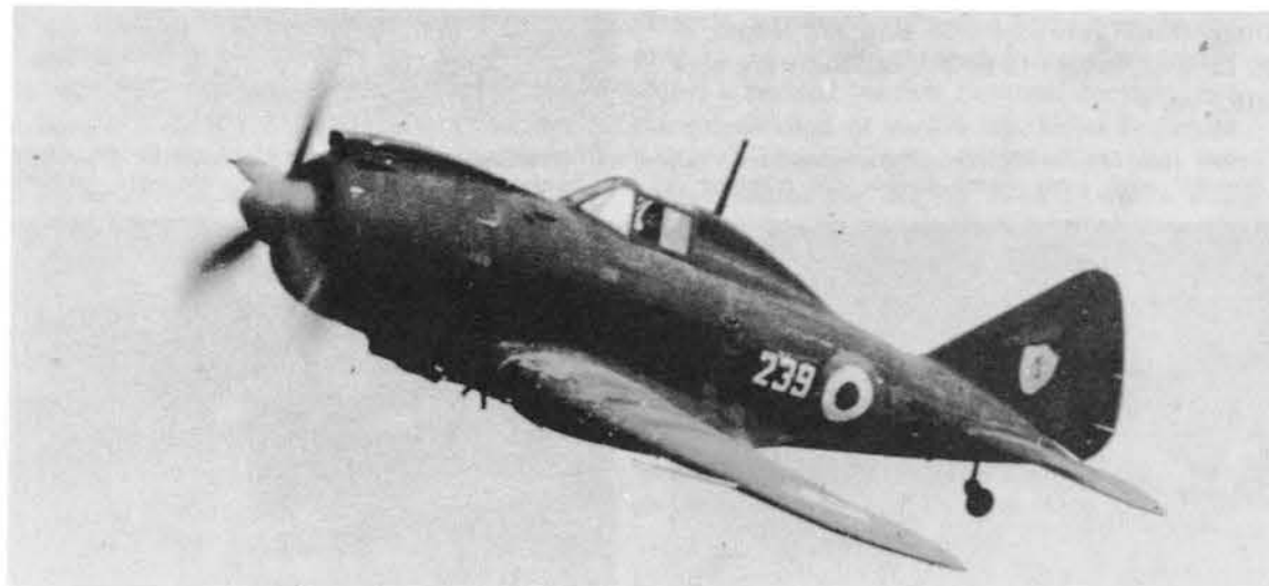
A production Re-2002 fighter-bomber with Co-Belligerent roundels. Note large spinner, revised cowling.
