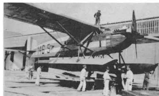
The Ca 111 was a single-engined long-range reconnaissance monoplane also developed from the Ca 101. Above, two views of the land version. Below, the Ca 111 idro, a twin-float adaptation.
