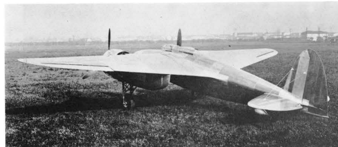
Above, the prototype Breda 88 with original tail assembly. Below, the same machine with twin fins.
