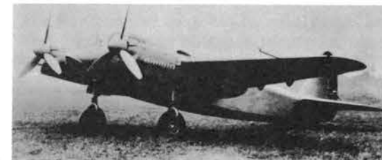
Above right and below, the SM.86 was a development of the SM.85 incorporating Isotta-Fraschini Deltas.
