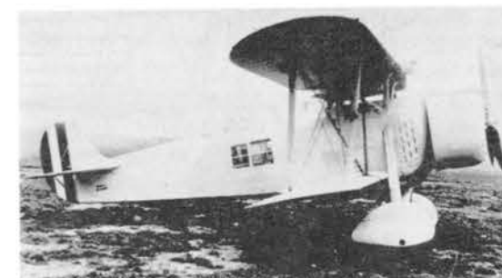
Above and below right, the Ro 37bis, which substituted a Piaggio radial engine for the FIAT unit.
