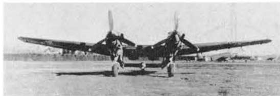
The SM.92 layout permitted a substantial reduction in drag and weight. The same basic formula was used later by the P-52 Twin Mustang.
