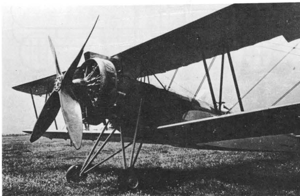
The Ca 161bis. Note the special four-bladed airscrew and long, high-aspect-ratio wings.
