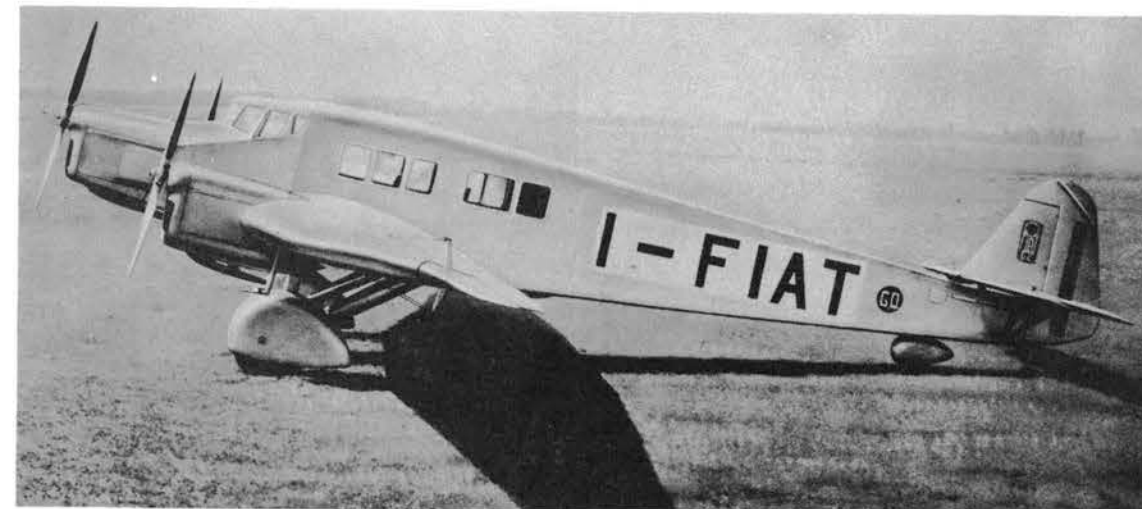
The G.2/4, with D.H. Gipsy-Queen III engines. The 1-FIAT registration was 'applied' via the negative.
