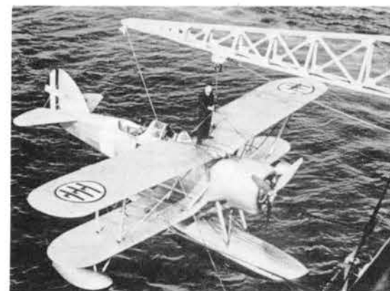
An Ro 43 reconnaissance floatplane being hoisted aboard an Italian cruiser.
