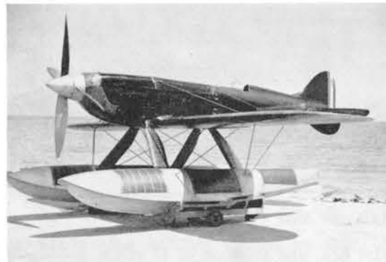
The MC.72 employed the 3100 h.p. twenty-four cylinder AS.6 engine and contra-rotating airscrews.
