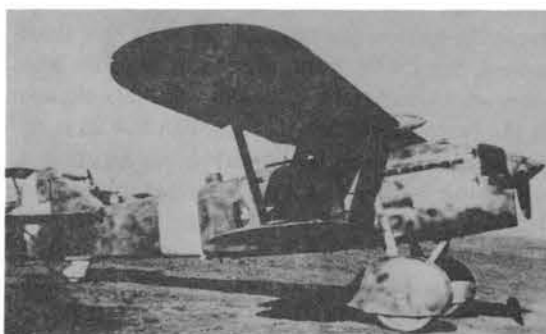
Above, two views of a CR.32ter fighter. The CR.32quater, below, was the lightest production version.
