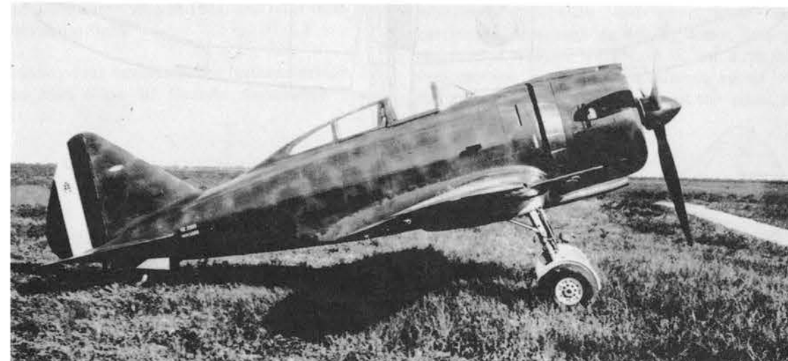
Above right, a Serie I Falco I with Hungarian insignia. Below, a similar Italian machine; in spite of the markings, this version was not ordered into production for the Regia Aeronautica. (MM 5066)
