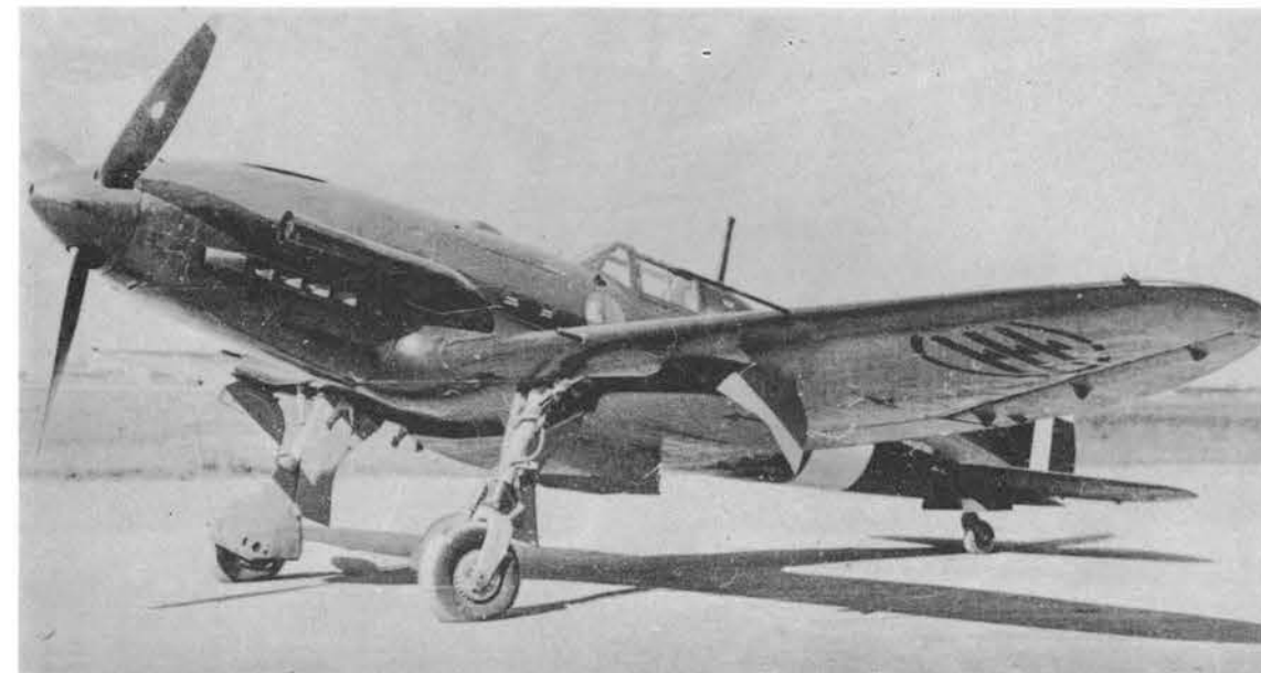
The first prototype Re 2005 Sagittario. Outward-retracting main gear was a characteristic. (MM 494)
