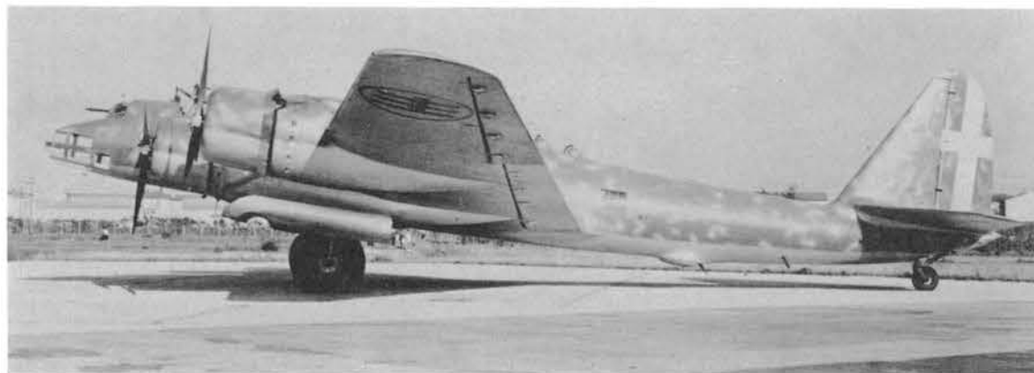
Sighting domes for the P.108B's remote-controlled nacelle turrets can be seen here atop the fuselage.
