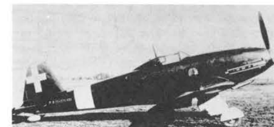
Above right and below, the F.6M, powered by a 1475 h.p. DB 605A liquid-cooled engine. (MM 481)
