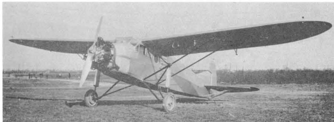
A development of the Ca 101, the Ca 105 had single engine, fixed-pitch metal airscrew, round wingtips.
