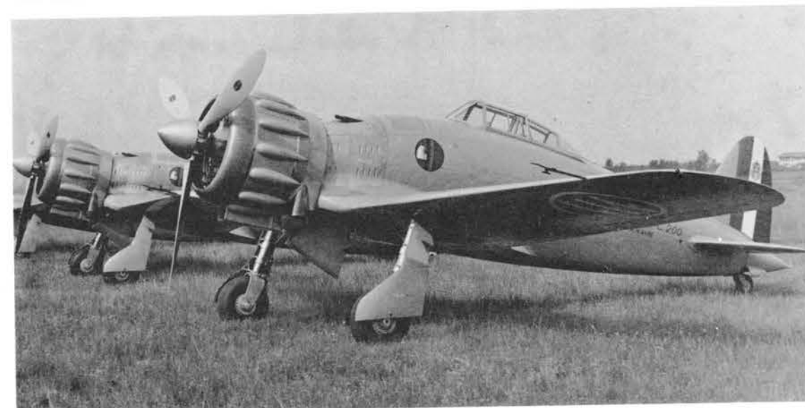
Above right, two views of early series MC.200's with enclosed sliding canopies and airscrew spinners. The same version is shown below in uncamouflaged prewar form. Note retractable tailwheel. (MM 4496)
