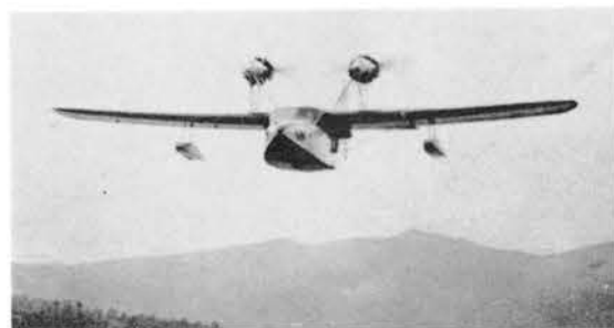
The SM.80bis employed two 75 h.p. Pobjoy radials. Power matched that of the C.N.A. version, but increased drag limited performance appreciably.
