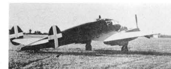
The Ca 331A was the first Bergamaschi design with all-metal stressed-skin structure.
