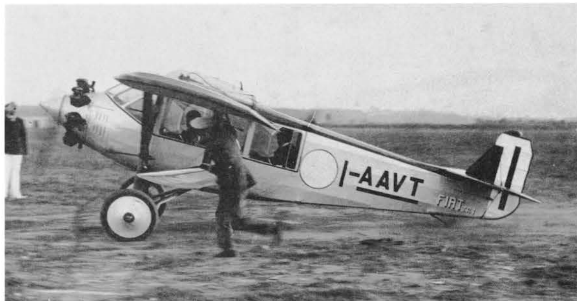
The TR.1 two-seat cabin monoplane was a contemporary of the basically similar AS.1 and AS.2 models. A seven-cylinder FIAT A.50 S radial engine provided 100 h.p. (I-AAVT)
