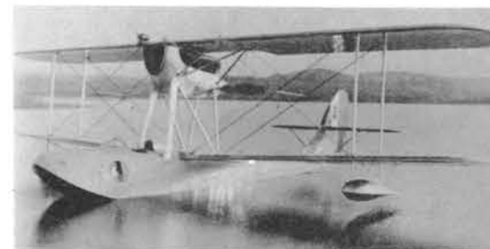
Left, the M.41 fighter flying boat. The M.71, right, differed only in the substitution of rigid bracing.
