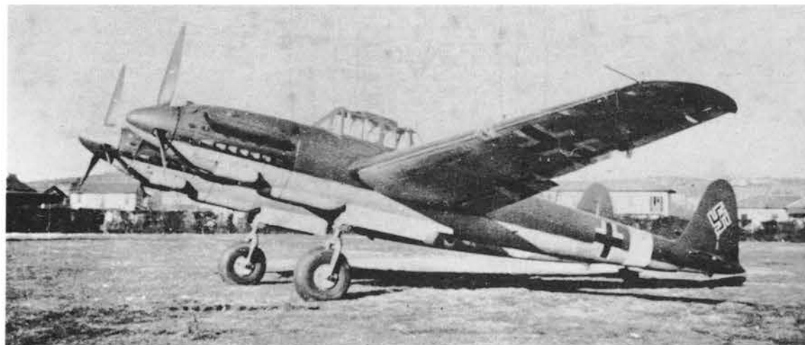
The SM.92, developed from the SM.91, placed the crew in the port boom, omitting the central nacelle.
