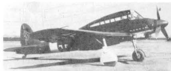
Above, two views of the SM.93 dive or torpedo bomber, which accommodated the pilot in prone position. Below the first SM.95 transport. Built as a civil airliner, it was flown in 1942 with military markings.
