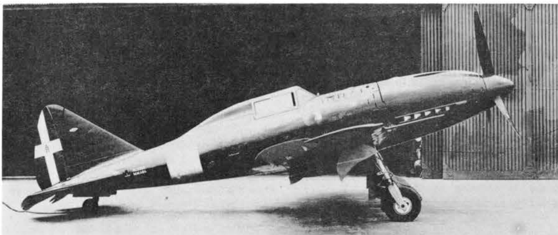
Above and below, the Re 2005 Sagittario was one of the best Italian fighters. Refined airframe and 1475 h.p. DB 605A-1 engine gave excellent performance. A few production machines began to enter service in mid-1943, too late to be effective. Some fought in Rumania and Germany. (MM 494)
