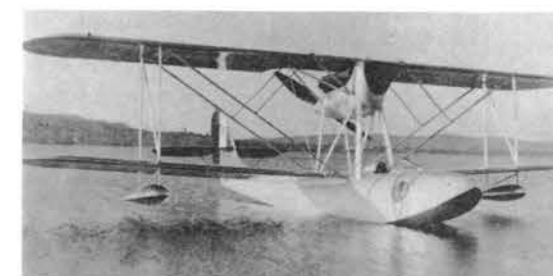
Left, the M.41 fighter flying boat. The M.71, right, differed only in the substitution of rigid bracing.
