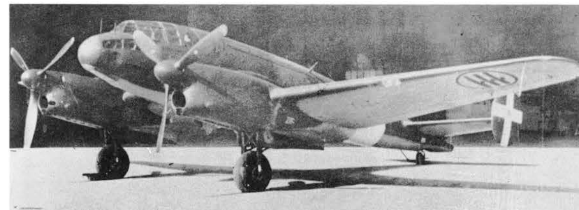
Above and below, the Ca 331B night fighter featured a revised nose with up to six 20-mm. cannon.
