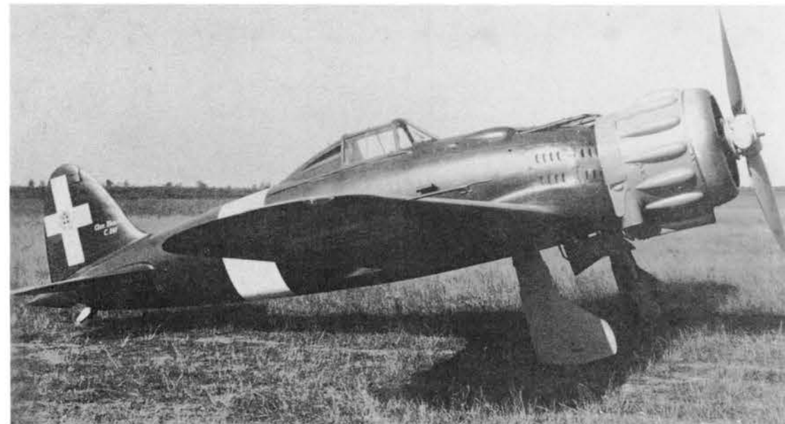
The MC.201 was characterized by a sleeker fuselage, enclosed cockpit, and prominent gun fairings.
