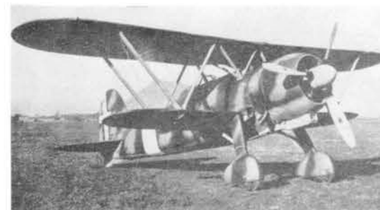
The CR.42 A.S. was an assault version for North African use. Modifications were revised air scoop and underwing fittings for two 220-lb. bombs or supplementary fuel tanks.
