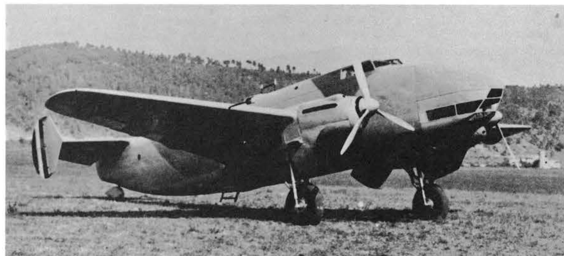
The P.32-I medium bomber appeared in 1936 with 820 h.p. Isotta-Fraschini Asso XI R.C. water-cooled engines. Visible here are the semi-retractable dorsal and ventral machine gun turrets.
