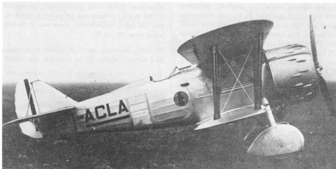
The CR.41 fitted a Gnôme-Rhône radial, three-bladed airscrew, and taller tail surfaces. (I-ACLA)
