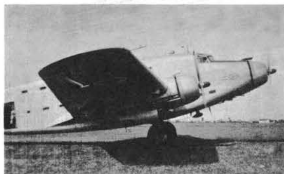
Postwar SM.82's were fitted with Pratt & Whitney radials. The Canguro was still operating twenty years after the appearance of the first prototype; it can be considered one of the most successful Italian aircraft.
