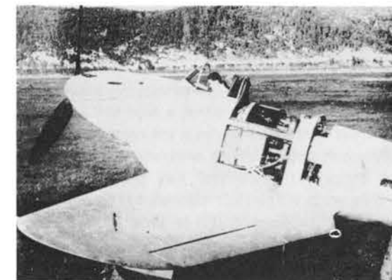
Above and below right, the P.119 had an eighteen-cylinder P.XV R.C.60/2v radial buried in the fuselage.
