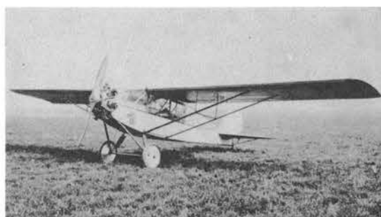
Left, a Breda 15 with constant-chord wing. Right, the improved 15 S with elliptical wing. (I-AAUJ)
