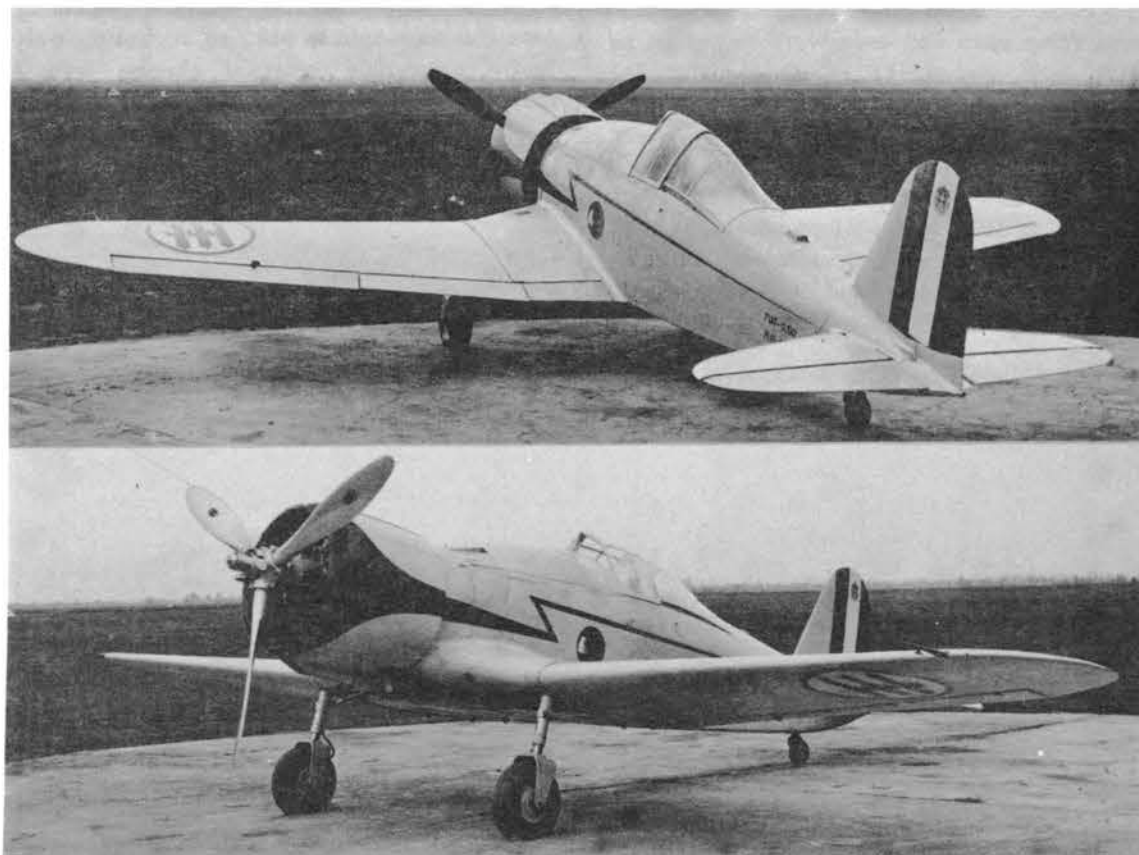
The prototype G.50, the first all-metal Italian single-seat fighter, built in 1937. (MM 334)
