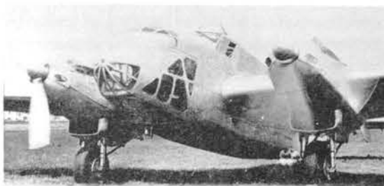
Above and below left, the Ca 135 prototype after the fitting of three-bladed metal airscrews.
