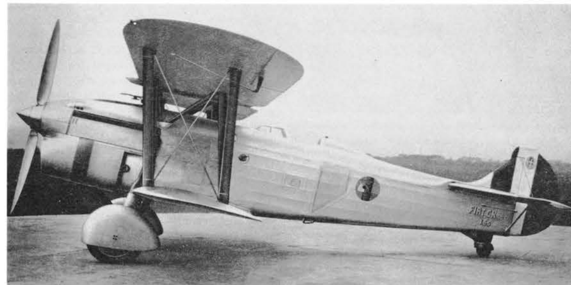
Above, the prototype CR.30, built in 1932. Below, a production model; note differences in fin shape, windscreen, and headrest. Exhaust extension was not a standard fitting.
