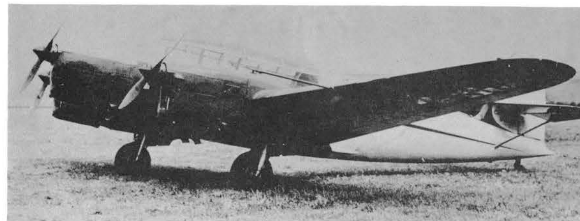
A Z.1012 fitted with four-cylinder 120 h.p. Alfa Romeo 110-I in-line engines.
