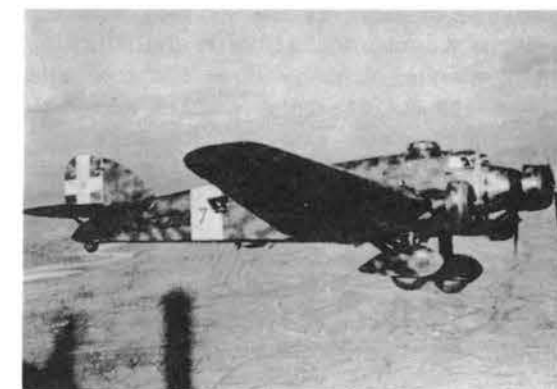
Above, the twin-engine SM.81B, with 840 h.p. Isotta-Fraschini Asso XI R.C. engines. Below right, a standard SM.81 bomber over Greece. As a night bomber, the type earned the name Pipistrello (Bat).
