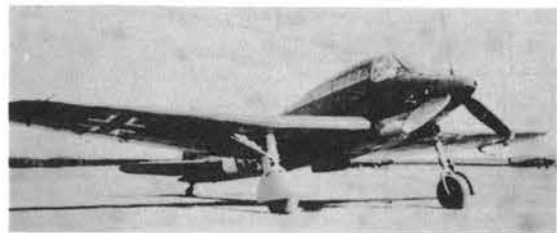
Above, two views of the SM.93 dive or torpedo bomber, which accommodated the pilot in prone position. Below the first SM.95 transport. Built as a civil airliner, it was flown in 1942 with military markings.
