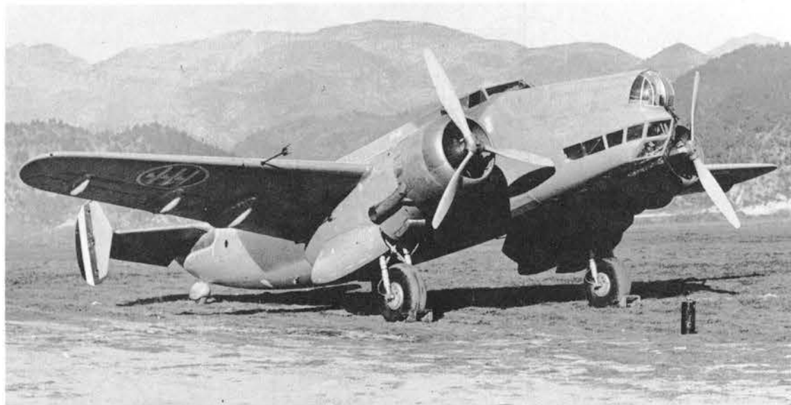
Above and below left, the P.32-II. This version had Piaggio P.XI R.C.40 radial engines in place of the Assos, plus a revised nose incorporating a gun turret above the bombardier.
