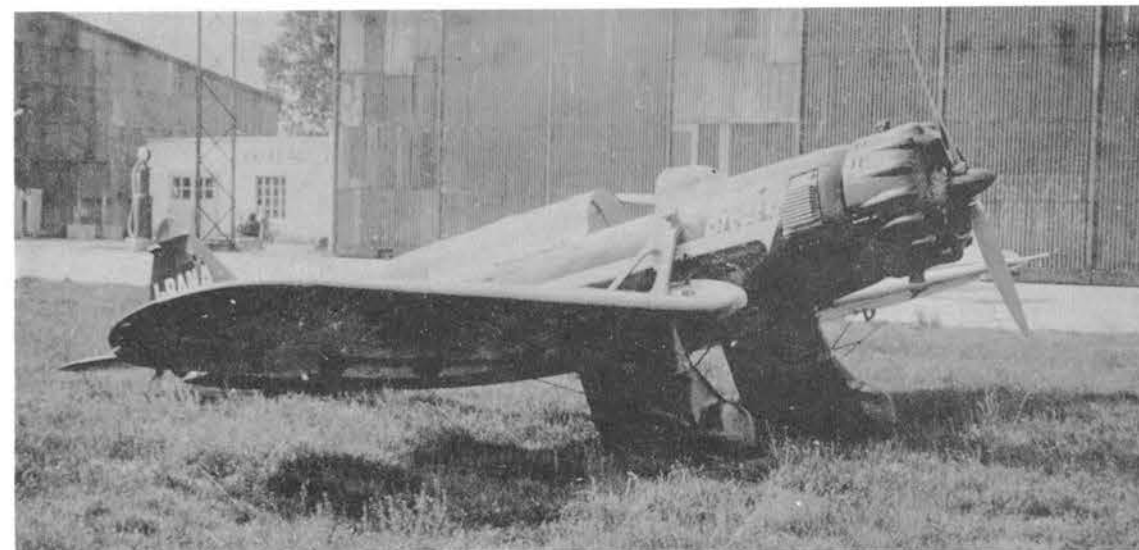
Above, a Breda 42 with postwar registration I-RANA. Below right can be seen the Breda-Mazzini wing-valve slots. This machine, I-OMBO, was photographed in Germany in 1934.
