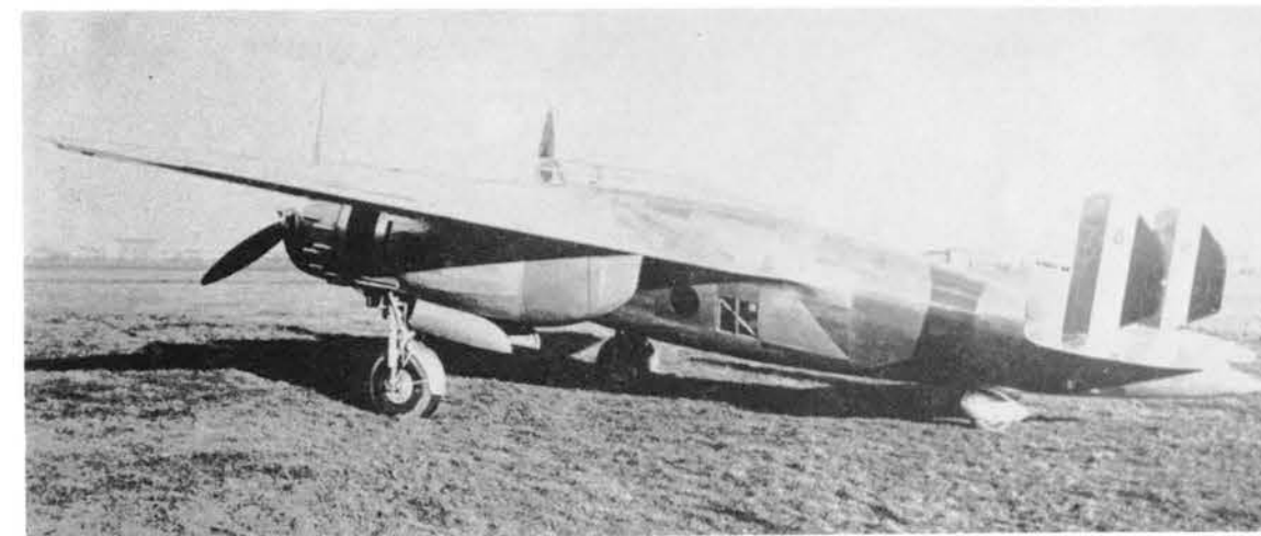
Above, the prototype Breda 88 with original tail assembly. Below, the same machine with twin fins.
