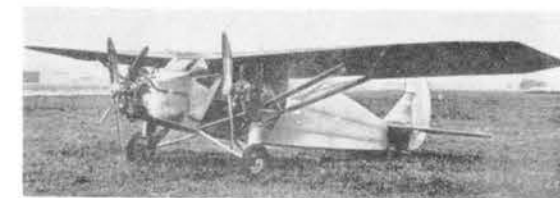
The trimotor version of the Ca 97, with 130 h.p. Lorraine-Dietrich five-cylinder radial engines.
