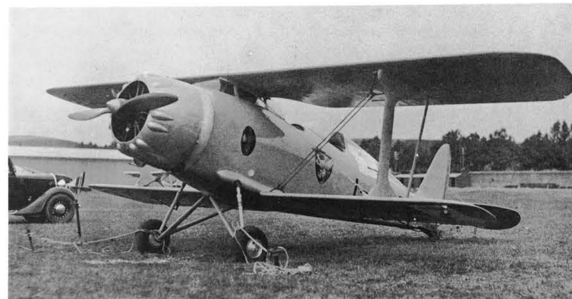
The S.A.I. 1 two-seat sport biplane; note the screen built into the wing center bracing. (I-AZIR)
