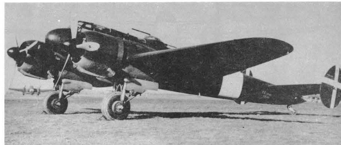
The FC.20bis ground attack machine with 37-mm. nose cannon and dorsal turret. (MM 404)
