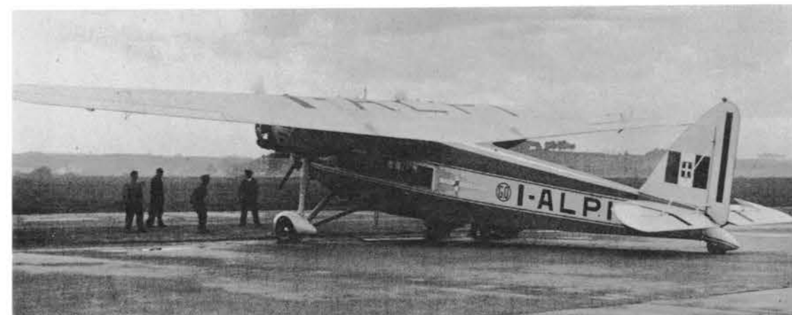
Above right and below, two SM.71 transports. Note different landing gear. (I-ROMA, I-ALPI)
