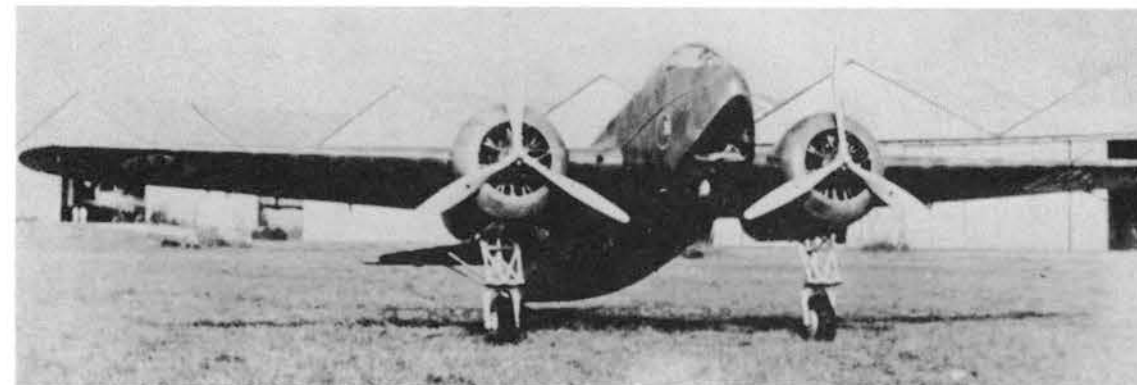
The SM.85 was powered by two 500 h.p. Piaggio P.VII R.C.35 seven-cylinder radial engines.
