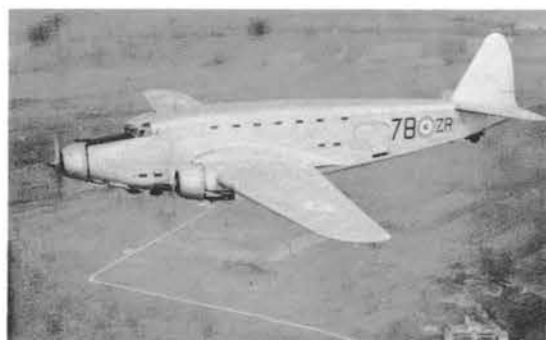
Postwar SM.82's were fitted with Pratt & Whitney radials. The Canguro was still operating twenty years after the appearance of the first prototype; it can be considered one of the most successful Italian aircraft.
