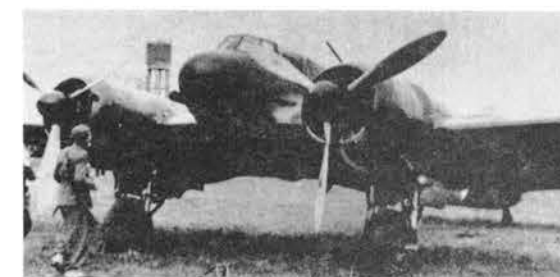
Nose cannon and wing root gun can be seen here.
