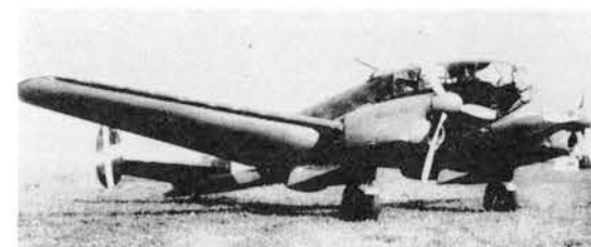
The Ca 331A was the first Bergamaschi design with all-metal stressed-skin structure.
