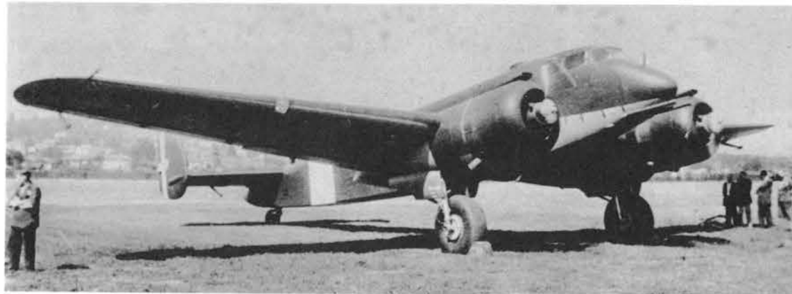
The SM.89 twin-engined attack bomber had a forward-firing armament of two cannon and two machine guns.
