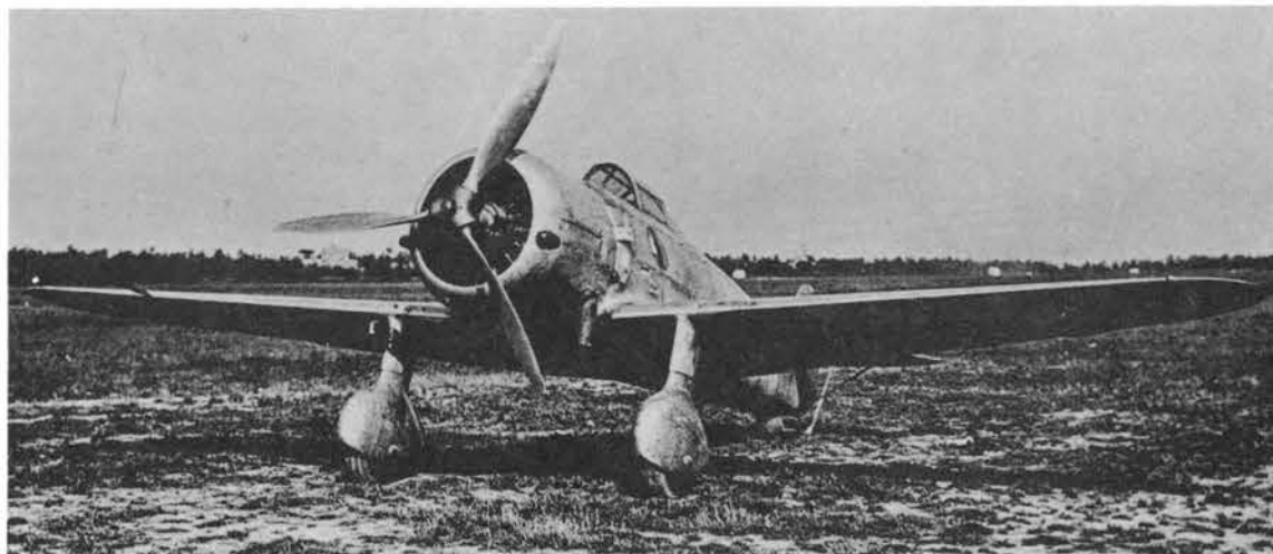
These two views show the differences between the initial Ro 51 and the second prototype, which had retractable landing gear and enlarged vertical tail surfaces.
