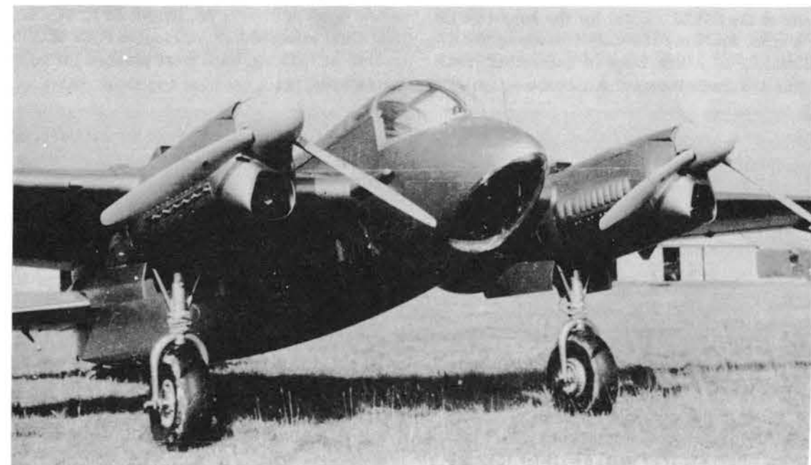
Above right and below, the SM.86 was a development of the SM.85 incorporating Isotta-Fraschini Deltas.
