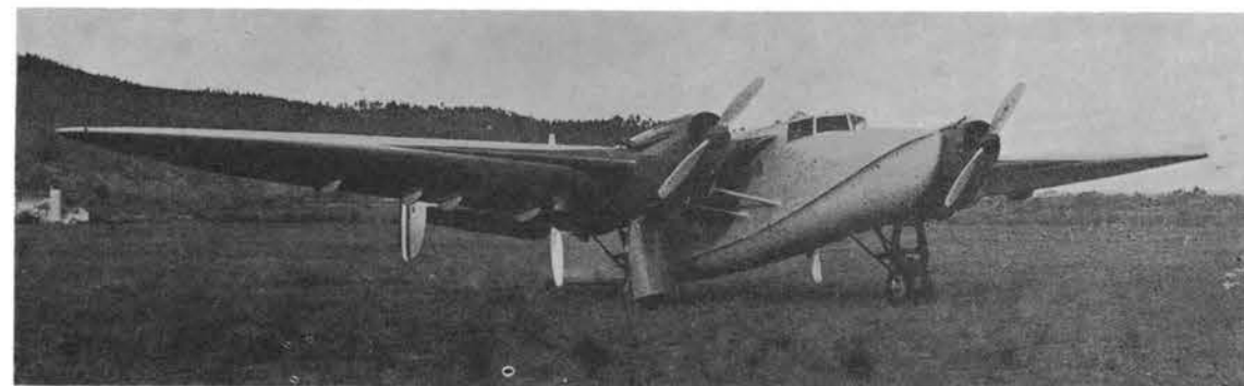
Above and below, the graceful P.23M, with fuselage "keel", tandem engines. Note missing gear fairing.
