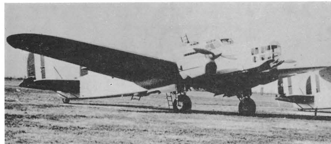
A view of the Asso-powered Z.1011, showing dorsal and ventral gun turrets.
