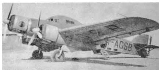
Above, the SM.79 military prototype with landing gear extended. Production SM.79-I's differed very little. Below, the personal SM.79 of Italo Balbo. In spite of I-AGSB registration, machine sported camouflage.
