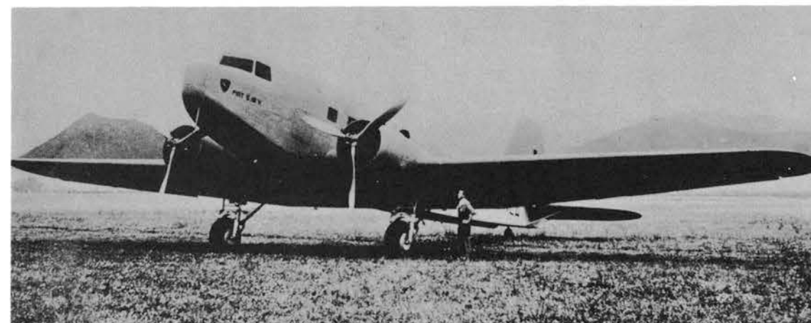
Above right, the first G.18. Below, Avio Linee Italiane G.18V with FIAT A.80 R.C.41 radials. (I-ENEA)
