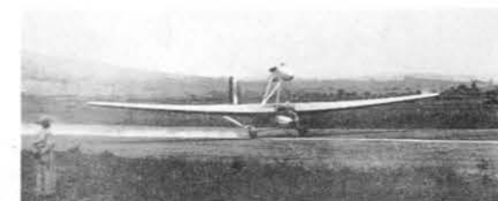
A specially prepared 4265-ft. cement track was required for the SM.64's record flights. The SM.64 weighed 15,430 lb. loaded, lifted off at 93 m.p.h.
