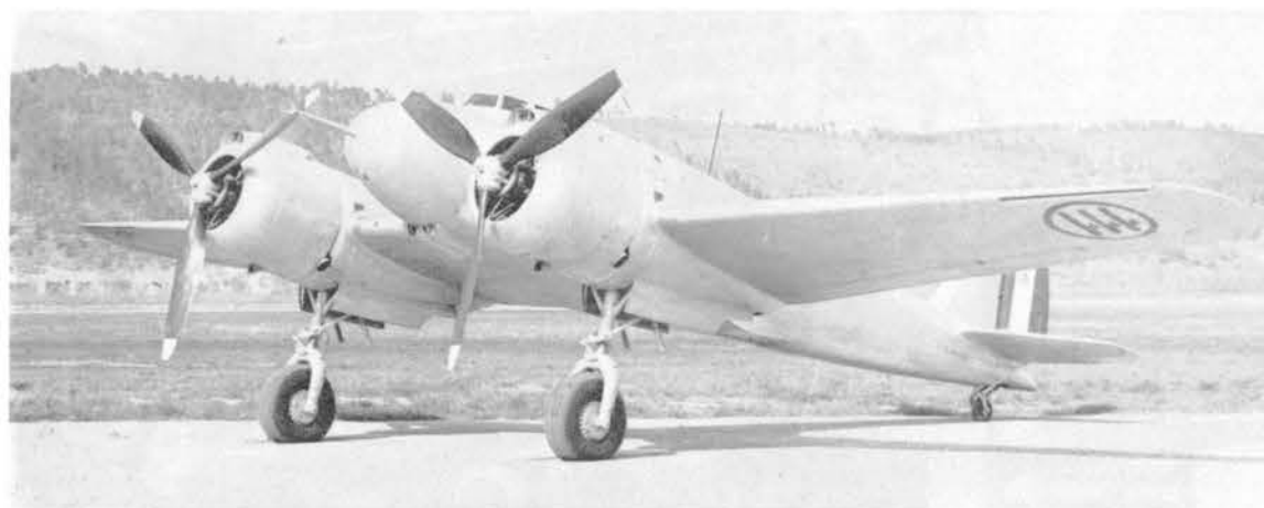
The P.111 was a high-altitude research plane built to test cabin pressurization techniques. (MM 465).
