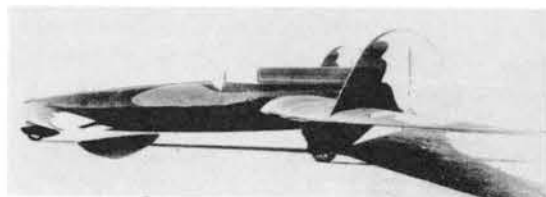
The SS.2 single-seat and SS.3 two-seat tail-first lightplanes were forerunners of the SS.4 canard fighter.
