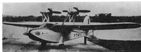
The SM.80bis employed two 75 h.p. Pobjoy radials. Power matched that of the C.N.A. version, but increased drag limited performance appreciably.
