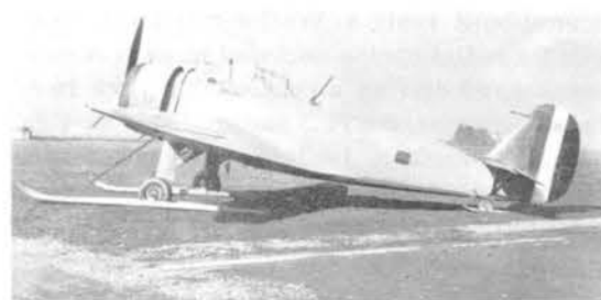
Left, a line-up of AP.1 reconnaissance aircraft. Above, a ski-equipped model. Below, a standard reconnaissance AP.1. Note mirror, gun barrel clip.
