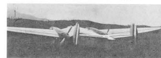
Above and below, the graceful P.23M, with fuselage "keel", tandem engines. Note missing gear fairing.
