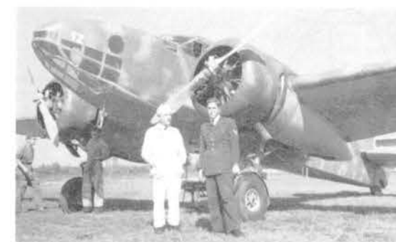
Above and right, the military version of the Ca 310 Libeccio featured extra nose transparencies and dorsal turret, plus two guns in wing roots.
