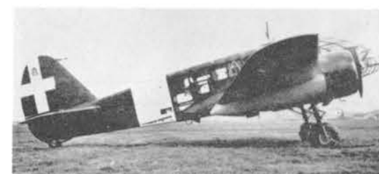
Above left, the Ca 310bis, prototype for the Ca 311. Above right, a Ca 311 reconnaissance bomber. Below, the Ca 311M, similar except for the adoption of a stepped windscreen.
