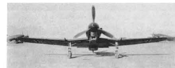
The G.56 prototype with DB 603A engine was the fastest Italian fighter, achieving 425 m.p.h.
