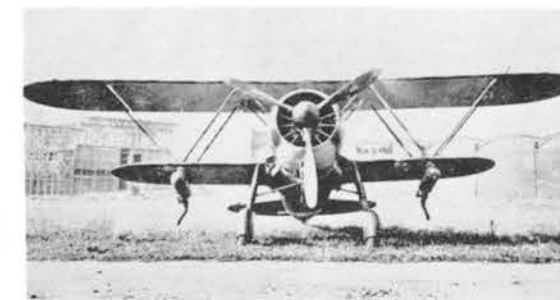
The CR.42 A.S. was an assault version for North African use. Modifications were revised air scoop and underwing fittings for two 220-lb. bombs or supplementary fuel tanks.
