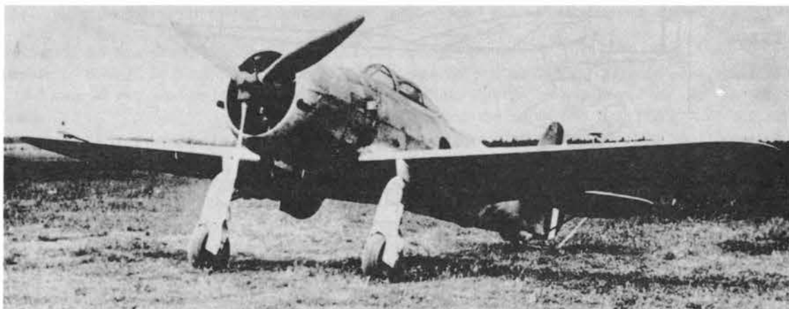
These two views show the differences between the initial Ro 51 and the second prototype, which had retractable landing gear and enlarged vertical tail surfaces.
