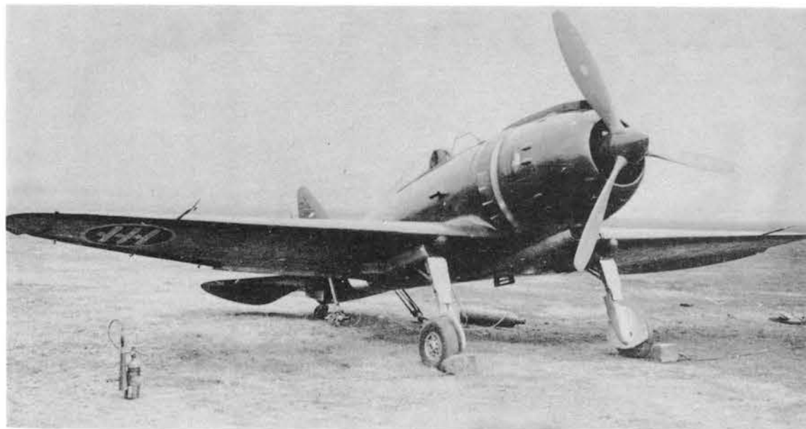
An early Re 2002 Ariete with small-diameter tapered engine cowling and small spinner.
