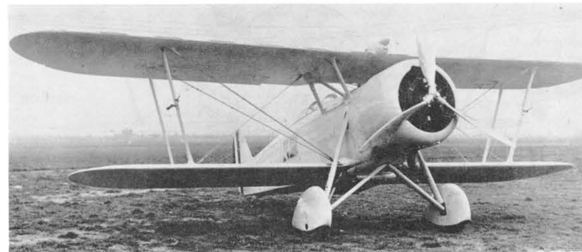
Above and below right, the Ro 37bis, which substituted a Piaggio radial engine for the FIAT unit.
