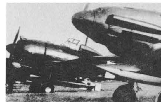
Below left, the Re 2001bis, an experimental version with leading-edge radiators. Right, an Re 2001 (foreground) with glide bomb below the fuselage. In the background is an Re 2002 Ariete with torpedo.
