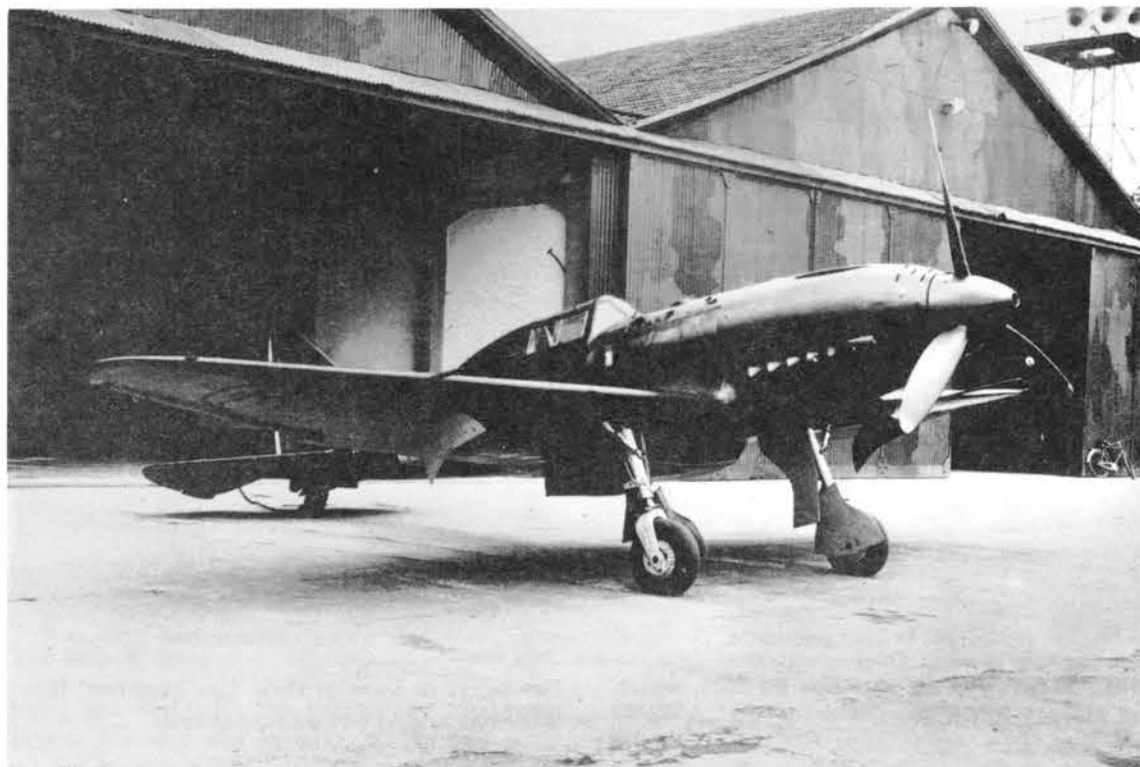
Above and below, the Re 2005 Sagittario was one of the best Italian fighters. Refined airframe and 1475 h.p. DB 605A-1 engine gave excellent performance. A few production machines began to enter service in mid-1943, too late to be effective. Some fought in Rumania and Germany. (MM 494)
