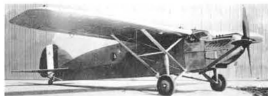
The Ca 111 was a single-engined long-range reconnaissance monoplane also developed from the Ca 101. Above, two views of the land version. Below, the Ca 111 idro, a twin-float adaptation.
