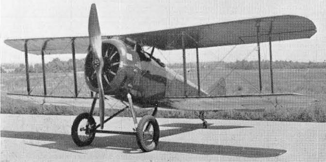
1 to 4. Standard E-1 44556 with horn-balanced rudder. The spinner of the earlier models has been abandoned. 5. E-1 of the type with plain fin and rudder, rebuilt by Wesley Tallent of N. Carolina, and currently flown at U.S.A.F. displays by Major K. S. Brown, U.S.A.F.
