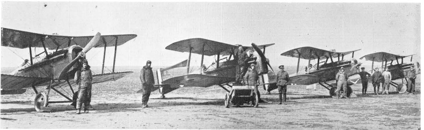
*A line-up of S.E.5a aircraft of No. 2 Squadron, Australian Flying Corps in France 1918. The 'Boomerang' marking (seen on the fuselage of the far right aircraft) was used also by No. 4 Squadron, A.F.C. on their Sopwith Camels.*
