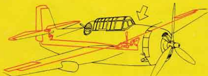
Movable controls from stick in cockpit.
