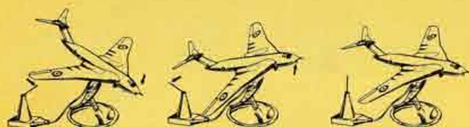
STICK CONTROLS ATTITUDE OF PLANE
