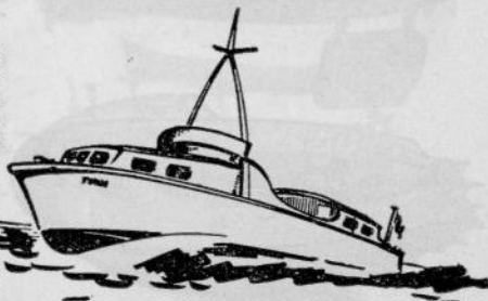
SPURTSTER By Vic Smeed Unusual 27 in. model designed round the Taplin Baker Hydrojet unit with 1½-5 c.c. engines. Simple all-ply construction, excellent performance with this novel form of propulsion. MM/695 * * 6/-
