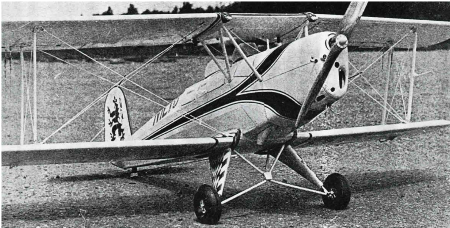
Only the rubber bands give it away as being a model. Note starting wires hanging from glowplug access hole.
