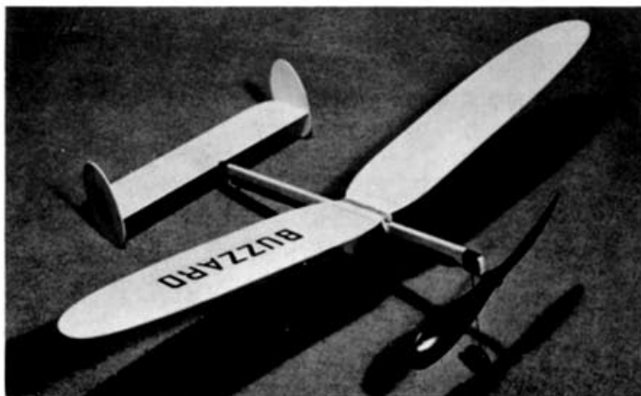
The twin-finned BUZZARD is capable of taking off under its own power from the ground. The detachable wing is held on with rubber bands.
