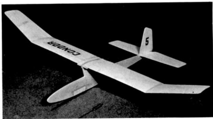
Completed CONDOR—ready for flight. Hold wing in place with rubber bands.
