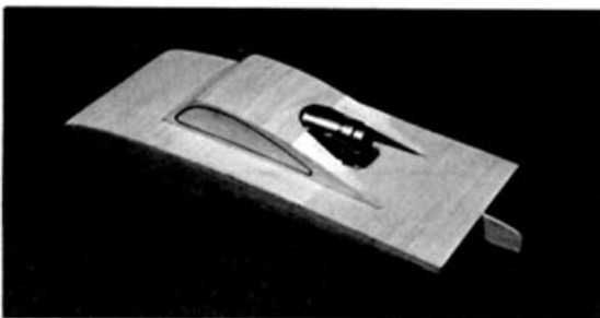
Complete model with loaded Jetex 50 motor in position.
