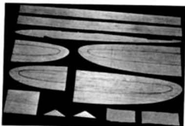
Shaped parts for SWALLOW. Note the trimming lines on flying surfaces.
