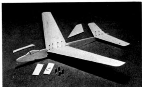
Cement flying surfaces to the fuselage, allow to dry, then replace piece of sheet over wing and add the fin.
