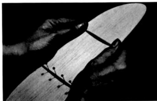
Camber outer portions of wing panels with sheet ribs.
