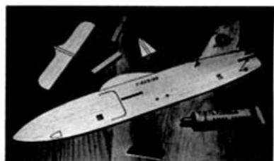
Start the construction by cementing fin to fuselage pinning down flat.
