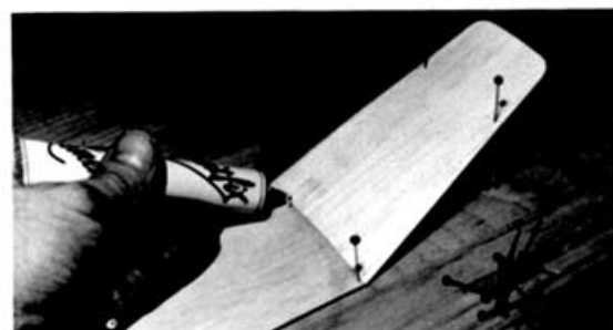
Join tip and main panels—packing up with 'Z' piece.
