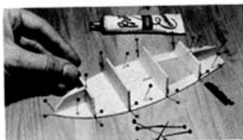
Start by pinning deck down flat and add formers (B, D, F, G)—also E and C.
