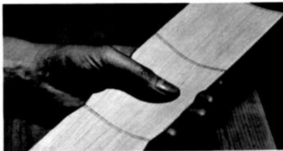
The sheet wing panels must bend easily across grain.
