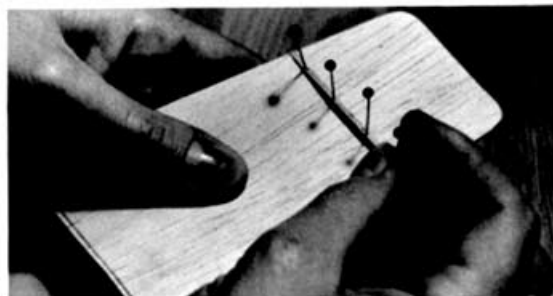
Cement 'E' ribs to the tip panels. Note use of pins.
