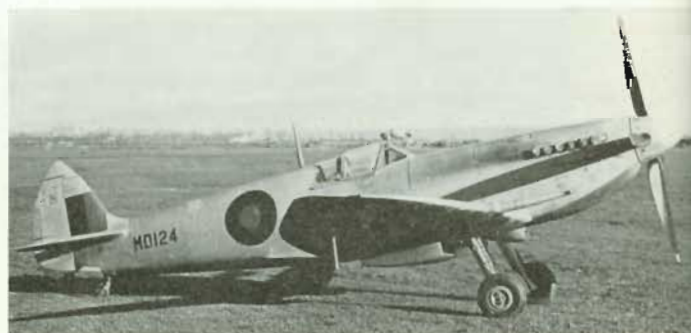
Spitfire H.F.Mk. VII in standard high altitude day fighter finish introduced 7th June, 1943. Upper surfaces Medium Sea Grey, under surfaces P.R.U. Blue. 30in. diameter Type B fuselage roundel and 24in. square fin flash.
