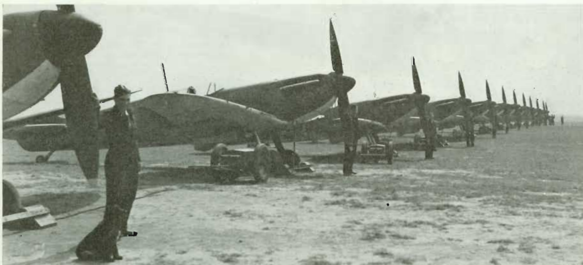
Spitfire Mk. Is of No. 19(F) Squadron. The foreground aircraft has B-scheme camouflage, the next A-scheme camouflage. Both have White undersides to the port ailerons. The painted-out Yellow ring on the fuselage, and serial number, can be clearly seen. Photo below shows Black ailerons on White wing.
