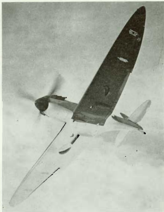
Factory finish from Feb. to May 1940. Night, White and Aluminium under surfaces. 35in. Type A fuselage roundel.
