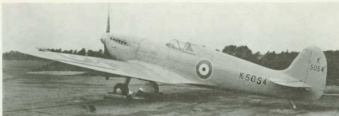
The Spitfire prototype in overall finish of Seaplane Grey. Fuselage roundels are 25in. in diameter outlined in white. Non-outlined upper wing roundels are 50in. dia. The white outlined serials are 8in. and 6in. high respectively.
