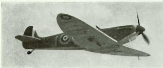
(Above and below) Spitfires of No. 19(F) Squadron. Both aircraft have Dark Green and Dark Earth upper surfaces and Sky under surfaces. The aircraft above has 25in. diameter under wing roundels, while the one below has 40in. roundels. Both aircraft have 7in. wide fin stripes.
