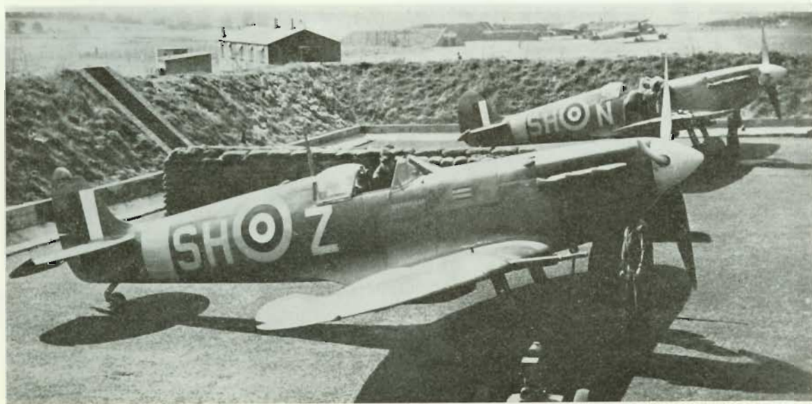
Spitfire VBs of No. 64(F) Squadron. Aircraft in foreground is 'Atchasmickar', a presentation machine. It carries the Squadron Leader's pennant. Note the 7in. Red centre spot of the 35in. roundel. Fin stripes are the standard 27in. x 24in. The camouflage scheme is probably Mixed Grey (Medium Sea Grey and Night) and Dark Green, with Medium Sea Grey under surfaces.
