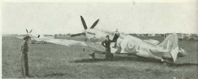
Spitfire Mk. XIV of No. 402 Squadron, 2nd Tactical Air Force. The Sky spinner has been repainted 'black' and the Sky 18in. fuselage band over painted in the standard camouflage colours. Type C upper wing roundel outlined in Yellow used during the final phases of war.
