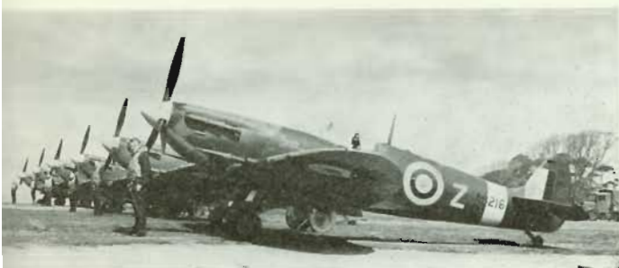
Spitfire VBs of No. 91(F) Squadron. Spitfire in the foreground is AB216, the Squadron Commander's aircraft. Upper surface colours are Dark Green and (probably) Ocean Grey.
