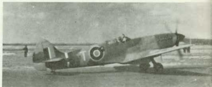
Spitfire F.R. Mk. XIV, RM795, in May 1945. Standard day fighter camouflage scheme. Thin White or Sky band, approximately 6in. wide, around the rear fuselage. Black spinner. (Photos: R.C. Jones).
