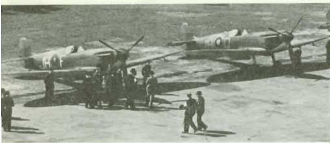
Spitfire Mk. Is of No. 74(F) Squadron at Northolt in May 1939. The port wings have been painted in Night, but the starboard wings are still in the original delivery scheme of Aluminium.
