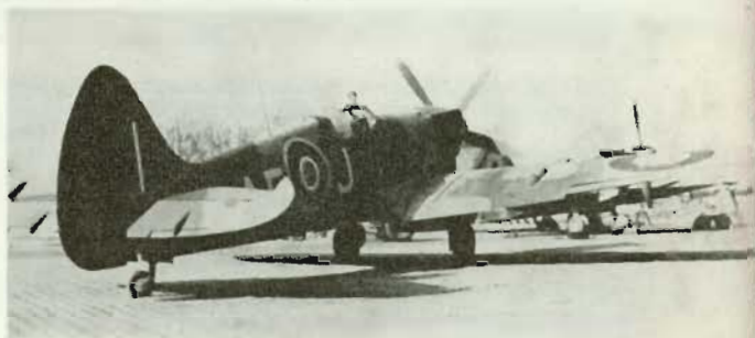
Spitfire Mk. XIV of No. 41(F) Squadron, on the Continent. Black spinner, Sky fuselage band overpainted in normal camouflage colours. Type C upper wing roundel of 56in. diameter introduced on production Spitfires after 9th March, 1945.
