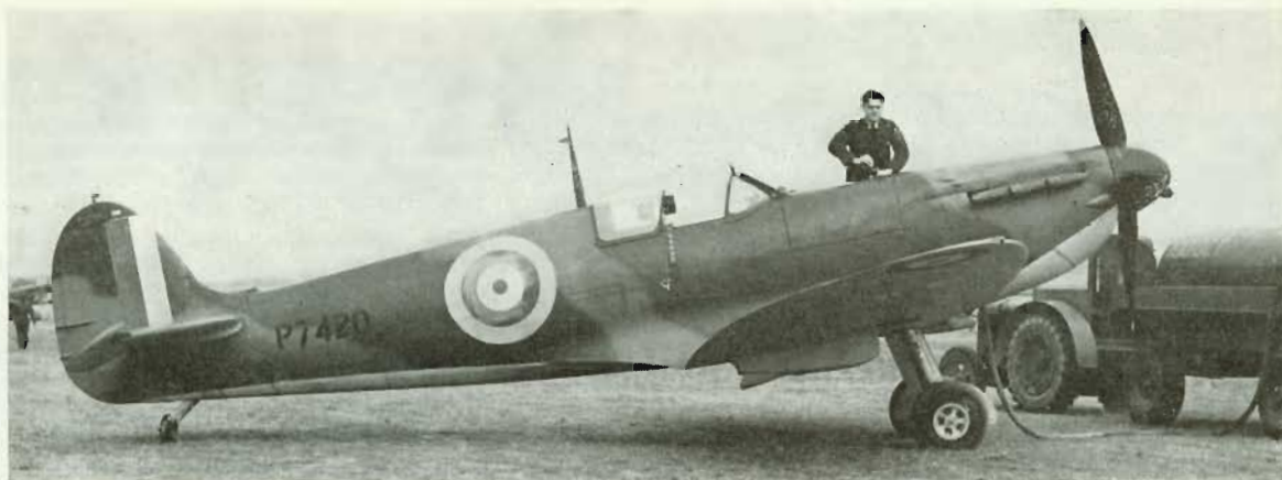
Spitfire IIA, P7420. Dark Green and Dark Earth upper surfaces, Sky under surfaces, 7in. wide bands on fin flash, 35in. Type A.I fuselage roundels, with correct proportion Red centre spot. 25in. under wing roundel near tip.
