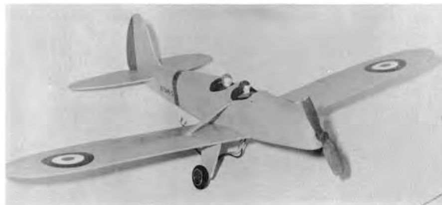
Modified Ryan PT 20 Trainer from a Frogflite kit. Prop is epoxied to shaft.
