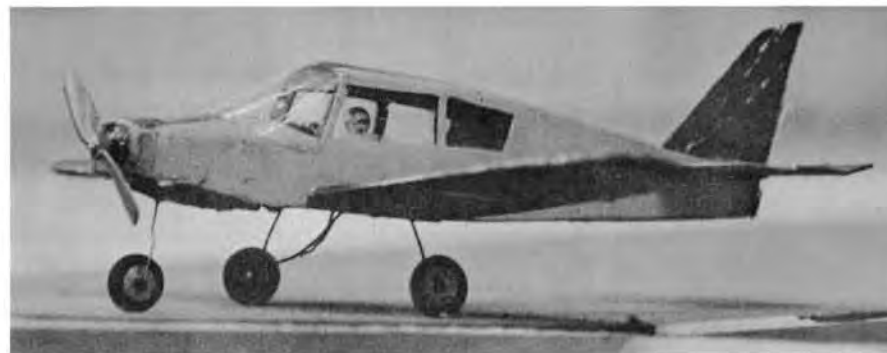
Frogflite Beagle Pup has tricycle landing gear which is an advantage for take-off and landing, also helps balance with the weight of one wheel forward.
