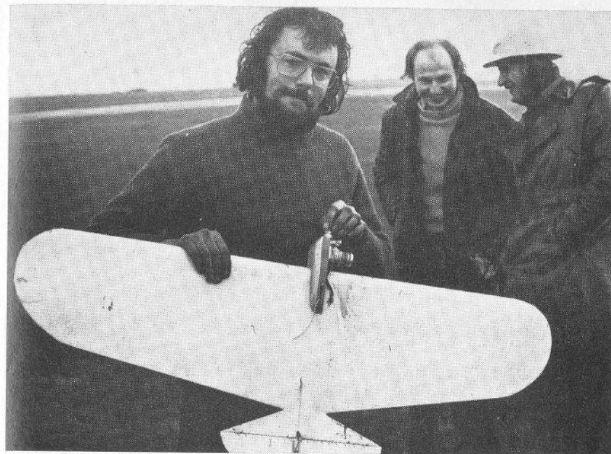
Returning to the combat scene after a number of years absence, Richard Wilkins set the 1975 scene alight with his outstanding flying ability, married to his very fast Super Tigre G15 glow powered, large area design which features polystyrene foam wing tips and leading edge sections for lightness. Motor runs on a pressurised fuel supply—using a metal tank, not a "pacifier".
