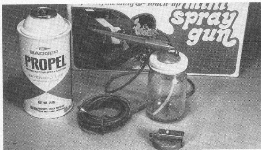
The simplest form of "air-brush", the Badger 250 Mini Spray Gun which is a spray atomizer operating on a suction principle. There is no needle but control can be achieved by variable pressure on the spray button. Opposite: Finishing sequence diagram from "Hobbypoxy Painting Pointers".
