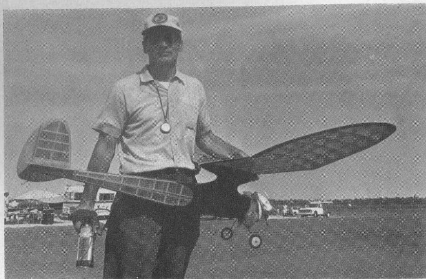
Most popular of all the subjects for R/C assist is the Cleveland Playboy Senior, a pylon design for '49 to '60 engines which performs well on wheels or floats and has relatively simple structure. It looks great when covered with bright silk.
