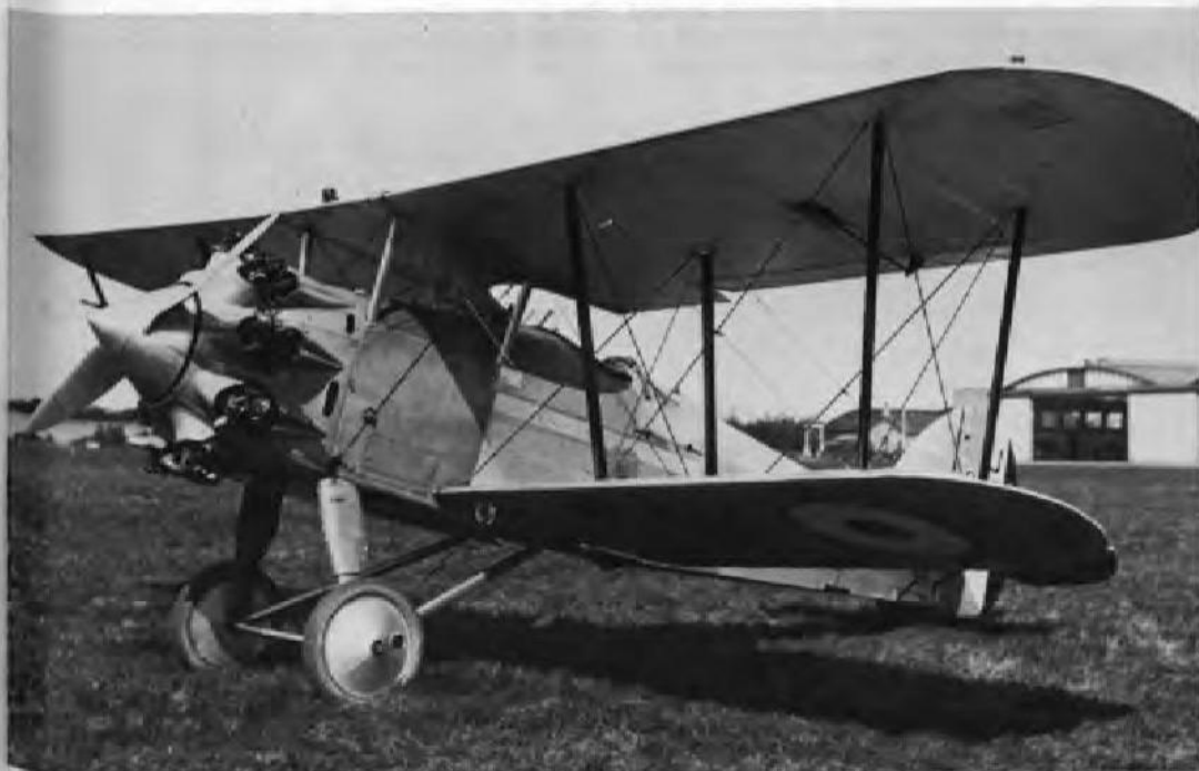
ABOVE: Letov Sm-I, the first Czechoslovak designed military aircraft demonstrates an example of a monocoque fuselage to good advantage. Note dorsal fin and well shaped gunner's cockpit (Z. Zaroslav). BELOW: Little known Hawker Hawfinch was the ancestor of the famous Fury fighter of the 1930s. Extremely clear photograph here shows a great deal of detail and is a perfect example of the more complicated built-up box. This aircraft demonstrates all the design characteristics and surface detail of the fighter aircraft of all nations during the late 1920s and mid-1930s (Hawker Siddeley).
