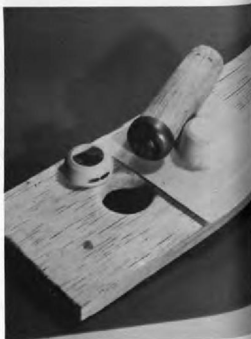
On this page can be seen (above) the actual cowl moulding process in operation, with ordinary office spring clips holding the plastic card in place over the 'female' mould. In this instance the cowl from a kit, fitted over suitable dowelling, is being used for a 'male' mould. At right can be seen the moulds, a moulding, and a completed cowl.
