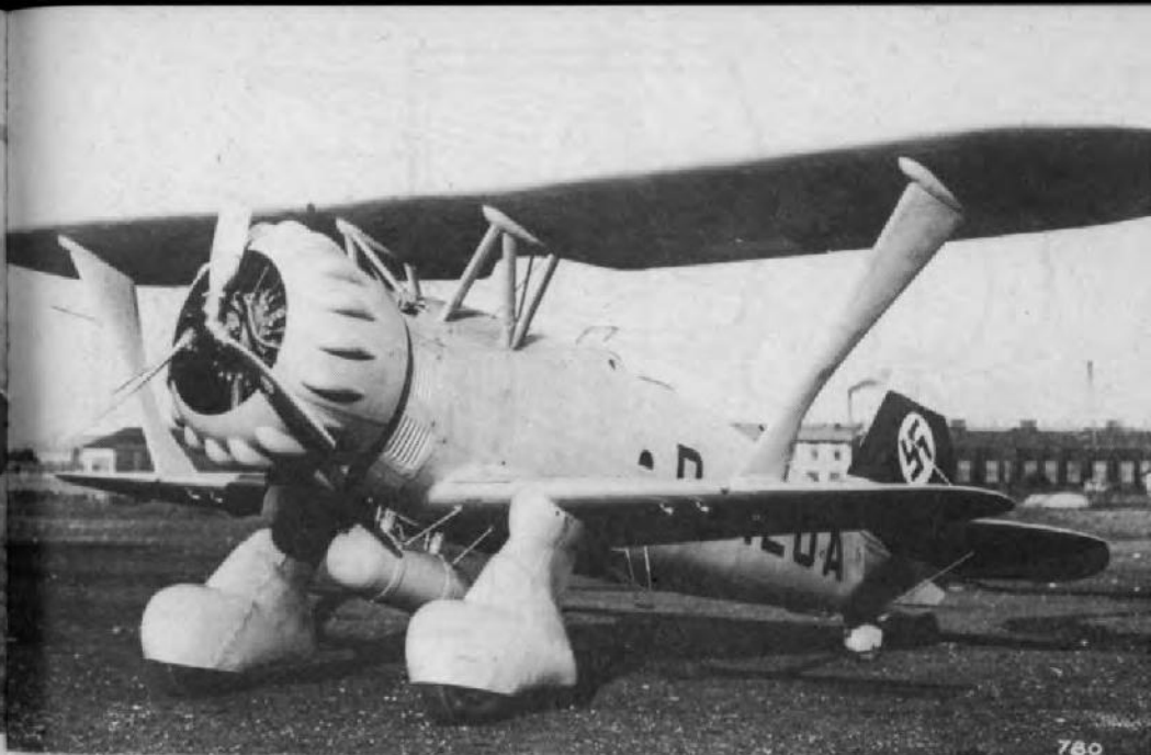
ABOVE: The prototype Henschel Hs 123 all metal construction and skinned throughout with metal except for control surfaces and parts of the wings; undoubtedly a moulded monocoque subject in model form though a kit by Airfix is available in 1:72 scale (Real Photographs).
