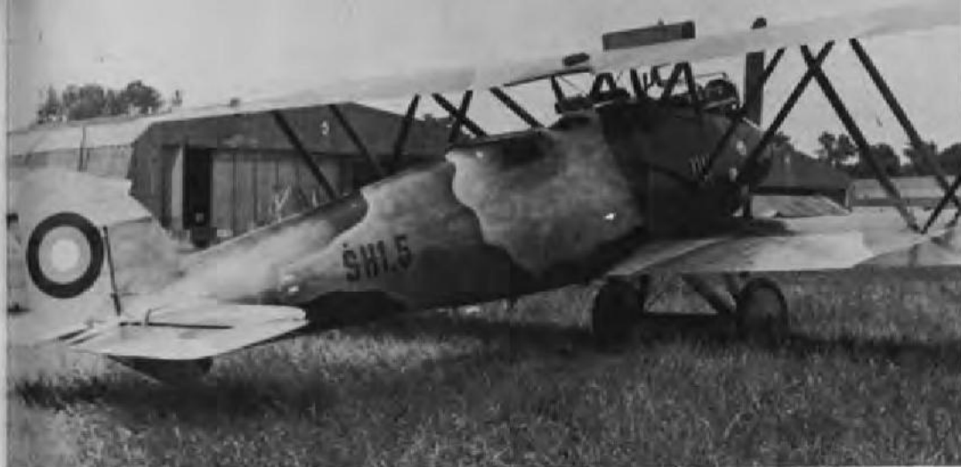
ABOVE: Letov Sm-I, the first Czechoslovak designed military aircraft demonstrates an example of a monocoque fuselage to good advantage. Note dorsal fin and well shaped gunner's cockpit (Z. Zaroslav). BELOW: Little known Hawker Hawfinch was the ancestor of the famous Fury fighter of the 1930s. Extremely clear photograph here shows a great deal of detail and is a perfect example of the more complicated built-up box. This aircraft demonstrates all the design characteristics and surface detail of the fighter aircraft of all nations during the late 1920s and mid-1930s (Hawker Siddeley).
