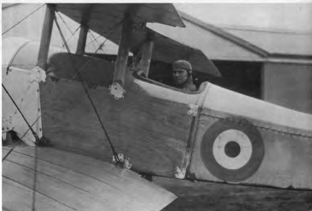
TOP: Familiar stitch lines on Bristol F2B. In this case the metal foil system can be used to great advantage, even the studs down the centre of the strips can be reproduced (IWM-Q11996). ABOVE: Martinsyde Scout shows the three basic materials of aircraft of this period, aluminium, plywood and fabric. Notice typical Martinsyde fishplates (IWM-Q65878).
