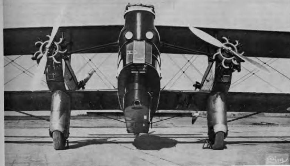
Heavily 'trousered' undercarriages were one way of achieving streamlining in the mid 30s before efficient retractable systems were evolved. Nose view of French Lioré et Olivier 206 bomber of 1936 shows these well.
