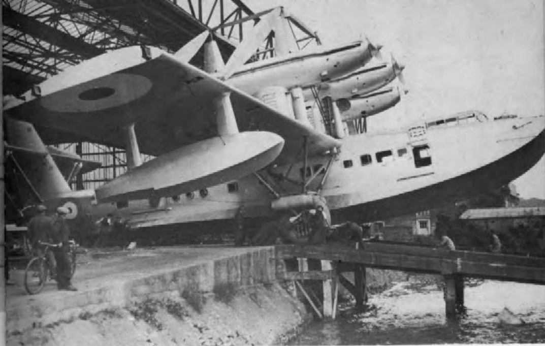
ABOVE: All metal float on Short Sarafand represents type used until virtual demise of flying boat in recent years. Note metal skinning of hull and sharp trailing edge of wing even on a very large machine such as this (Short Bros). BELOW: Modern floats fitted to a Fairey Swordfish. There is quite a large amount of surface detail on floats which should be reproduced in a 1:48 scale model such as the old Merit kit. More particularly, note the lugs, panels and sea rudder detail (MOD).
