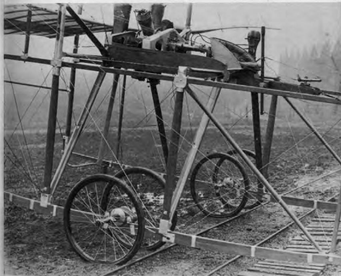
Close up shot of Valkyrie monoplane (Type B) of 1911 shows quite clearly the excellent workmanship and finish of early aeroplanes. Note the different types of joints and taping, the rubber cord shock absorbers on the undercarriage and the pilot's dashboard on the left side of the seat ('Flight International').
