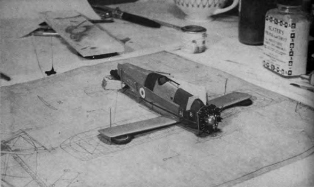
ABOVE: A simple rig to ensure correct setting up of wings and fuselage. This is the author's Siskin model being assembled. Note that the plan is laid on to a plastic ceiling tile and held in position with pins (or toothpicks). This ensures that the wings are correctly lined up and that the lower dihedral is correct. Note the simple plastic card support on top of fuselage to receive the upper wing. After the upper wing was fitted the support was merely cut at the rear end with scissors and it fell away.
