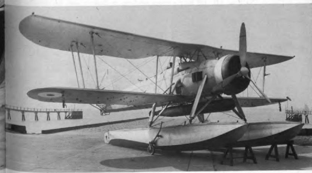
ABOVE: All metal float on Short Sarafand represents type used until virtual demise of flying boat in recent years. Note metal skinning of hull and sharp trailing edge of wing even on a very large machine such as this (Short Bros). BELOW: Modern floats fitted to a Fairey Swordfish. There is quite a large amount of surface detail on floats which should be reproduced in a 1:48 scale model such as the old Merit kit. More particularly, note the lugs, panels and sea rudder detail (MOD).
