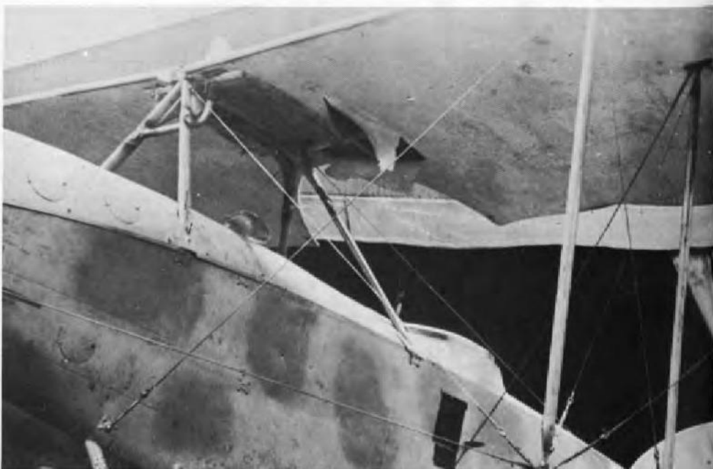
ABOVE: Close up of nose of SPAD XII shows radiator shutters in detail and meshwork behind. The propeller was geared as a 37 mm Peteaux gun fired through the hollow shaft. The SPAD XII carried a solitary Vickers gun for firing sighting bursts for the cannon. The tremendous recoil and slow rate of fire made this arrangement unpopular. BELOW: Wing mounted radiators should be visible on the under as well as upper surfaces of wings, as shown on this Albatros C.V (serial C1394/17) in May 1917.
