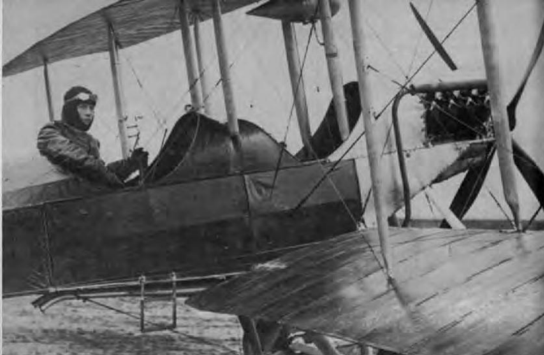
ABOVE: Sgt Parkhurst in the cockpit of a BE 2a, in 1913. Fuselage is a perfect example of the built-up box type. Note also that fabric was drum tight over wing ribs (MOD). BELOW: Line up of Hiero engined Albatros C-1s at an Austrian factory. Note typical plywood skinning of nose area surmounted by metal cowlings plates. Lateral radiators are seen quite clearly in this view.
