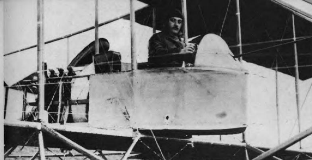
ABOVE: Maurice Farman Longhorn nacelle illustrates the 'Skeletal and partly covered' type of fuselage. Such detail as the metal facings to the holes for control wires and elevator rod are important when modelling such aircraft (Real Photographs).
