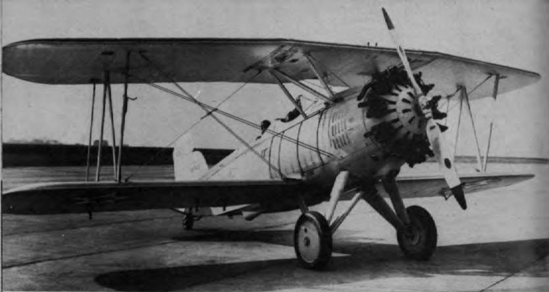
ABOVE: Typical metal propeller of the 1930s is shown here on a Curtiss 02-C1. The trademark indicates that it is a Standard Steel Propeller; note usual US Navy painted tips (from tip in: red, yellow and blue). 'Standard' trademark is dark red ellipse, with yellow lettering and yellow propeller. This type of propeller was used extensively by US aircraft in the 1930s (Smithsonian Institute). BELOW: Author's fine model of the Curtiss BFC-2 in 1:48 scale carries a propeller similar to the type shown above.
