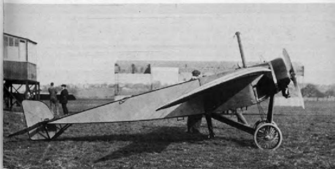
ABOVE: The original Morane monoplane showing the slab sided construction very well. This aircraft would make an ideal subject for simple box construction, note also camber of wing, and completely flat horizontal tail surfaces (elevators only). Anthony Fokker bought a damaged example of this type of machine and produced a virtual copy with his M5 monoplane although he simplified construction considerably and incorporated a better wing section ('Flight International').
