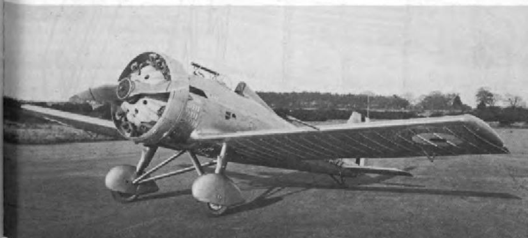
BELOW: An interesting and challenging model subject would be the Vickers Type 151 'Jockey' interceptor fighter of 1932. The project was abandoned after it failed to recover from a flat spin, the pilot bailing out. It is interesting to note the early all metal construction, metal propeller and formidable riveting (MOD).
