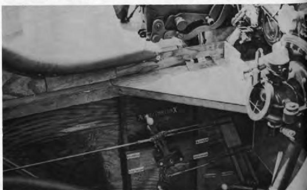
BELOW: Port side of pilot's cockpit in a DH 9a. Note unpainted wooden sides, breech of Vickers gun, top of basket seat, and small lights on dashboard (Imperial War Museum-Q63803).
