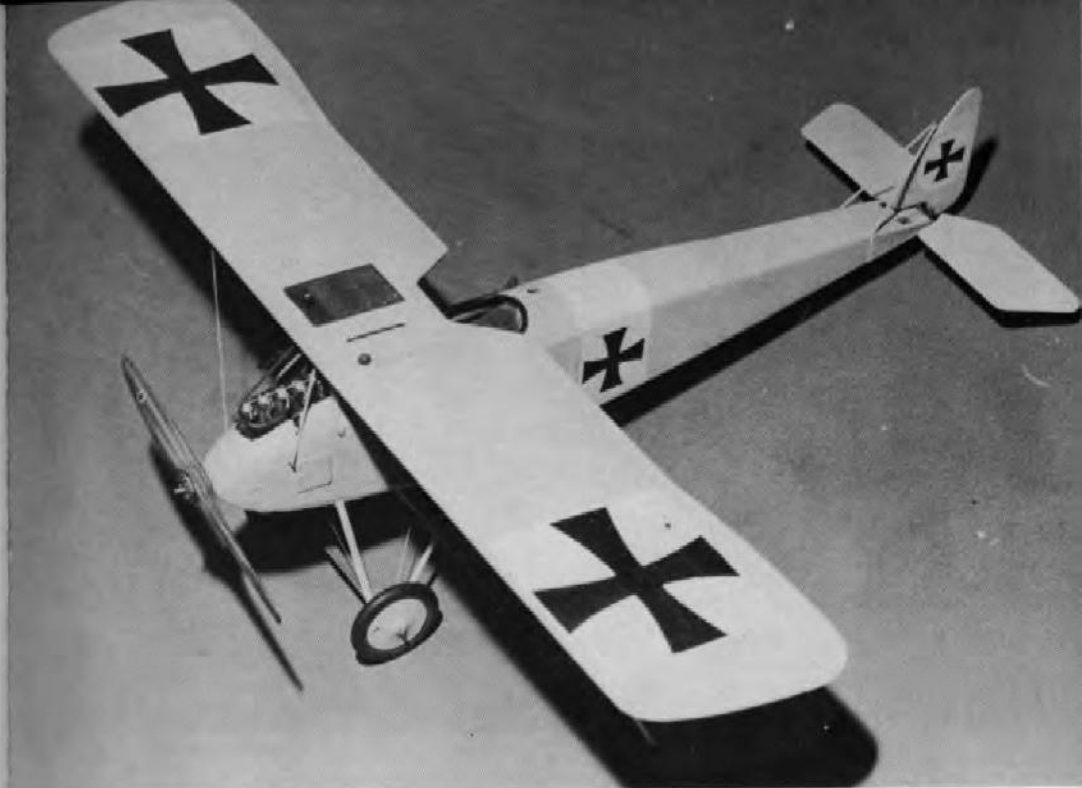
ABOVE: Author's neat model in 1:48 scale shows a multi-louvered radiator in the wing top surface made as detailed opposite. Note also the laminated propeller and the meticulously detailed engine. This is a Halberstadt D II, illustrated also in other pictures.
