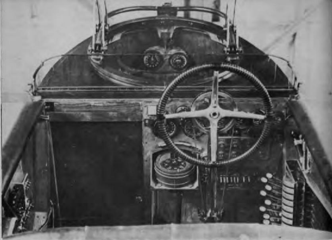
ABOVE: Pilot's compartment of Handley Page V/1500 is typical in layout of large multi-engined aircraft of the late 1914-1918 war years and early 1920s (MOD).
