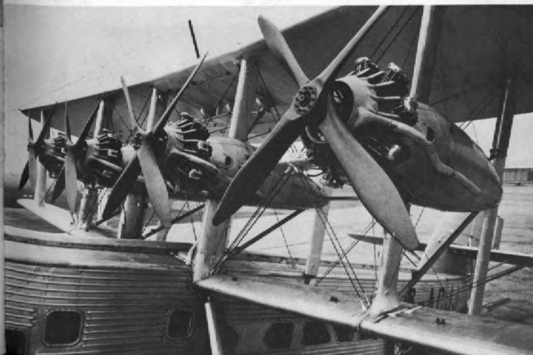
ABOVE: Surface detail on the Armstrong Whitworth Argosy airliner of Imperial Airways in the mid-1920s is shown well here, as is the undercarriage. Note also the external control wires ('Flight International'). OPPOSITE, TOP: Flush riveting lines on the Dornier DO-X can be depicted on plastic card by adapting a small cog wheel from an old watch and running it along a steel rule, or by 'embossing' with a pin point ('Flight International'). OPPOSITE: Short Scylla airliner of mid-1930s shows corrugated covering and drum tight fabric skinning of wings. Note engine and propeller detail.
