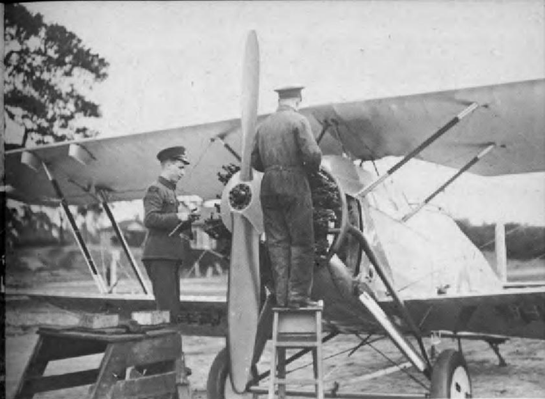
ABOVE: A good example of a flat conical boss carved integrally with propeller. Early Armstrong Whitworth aircraft used this type of propeller seen here on an Atlas General Purpose machine of No 4 Squadron in the early 1930s (MOD).
