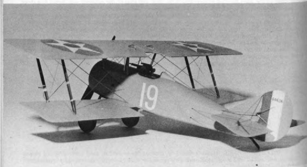
FOLLOWING PAGE: Author's model of Nieuport 24 bis (Nungesser's machine) in 1:48 scale. This was originally a Hawk kit of the 17c but a great deal of replacement was required. The only items of the original kit used in the final model were the fuselage which was re-skinned as described in the text, and the wheels. The kit propeller proved to be too weak and a new one was made from plastic card. The wings and tail assembly are made as described on the text and the cowl was moulded using the original kit cowl (which had been slightly reshaped and reduced with sanding) as a male mould. This model and the Thomas Morse and Voisin models shown in this book were all damaged when a shelf fell on them. They are all shown here as rebuilt illustrating the resilience of plastic card.
