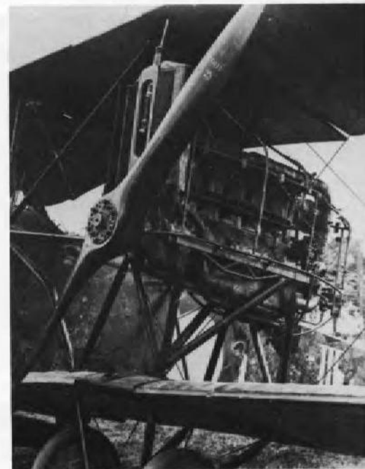
RIGHT: Wolff propeller on AEG GIII. This is the famous No G105 captured on December 23, 1917. The diameter of the Wolff propeller is 10 ft 3-8 inches and is made of laminations of walnut and mahogany making it rather dark in appearance. Radiator was of vertical tube type with adjustable shutters in front (Imperial War Museum - Q55028).
