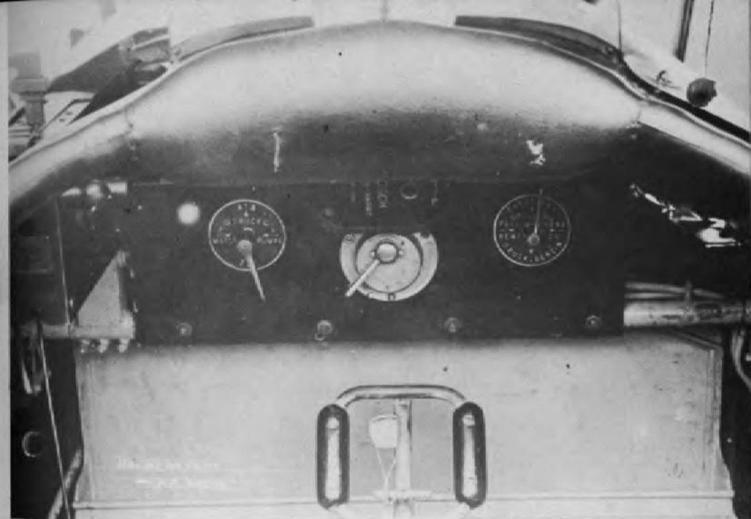
ABOVE: Cockpit of Halberstadt D II (Argus engine) of 1916 shows rudimentary dashboard. It was by no means uncommon for certain instruments to be mounted outside the cockpit altogether at this stage.
