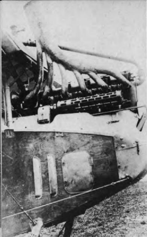
RIGHT: Nose of Breguet 14 shows typical louvred panelling common on many aircraft with nose radiator (1WM-Q58354).
