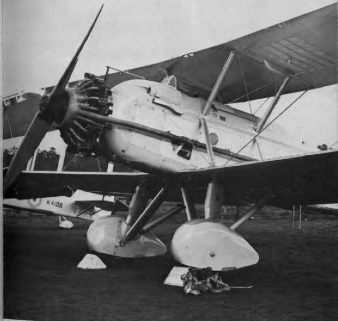
VICKERS VILDEBEEST: Note prominent collector ring and exhaust pipe of Pegasus engine arrangement typical of the period. Also many other details (FLIGHT INTERNATIONAL).
