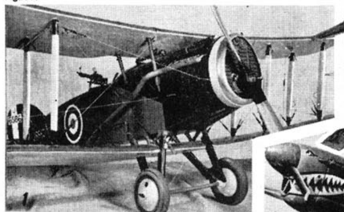
Fig. 56.—1. Bristol F2b fighter with all possible detail including scale prop for 10 c.c. petrol engine. 2. D.H. Comet with Ducted Fan Frog 500 has metallised covering and u/c as in Fig. 59.
