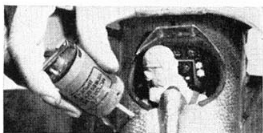
Fig. 109.—Pilots by Capt. Milani add character to his models. Bottom, use of electric-motor-driven eraser to simulate "engine turning" on metallised paper.
