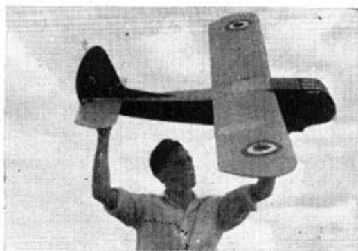
Fig. 1.—Accurate scale version of the Waco Hadrian troop carrier flies well from tow launch or when slope soaring.
