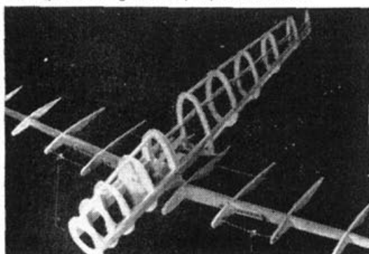
Fig. 40.—Author's Nakajima Tony fighter made of basic crutch construction with sheet wrapping for fuselage and wing surfaces, top and bottom.
