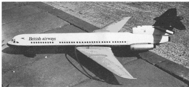
HSA Trident 3 is ambitious but perfectly feasible for compressed air. Note position of air take near leading edge and mid-chord anchor point for RTP cable.
