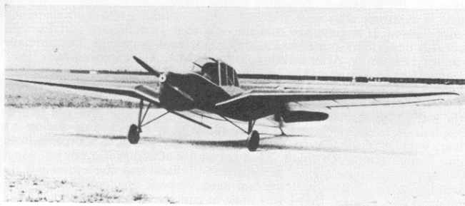
In the same year as the "Sparrowhawk" 1936, the author acted as project engineer for the Koolhoven FK-53 "Junior", side-by-side light plane with 60 h.p. Walter "Mikron" four cylinder in line engine. Unfortunately, it was not a success; only two prototypes being built.
