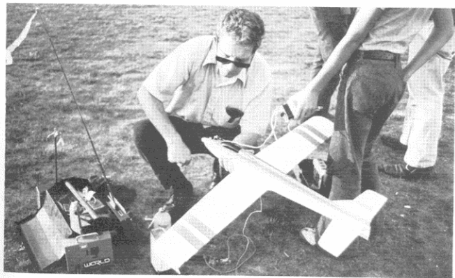
Frank Baker starts his .049 in the Pacer at Madison. Model has foam wings, 40 in. span.
