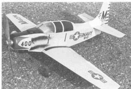
Marvin Martinez made this Skyraider for Class 1 using a K & B 40 with 9x7 in. propeller.
