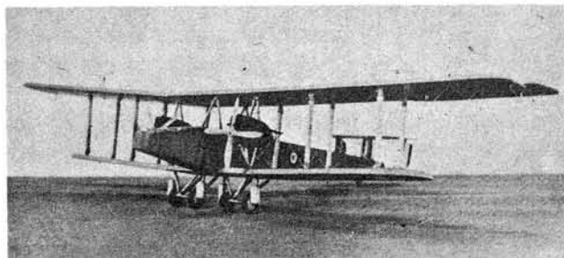
British Handley-Page of WWI. Had two Liberty engines of 400 hp each; 97 mph. Span 100 ft.; weighed 14,000 lbs. fully loaded.
