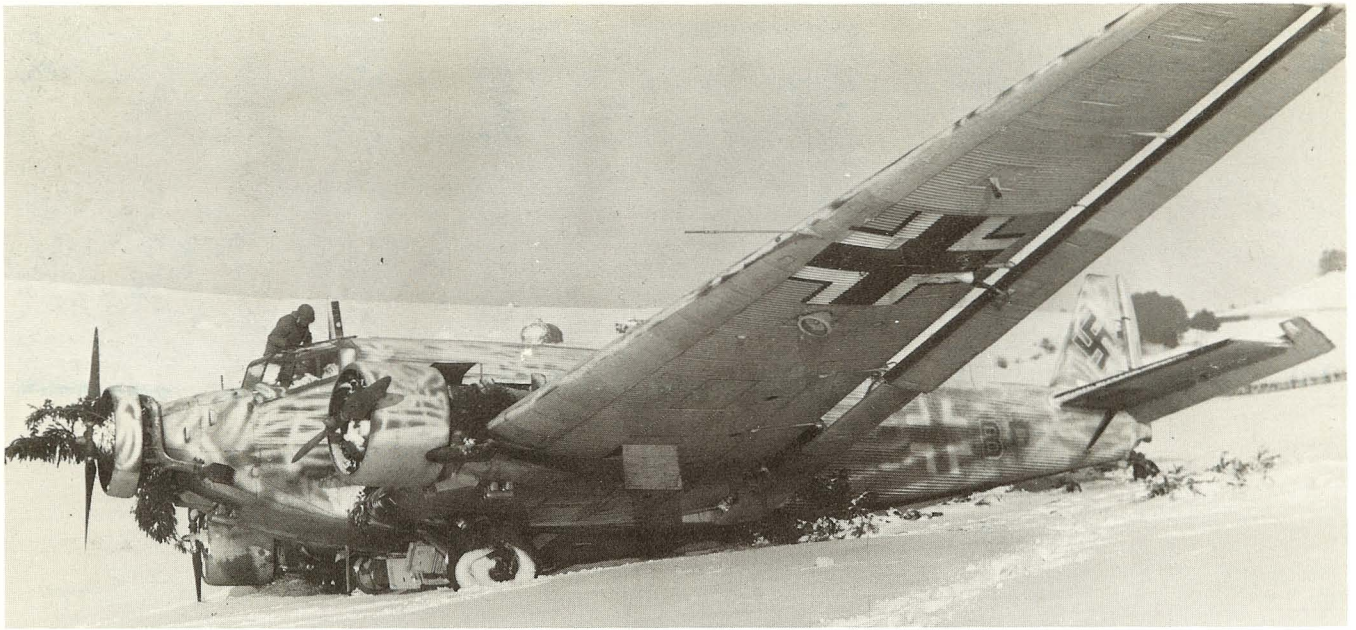
Above: This Ju 52/3m g5e, W.Nr. 7279, 4V+BP (originally TG+ES) was one of a pair which force-landed on January 22, 1945, southwest of Asselborn, Luxembourg. Fitted with flame dampers for night operations, the standard 70/71/65 has been altered by the liberal application of white over uppersurfaces, while the outer portion of the wing's undersurface was in yellow. Reportedly, this machine was on strength with III./TG 2. Left: Logical successor for the Ju 52 would have been the Ju 252, but only 25 were built. This example, Ju 252 V5, DF+BQ, was in 70/71/65, with a yellow tail band. It was operational with LTSt. 290 based at Berlin's Tempelhof airfield early in 1943. All 25 examples of the "Herkules" were considered prototypes being retained for special missions and VIP transports. Below: This Ju 352 A-1, N1+CX, originally attached to Grossraumtransp. st. based at Tutow, was captured after the war and used by the RAF for various ferry missions as AM 18. Camouflage was 70/71/65.
