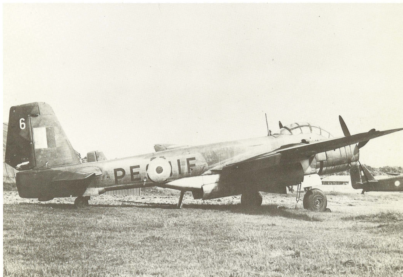
The high performance Junkers Ju 388 K-1/V6, W.Nr. 500 006, PE+IF, prototype for the Ju 388 K-1 series, was completed during the summer of 1944. Captured intact by British Forces, it was shipped to England for evaluation. Camouflage in all probability was 70/71/65. Ultimately, however, the new colors, 81/82/76, would have been employed. German national markings, except for the underwing crosses, were the usual simplified white outline variety. The white number six applied to the rudder denotes prototype number 6.
