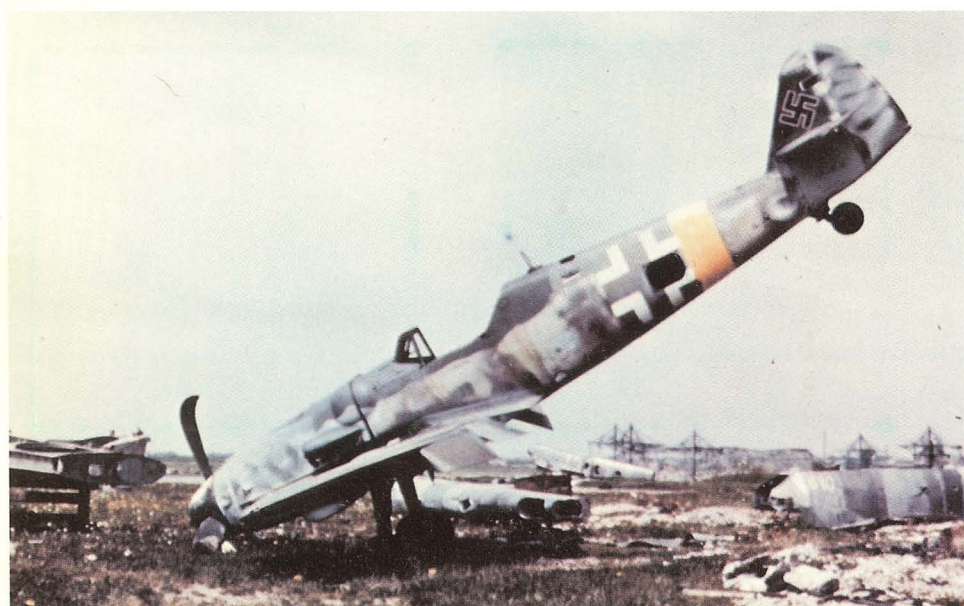
Above: A photo-reconn Messerschmitt Bf 109 G-10/R2, W.Nr. 770 269, "Black 12" of 2./NAG 14. Camouflage was essentially 74/75/76 with a dense mottle of 02 and 74. Prop blades and two-thirds of the spinner were 70 with one-third 21. A red cap, fitted over the aperture, indicated the engine-mounted weapon was not fitted. The MW 50 powerboost fuel triangle was red and white with yellow trim. The rear yellow and white triangle identified the location of the engine fuel primer tank. Left: Photographed at Messerschmitt's Augsburg plant in May 1945, this Bf 109 G-14, W.Nr. 165 545, carries an interesting camouflage of Gray-Green 74 and Gray-Violet 75 over Light Blue 76. The significance of yellow tail bands at this juncture in the war is unclear, but it is believed to have indicated that the aircraft operated on instruments. Below: The remains of a Bf 109 G-6, found by U.S. troops following demolition by retreating Luftwaffe personnel. Compare this fighter trainer with the one at the bottom of page 43.
