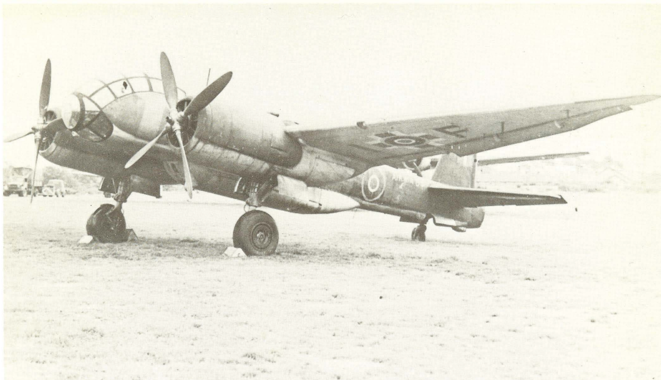
The high performance Junkers Ju 388 K-1/V6, W.Nr. 500 006, PE+IF, prototype for the Ju 388 K-1 series, was completed during the summer of 1944. Captured intact by British Forces, it was shipped to England for evaluation. Camouflage in all probability was 70/71/65. Ultimately, however, the new colors, 81/82/76, would have been employed. German national markings, except for the underwing crosses, were the usual simplified white outline variety. The white number six applied to the rudder denotes prototype number 6.
