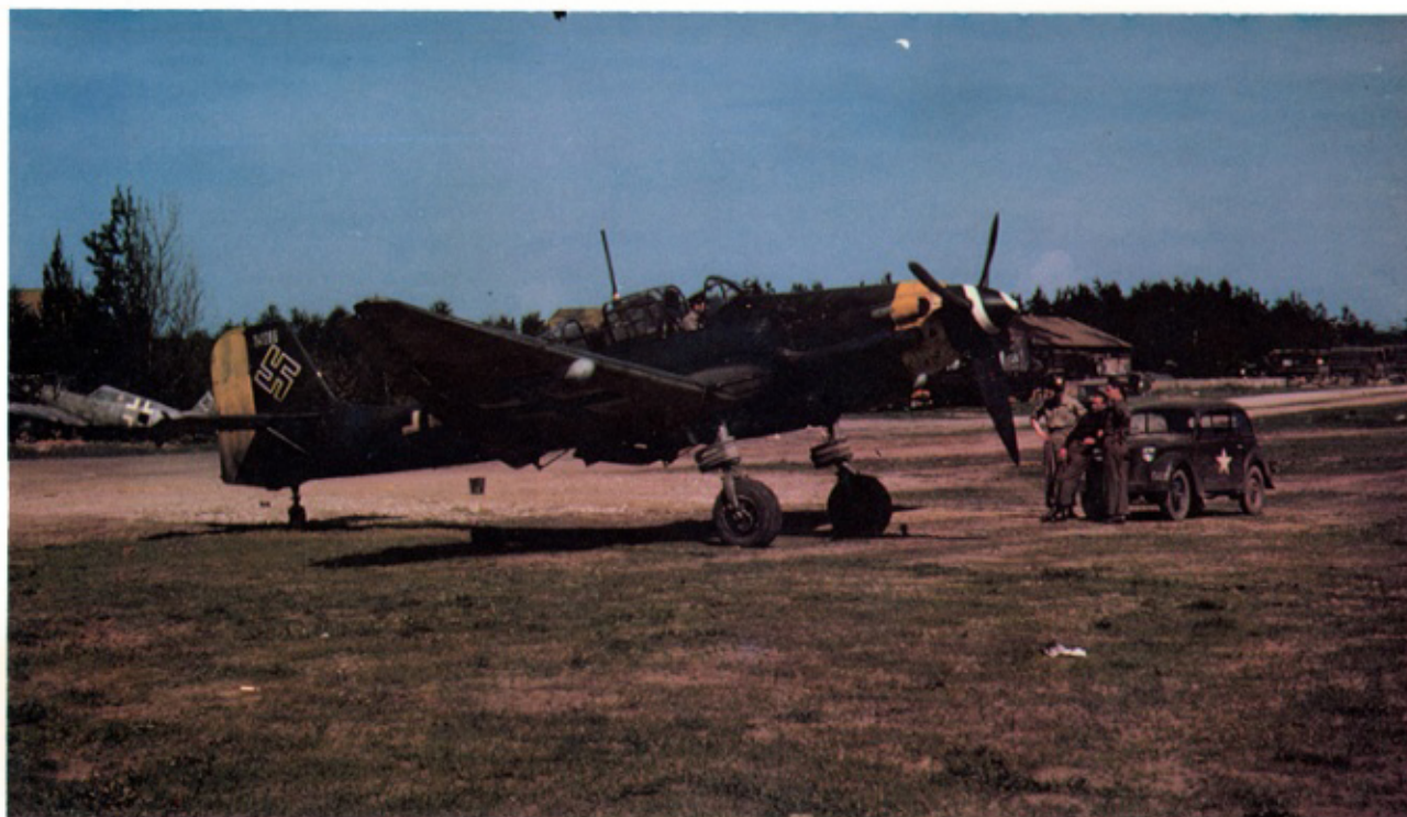
Above: Surrendered by its crew at Fürth, this Junkers Ju 87 D-5, W.Nr. 141 286, is camouflaged 70/71/65 with yellow tactical colors applied to the nose, rudder and underside wing tips. Note the absence of wheel trousers exposing the landing gear legs painted RLM Gray 02. Below: This Ju 87 G-2 was captured in Pilsen, Czechoslovakia. Although the color has badly sepiad over the years, the basic camouflaged coloring of 70/71/65 is still obvious. Like the Stuka above, this example carries the tactical color yellow around the cowlings; but unlike the machine above, the flame-damping exhaust tubes are angled to eject downward. The spinner was finished in Black-Green 70 while the Junkers VS 11 wooden prop blades were in Dark Green 71.
