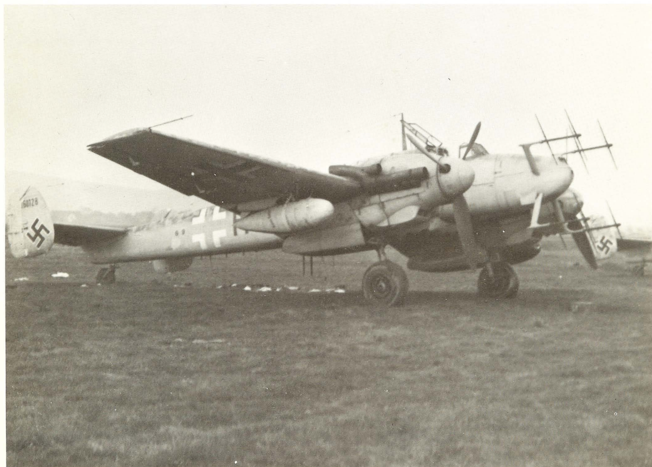
Below: Camouflaged overall Light Blue 76 with Gray-Violet 75 uppersurfaces, this Bf 110 G-4, A.Nr. 160 128, G9+HT was operational with 9./NJG 1. Captured at Fritzlar in early April 1945, this machine was equipped with 300 Liter drop tanks.
