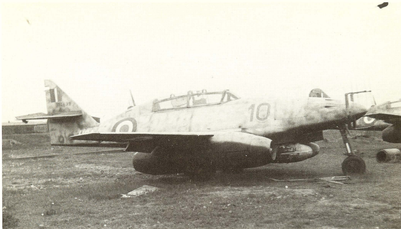
Above: Lacking its rudder, this Messerschmitt Me 262 B-1a/U1, W.Nr. 110 635, "Red 10" shown here at Dizier was one of the two-seat night fighters acquired by Col. Watson's crew at the close of the war. Although carrying RAF roundels and fin flash, the rear fuselage bears the inscription "USA 1". Most of the two-seat conversions were carried out by Blohm & Voss and their camouflage was fairly consistent from one aircraft to another, being Light Blue 76 over top surfaces with a mottle of Gray-Violet 75. Red 10's wing uppersurface was similar to the fuselage mottle, this being applied in a random pattern of serpentine Gray-Violet lines. The simplified black outline cross was applied to the fuselage and upper wing surfaces. The fin carried a simple solid black
