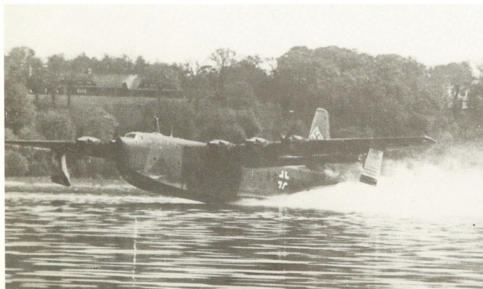
Left: With a wing span of 197 ft. 4¼ in., the BV 238 V1, RO+EZ, was a very large flying boat completed in early 1944 for maritime transport and patrol duties. Camouflage colors were standard 72/73/65, with the simplified white outline insignia at all positions except for the outboard underwing crosses. Prior to the completion of flight trials, it was sunk at its mooring on Lake Schaal by American P-51s.
