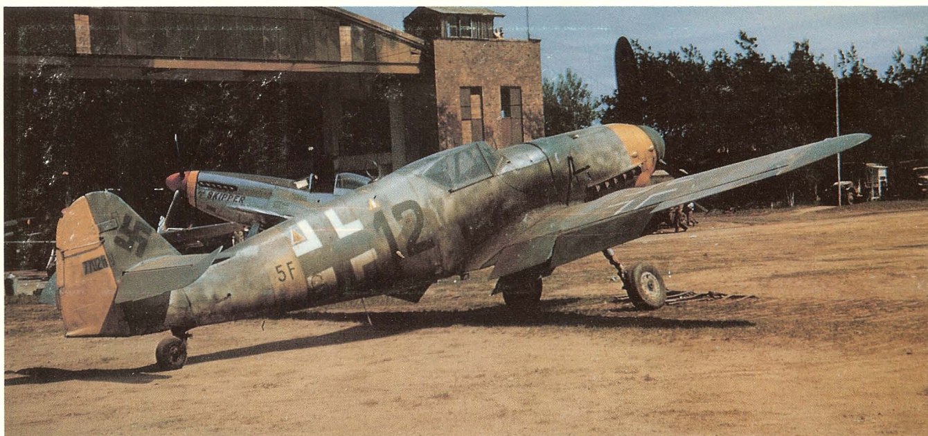
Above: A photo-reconn Messerschmitt Bf 109 G-10/R2, W.Nr. 770 269, "Black 12" of 2./NAG 14. Camouflage was essentially 74/75/76 with a dense mottle of 02 and 74. Prop blades and two-thirds of the spinner were 70 with one-third 21. A red cap, fitted over the aperture, indicated the engine-mounted weapon was not fitted. The MW 50 powerboost fuel triangle was red and white with yellow trim. The rear yellow and white triangle identified the location of the engine fuel primer tank. Left: Photographed at Messerschmitt's Augsburg plant in May 1945, this Bf 109 G-14, W.Nr. 165 545, carries an interesting camouflage of Gray-Green 74 and Gray-Violet 75 over Light Blue 76. The significance of yellow tail bands at this juncture in the war is unclear, but it is believed to have indicated that the aircraft operated on instruments. Below: The remains of a Bf 109 G-6, found by U.S. troops following demolition by retreating Luftwaffe personnel. Compare this fighter trainer with the one at the bottom of page 43.
