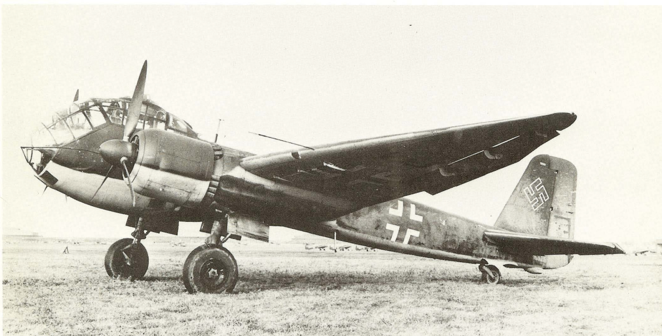
Left: This war-weary Ju 188 A-2, W.Nr. 160 078, has received several replacement parts during its service career, but the basic 70/71/65 scheme seems to dominate. The rudder may well have been covered with a marking color, such as yellow; but most likely it is merely a replacement item painted RLM Gray 02. Note the duplication of the serial number on the fuselage in addition to the model number immediately above the center of the fuselage simplified black outline cross.
