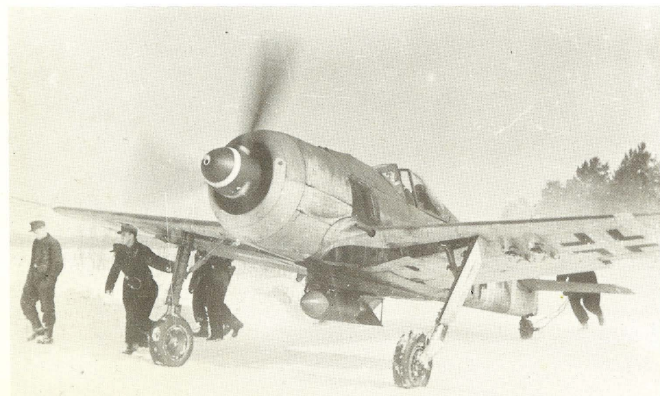
Left: This Fw 190 F-8/R1 serving with SG 2, taxis into takeoff position in Hungary early in 1945. Note the tactical "V" marking under the port wing which is identical to the aircraft on page 69. The "V" motif overlaps the top surface, extending for 56 cm on the outboard side and 38 cm on the inboard side. This marking also was employed by Oberstlttn Rudel of Stab II./SG2. Undoubtedly camouflage was similar to the color illustration on page 69.
