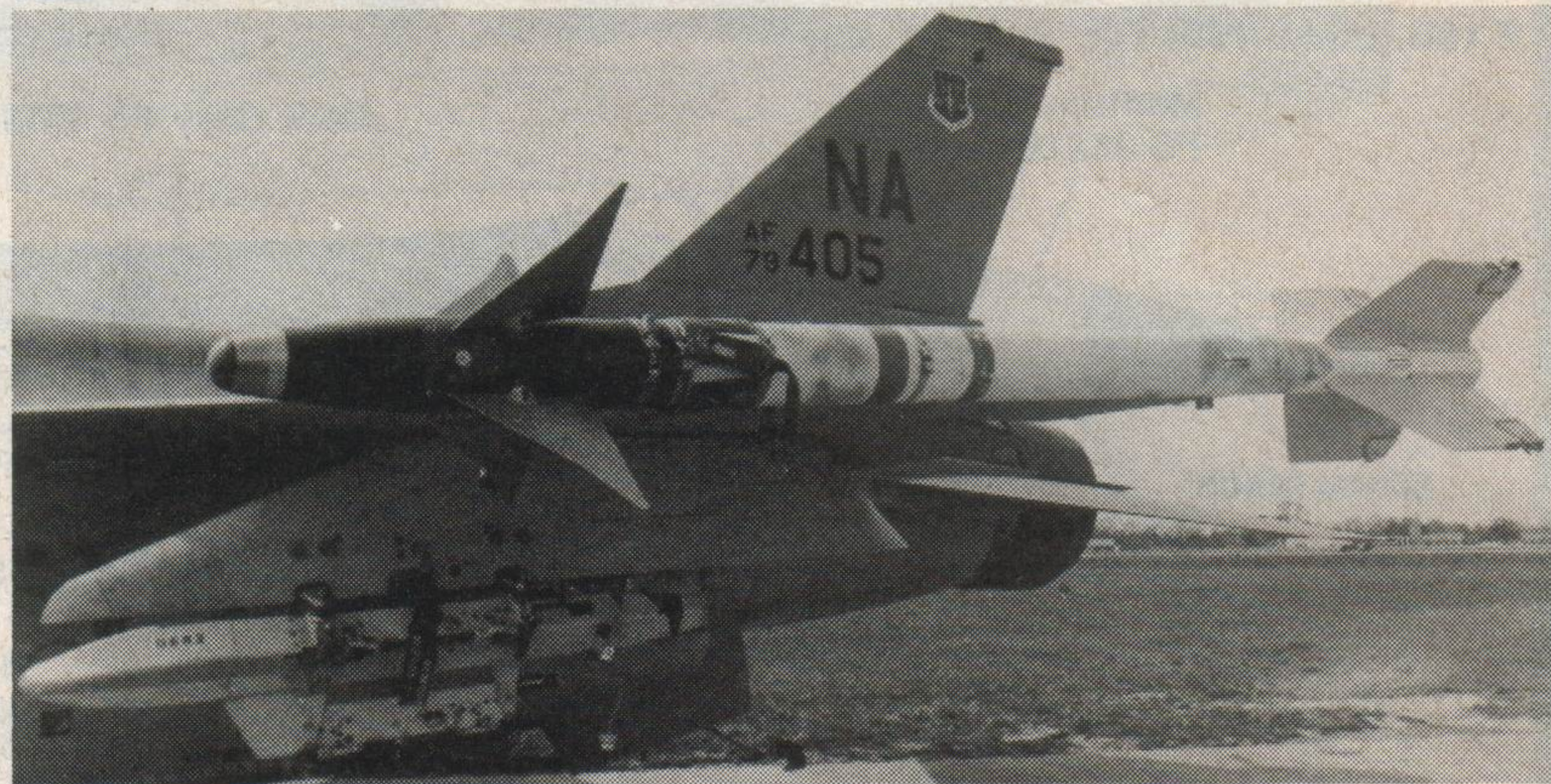
130. F16 79-405 configured for the ground attack practice mission, April, 1981. 131. Rear port tail detail looking forward – note slot at root, an oft-missed feature. 132. Blue bands on this AIM-9L Sidewinder missile identifies it as a practice round. A Triple Ejector Rack is mounted in the outer underwing pylon.
