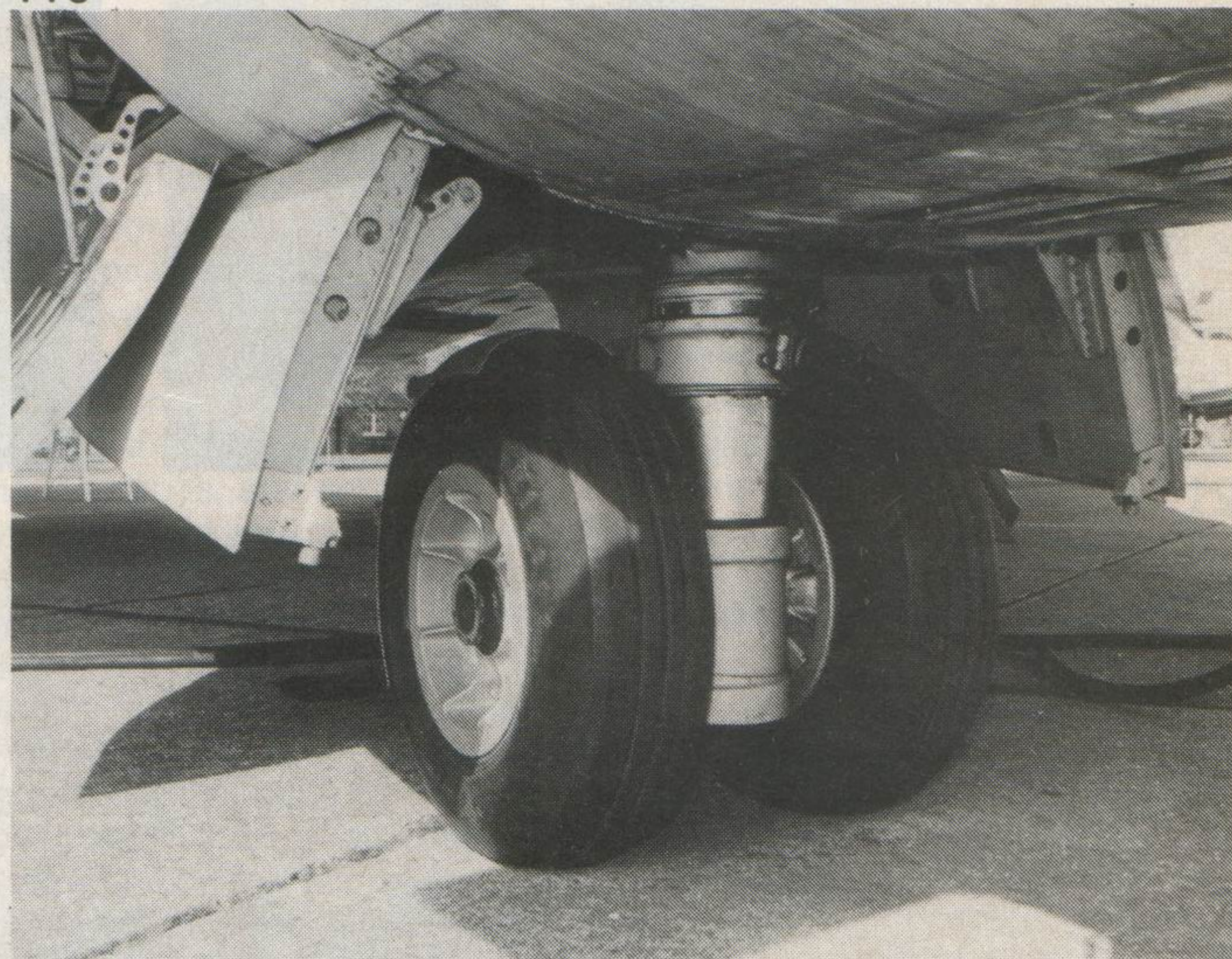
115. Front view of the nose undercarriage – note the small clearance between tyres and mudguards. 116. Bomb bay detail. Note the two fuel tanks – standard for the 'two-pointer' tanker versions, petal in front of bay to break up the airflow and the flaps in fully down position. 117. Victor K2 of 57 Squadron in standard camouflage scheme – all colours are matt.
