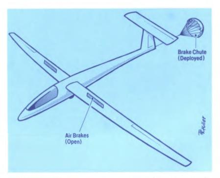
to be employed for training purposes and on which, conveniently, all the control wires were exposed. We have superimposed on this picture some of the secondary controls now found on most gliders for glide path control.
