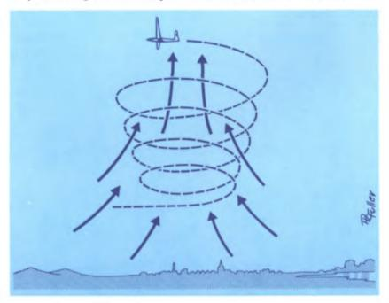
of a column or funnel. More often than not such a column known to glider pilots as a thermal — is sufficiently large for him to keep within, provided he rotates in fairly tight circles. By doing this he effectively spirals his way upwards: like someone climbing a spiral staircase.
