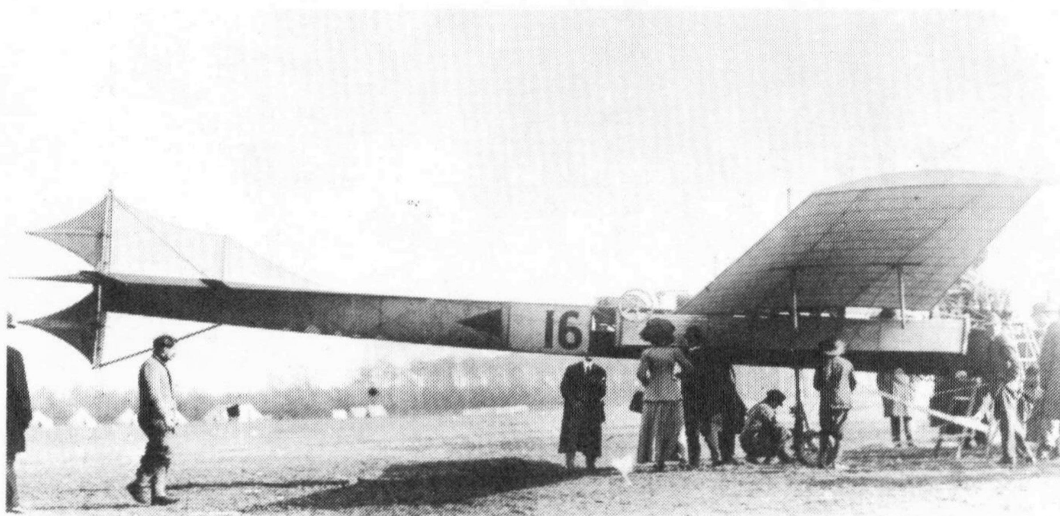
The advancement in aircraft design exhibited here in 1908 was quite revolutionary. Note rudder and elevator control surfaces. The entire wing panels were moved for lateral control. Photos courtesy of Leonard Opdycke, WW I Aeroplanes.
