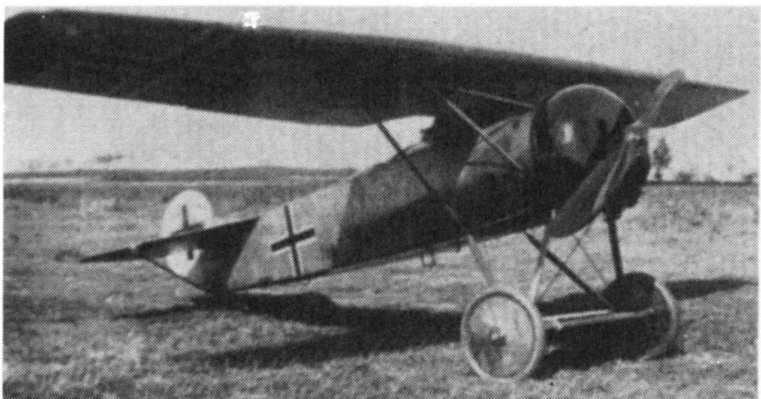
*The Fokker D.VIII was unique in several respects. Full cantilever wing, no struts and good performance gave its pilots a tremendous advantage over their foes. Photo courtesy of "Fokker, the Man and the Aircraft."*
