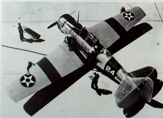
Left: A North American SNJ-3 with Red wing and fuselage stripes to indicate it is an instrument trainer prior to May 1942.
