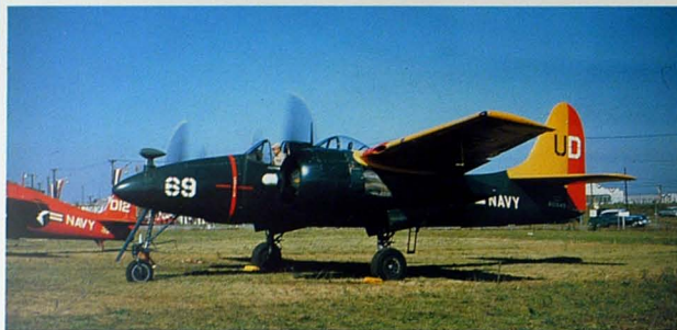
Left: A Grumman F7F-2D, Tigercat, of VU-4 which served as a drone controller. The drone pilot sat in the second seat to fly the drone F6F-5K (see p. 57 top).
