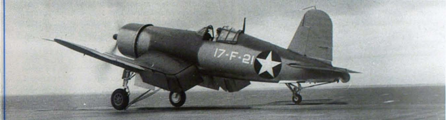
Right: An early production Vought F4U-1 Corsair photographed during the summer of 1942. Note that this aircraft has the older braced canopy which was later replaced with a blown hood and higher seat for improved forward visibility. Below: A Consolidated PBV-5 at NAS Pensacola in 1943. While this airplane is painted in the basic camouflage, as used in the Fleet, the upper wing surface has been painted Orange Yellow for better visibility in the event of a forced landing during a training flight. This was not an uncommon practice in the Training Command. Bottom Left: A VF-5 Grumman F6F-3 prior to launch from the deck of the USS YORKTOWN (CV-10) in May 1943. Bottom Right: This stern view of a PBV-5 illustrates the uneven line dividing the White and Intermediate Blue and how White was not to be applied above a point where it could be seen from above.
