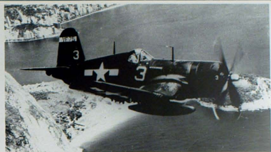
Right: F4U-4 of VF-75 March 1946. The use of the squadron designation on the vertical tail is only known to have been used by the squadrons of CVBG-75 aboard the USS MIDWAY (CVB-41).
