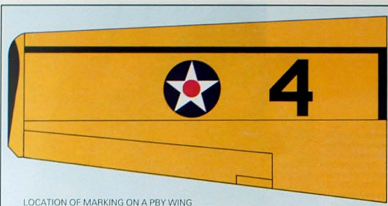
LOCATION OF MARKING ON A PBY WING
