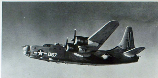
Left: A Consolidated PB4Y-2, in August 1942, with the three tone camouflage showing the engine nacelles painted in the same manner as the fuselage. The White on the fuselage produces Counter-Shadowing. D67 code is unknown. Middle Left: Note how the under portion of the engine nacelle on this PBJ-1J is painted to blend with the under wing surface and provide Counter-Shadowing. Middle Right: A Piper AE-1 obtained from the Army in New Guinea and operated for a short period by the US Marine Corps. USMC was applied to the tail but all other painting and markings including the aircraft serial number remained Army markings. Bottom: Goodyear FG-1D painted overall Sea Blue with no markings other than those assigned by the pool.
