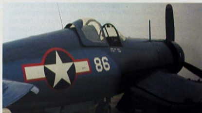
Left: This F4U-1 Corsair photographed at Espiritito Santo, New Hebrides, shows how quickly the paint can fade in tropical climates.
