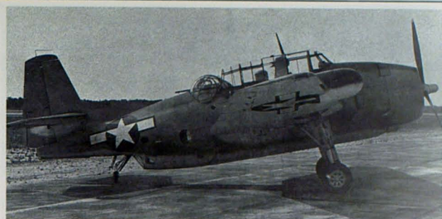
Right: General Motors TBM-1C clearly shows the Counter-Shadowing to help eliminate the shadow caused by the horizontal stabilizer and the wing. Note the treatment of the radar fairing on the wing as though it was an engine nacelle. This aircraft is assigned to NAS Patuxent River for technical testing.
