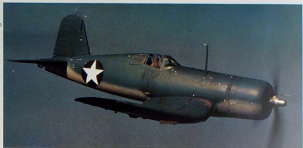
Right: An early production Vought F4U-1 Corsair photographed during the summer of 1942. Note that this aircraft has the older braced canopy which was later replaced with a blown hood and higher seat for improved forward visibility. Below: A Consolidated PBV-5 at NAS Pensacola in 1943. While this airplane is painted in the basic camouflage, as used in the Fleet, the upper wing surface has been painted Orange Yellow for better visibility in the event of a forced landing during a training flight. This was not an uncommon practice in the Training Command. Bottom Left: A VF-5 Grumman F6F-3 prior to launch from the deck of the USS YORKTOWN (CV-10) in May 1943. Bottom Right: This stern view of a PBV-5 illustrates the uneven line dividing the White and Intermediate Blue and how White was not to be applied above a point where it could be seen from above.
