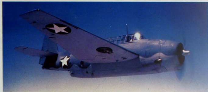
Right: The underside of this Grumman TBF shows the Sea Blue carried over the leading edge of the wing to insure that no white is visible from above. Below: A Vought SB2U-2 of Scouting Squadron 9 (VS-9) in the two tone scheme about to catch the arresting cable aboard a carrier in October 1942. Note the fiddle bridge in the foreground to raise the cable off the deck to assist the aircraft's tail hook to catch the arresting cable.
