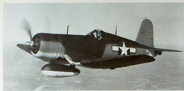
Left: Vought F4U-1D Corsair in three tone camouflage. The centerline fuel tank is painted in two colors in an attempt to conform to the basic camouflage. A definite color is apparent in this photo from the Sea Blue of the upper fuselage and the Insignia Blue of the national aircraft insignia. Bottom: A new Grumman F6F-3, Hellcat, shown over Long Island, New York during the summer of 1943. The new national insignia, shown on this Hellcat, was in force barely three months before it was changed.
