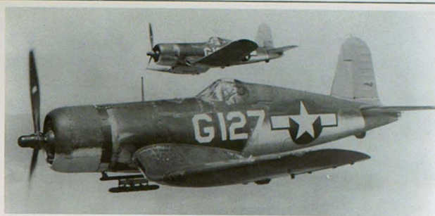
Right: This Vought F4U-1D clearly shows the Intermediate Blue tail color. The necessity of walking on the painted wing surface soon wore the paint off, as can be seen on this training squadron aircraft. A practice bomb rack for miniature bombs is carried on the fuselage center station.
