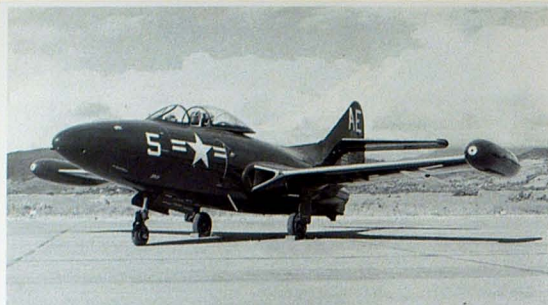
Left: A VMF-115 Grumman F9F-2B Panther. The suffix "B" denotes the aircraft has been modified with racks to carry bombs and rockets.
