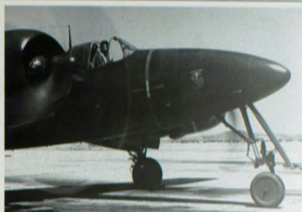
Right: A Grumman F7F-4P assigned to Marine Photographic Squadron 254 (VMP-254) in 1948, showing the propeller warning stripe and the identification of an ammunition box access door.
