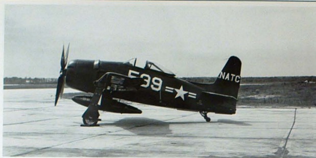
Left: In late 1949, this Grumman FBF-2 was assigned to NATC Patuxent River. Maintenance instructions such as TIRE PRESSURE 100 POUNDS on the landing gear fairing as well as instructions on the Mk-12 external fuel tank are visible. Below: A FJ-1 assigned to a fleet squadron still carries a variety of service markings along with its unit and individual markings.
