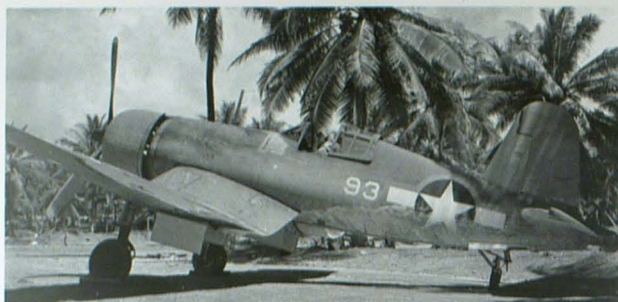
Left: This F4U-1 Corsair photographed at Espiritito Santo, New Hebrides, shows how quickly the paint can fade in tropical climates.
