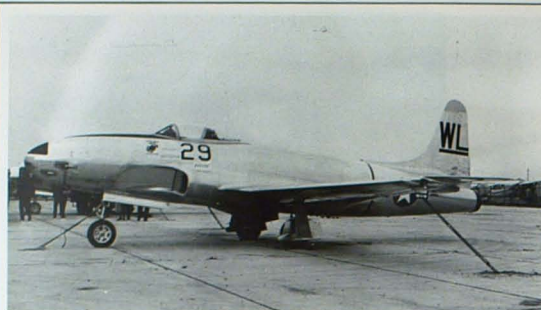
Left: A bare metal T-1 assigned to VMF-311 in 1948. Note the Red warning stripe around the aft fuselage in line with the turbine blades. Bottom: Another VMF-311 Lockheed T-1 with numerous safety and service instructions stenciled on the bare metal skin.
