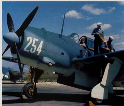
Left: Curtiss SB2C-3 Helldiver in the three-tone paint scheme. Note the transition from Sea Blue—Intermediate Blue—Insignia White on the forward fuselage. Middle Left: This Grumman F6F shows how an airplane, viewed from below, should appear to be White with the edges shading into Intermediate Blue. Middle Right: Curtiss SB2C carries a large identification number on the cowl which is only a sequential number not a unit identification number.
