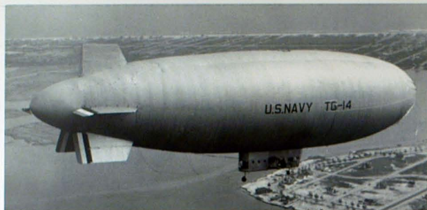
Left: Nonrigid airships carried a national aircraft insignia on the centerline of the envelope, both top and bottom, as well as the Red, White and Blue stripes on the moveable control surfaces.
