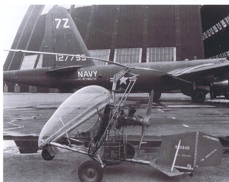
Above: A close-up of a special one-man helicopter under test at NAS South Weymouth during the 50s. Data on the fin refers to it as the GB-1, Ser-001, N10540, Gurleybird. It is unclear if this was a private venture or an official government-approved project.
