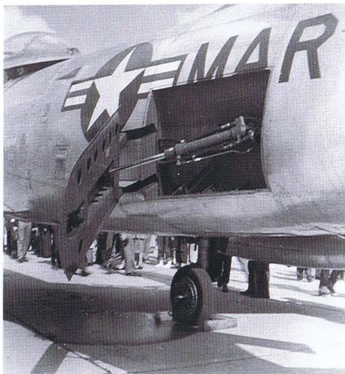
Left: Inner surfaces of speed brakes were painted red as a warning to those working around the aircraft.
