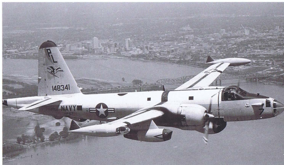
Right: This P2V-7 of VP-67 has the solar heat reflecting white top to reduce the temperature of the cabin for those operating all the antisubmarine warfare equipment. Colorful tail designs were a feature of the VP community.
