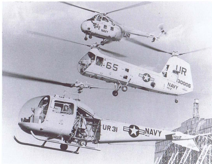
Left: These Light Gull Gray Sikorsky HO4S-3, Piasecki HUP-2, and Bell HUL-1, all assigned to Helicopter Utility Squadron 2, illustrate the difficulty in specifying a standard placement of markings due to the varied configuration of the early helicopters. Below: A Beech SNB-5 assigned to Helicopter Anti-Submarine Squadron 2 for utility work is painted in a variation of the high visibility scheme.
