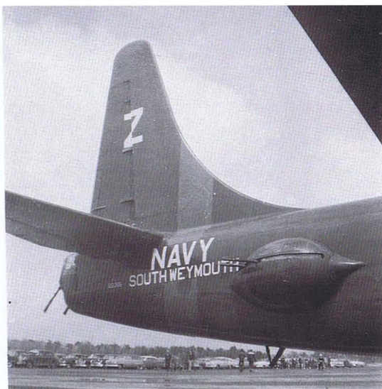
Left: This photograph of a consolidated PB4Y-2 tailsection is another example of how the aircraft configuration could vary the placement of insignia and markings. Due to the location of the side gun turrets on the PB4Y-2 Privateer, the reserve fuselage band and base name had to be applied much further aft than normal.
