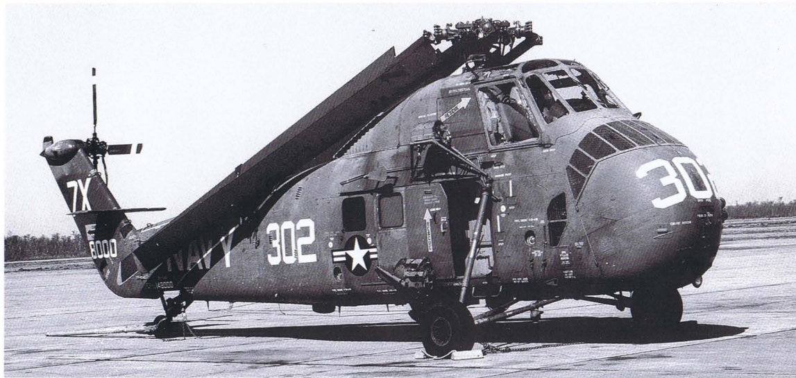
Opposite Right: This VMF(AW)-1 Douglas F4D-1 is shown at MCAS El Toro, California with colorful tail and drop tank stripes on an otherwise standard finish. Left: A New Orleans-based HSS-1 shows a multitude of service markings and rescue arrows to advantage. Notice how the national aircraft insignia will be covered when the door is opened in flight. Bottom: The location of the name on the undersurface of the right wing of this F8F-2 is a little unusual. This aircraft was assigned to the Navy Post Graduate School at Monterey, California for students to maintain flight proficiency. Bottom Right: These colorfully painted F9F-2s were operated by Advanced Training Unit 206 at NAS Pensacola.
