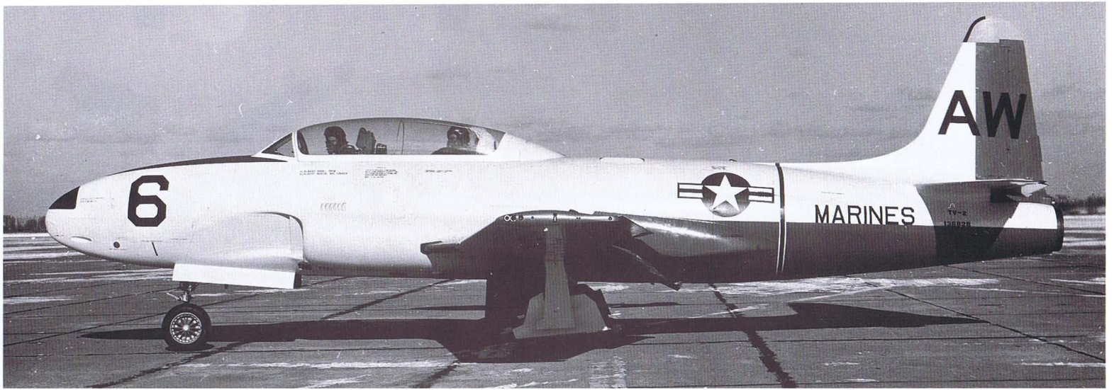
Above: A Lockheed TV-2 of Headquarters Squadron, Marine Aircraft Group 24 with high visibility scheme again shows the concern over the early turbine wheel throwing a blade. Left: Due to their small size most technical markings such as these on a F9F-8T do not show on photographs of the entire aircraft. Below: The rain erosion Cora-Guard on the leading edges of the wing and tail surfaces on this FJ-3 was dull aluminum, while the distinctive markings are red outlined with white.
