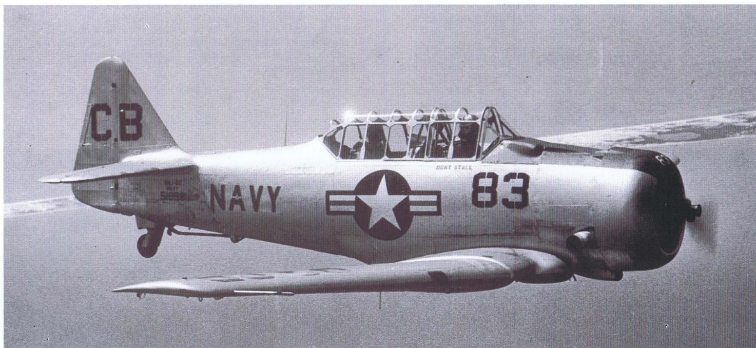
Above: This SNJ-SC is assigned to Carrier Qualification Training Unit 4 at NAAS Correy Field in 1950. The C modification shows that these airplanes have been modified with a tail hook for carrier operations. The legend under the lip of the pilot's canopy DON'T STALL was a gentle reminder each time a student climbed in. Left: A two-plane echelon of bare metal Lockheed TV-2s. These two-place jet trainers are assigned to Advanced Training Unit 200 based at NAAS Kingsville, Texas. Right Above: This is an F4U-ID with the additional reserve markings of base name and International Orange fuselage band. Right: NAVY has been applied higher than usual on this AF-2S Guardian to make the base name OAKLAND more visible in the center of the International Orange band.
