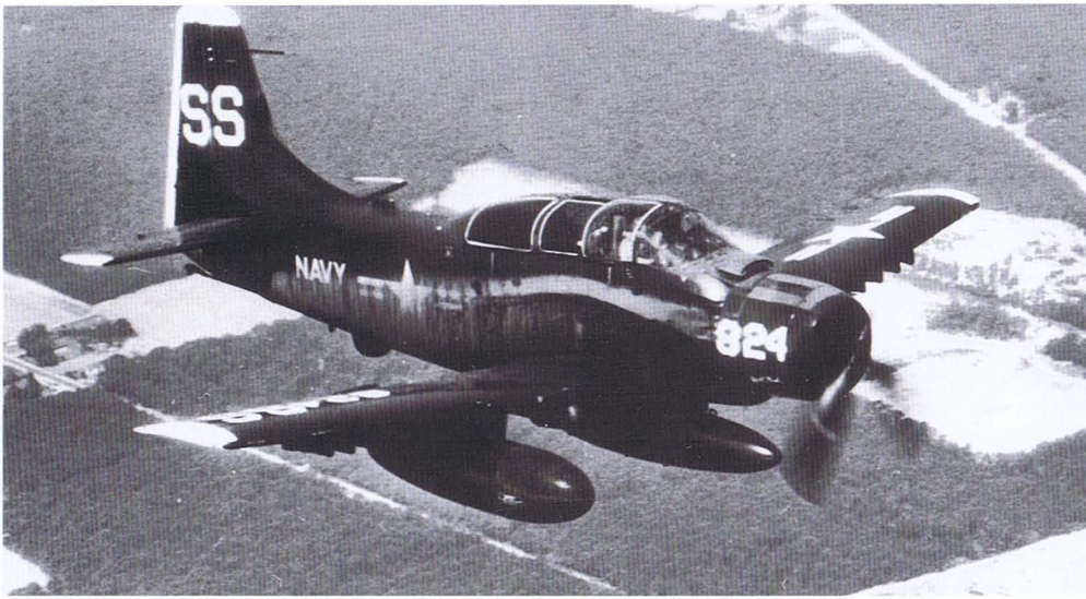
Left: Soon to become VA(AW)-33, this Douglas AD-5N of VC-33 is about to have the national aircraft insignia obliterated by exhaust stain. Opposite Right: This Utility Squadron 3 F4D-I clearly illustrates the need to position the national aircraft insignia on the forward portion of the fuselage.
