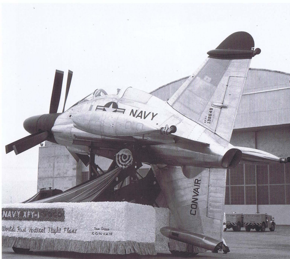
The Convair XFY-1 Pogo, was powered by an Allison VT40-A-14 turboprop capable of developing almost 7,100 hp during take off. The pilot sat in a gimbal-mounted seat which could tilt forward 45 degrees when the aircraft was in the vertical position. As the Pogo rotated to horizontal flight, the pilot's seat also rotated to its normal position. The XFY-1's landing gear consisted of four small castoring wheels. Ground tests conducted with Pogo indicated that it could remain in a stable vertical position up to 26 degrees from level before it was in danger of toppling.
