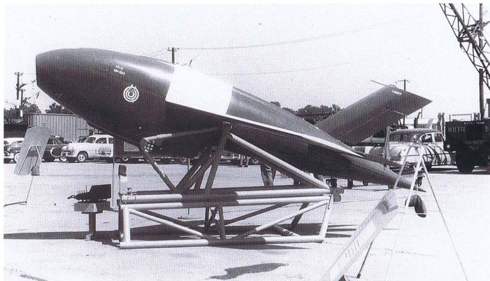
Left: The diminutive Ryan Firebee target drone was a high-speed jet-powered drone built for all three services but used by the Navy under the designation KDA-1. It was to be used for fleet anti-aircraft, aerial gunnery and guided missile training. On the opposite page, artist Dave Power has graphically depicted how the Firebee was to be carried aloft by a special version of the Neptune. Our photograph shows an Air Force Firebee (Q-2), but the Navy version was identical.
