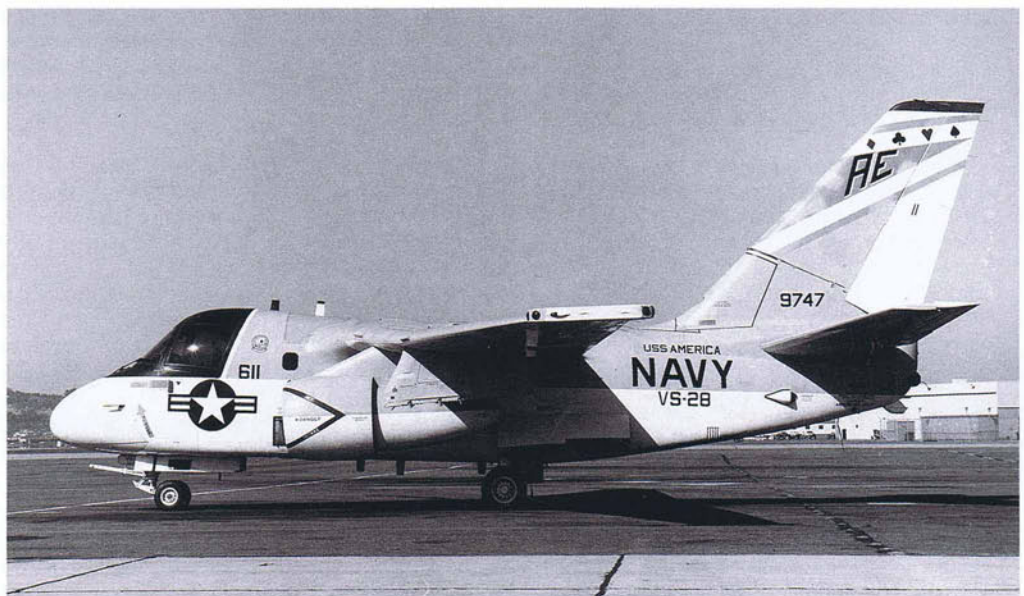
Above: A two-tone blue camouflage tested at the Navy Fighter Weapons School. Right: The hard line separating the Insignia White and Light Gull Gray on the fuselage of this S-3A is repeated on the engine nacelle rather than the normal blending of the colors. Below: "Mongoose" an A-4E stripped of all equipment except rudimentary avionics was flown at the Navy Fighter Weapons School in this three-tone Sand, Brown and Green Camouflage.
