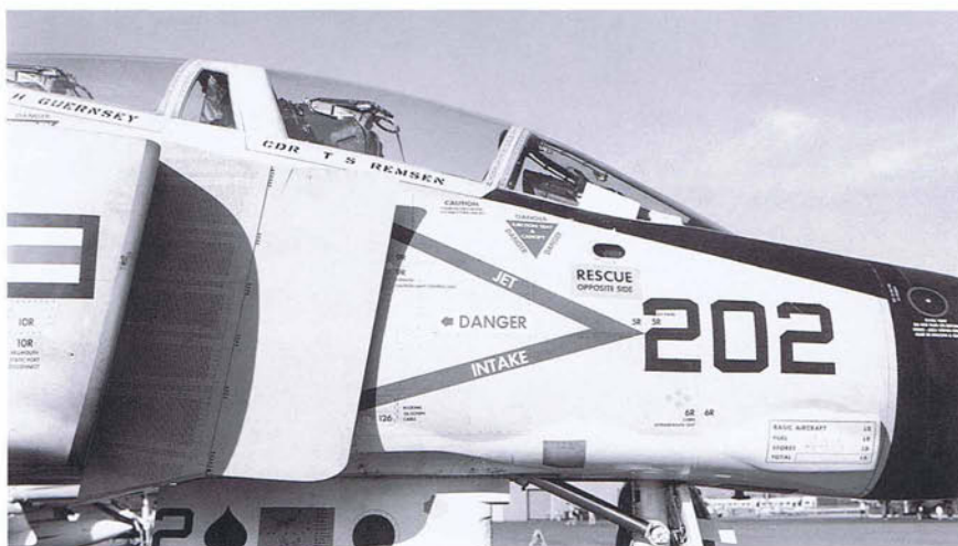
Left: Numerous servicing markings can be seen on this F-4. The placard of weights is for the catapult crew to know how much power will be needed to safely launch the aircraft. The legend on the radome is STATIC VENT DO NOT PLUG OR DEFORM HOLE - AREA WITHIN CIRCLE MUST BE SMOOTH AND CLEAN. Bottom: Notice the large area on top of each engine nacelle which have been painted Black due to the engine exhaust problem.
