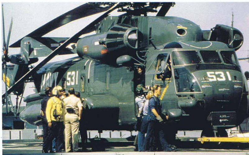
Left: Numerous service markings can be seen on the nose as well as on the folded tail rotor pylon of this CH-53.
