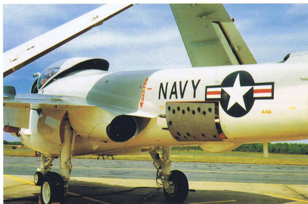
Above left: The demarkation between the Light Gray and Field Green of the land camouflage scheme is clearly evident on the VMO-8 Bronco. Left: The red warning markings around wheel doors, speed brakes, and flaps is clearly visible on this newly painted A-6A. Below: This QF-9 Cougar of VC-8 shows the distinctive paint scheme for a target aircraft in 1968.
