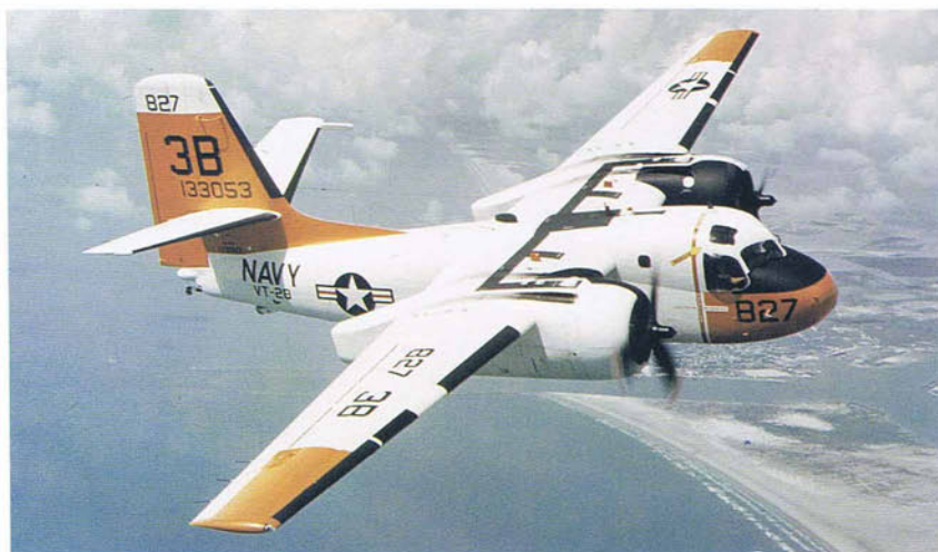
Left: In contrast to the high visibility scheme on this TS-2A, notice the large antiglare areas on the inboard side of the engine nacelles and the walkways on the upper surface of the wing, fuselage and engine nacelles. Below: While this UH-1E of VMO-6 is painted with the land camouflage scheme, the white lettering is highly visible. Bottom: Carrying BQM-34 Firebee target drones this DC-130A is painted in the colorful drone control scheme. Note the black areas of the under wing surface that are impinged upon by the engine exhaust.
