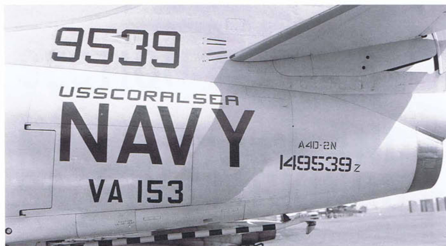
Left: The manufacturer's block designator has reached the end of the alphabet on this A4D-2N. Markings indicating the stabilizer position, which usually are not visible, clearly show as do the alternating black and white stripes on the tail hook. Bottom: Not all aircraft had as many visible maintenance markings as this F-4B which illustrates the volume of markings that could be found on an aircraft.
