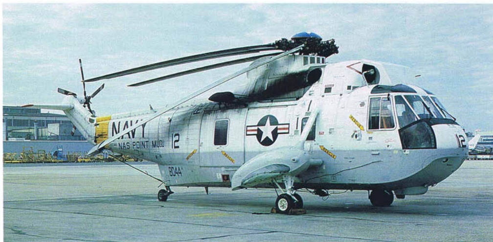
Left: The reason for painting areas black that are impinged upon by the exhaust is well illustrated by this SH-3G assigned to NAS Point Mugu. Below left: In contrast to the reduced visibility national aircraft insignia, the "Valions" (VFA 15) painted all other recognition markings so as to be clearly visible.
