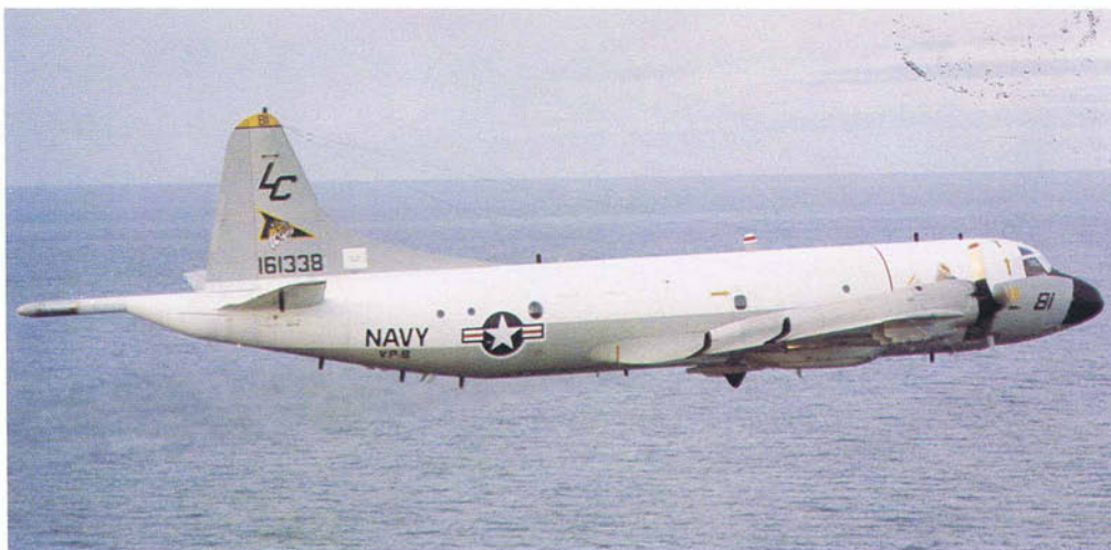
Left: The P-3C needed the solar reflecting white top to help keep the cabin temperature down for the crew operating all the electronic equipment. Bottom: One of the numerous paint schemes evaluated in 1988. Notice the Light Blue being used in place of red, yellow and white markings.
