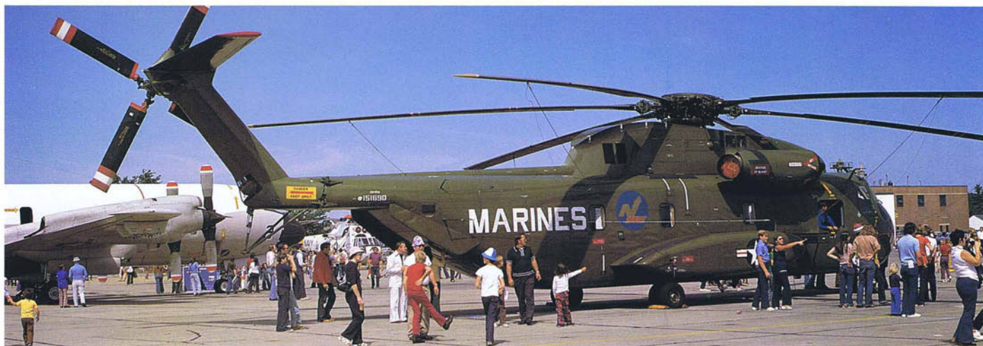
Above: The white stripes on the side of this CH-53A are guide lines to the various steps. Left: Helicopter Antisubmarine Squadron Light 31 carried numerous bright markings on the Engine Gray background. Below: This glossy Field Green CH-46F of HMM 263 shows all the colorful markings in effect prior to April 1977.
