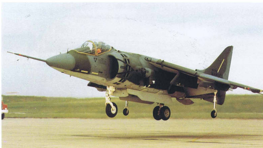
Left: The small national aircraft insignia on the fuselage of the AV-8B is painted in accordance with the tactical paint scheme requirements. Below: The national aircraft insignia on the wing of the AV-8A of VMA-513 is located as for a straight wing aircraft.
