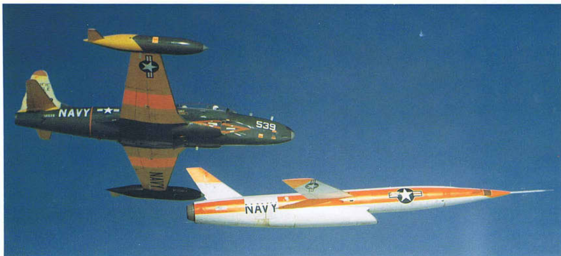
Left: This 1962 photo shows a slightly different drone control scheme on a Pacific Missile Range TV-2 with a Regulus II KD-2D guided missile.
