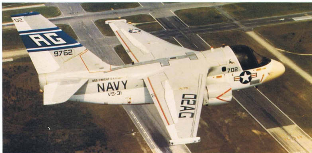
Left: The dark hard area walkway along the spine of this S-3A, is clearly visible against the lighter gray of the fuselage. Bottom: It is readily apparent on this A-7E that the rescue arrow points to a specific location such as the canopy release and not just to a general area.
