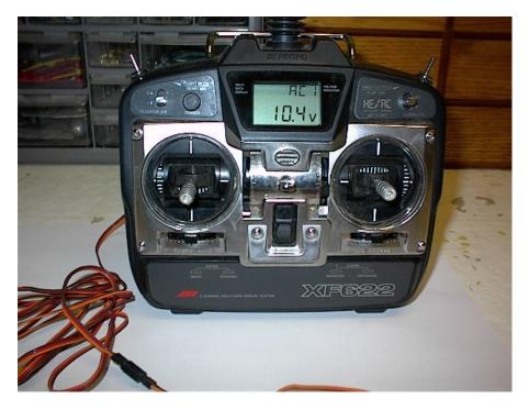
Photograph 5.11 -Typical JR computer radio with DSC. Toggles on top left and right are for retractable great landing gear, bomb drop. Left stick is used for throttle control. The right stick, which is normally used for elevator on RC models, can be used for flaps if the spring is removed. At the time of printing the XP652 was available.
