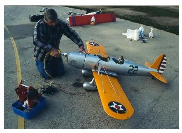
**Photograph 9.2** - Test run motor with handle, transmitter or servo plugged directly into the airplane. The lines have not been rolled out yet. Steve has brakes on this model. For additional safety you should have a friend hold the model while you start and adjust the needle valve.
