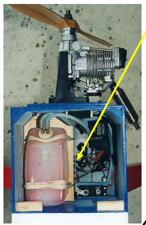
**Photograph 16.2** - This is the setup for my camera plane. Notice the stiff metal pushrod from servo that goes to the motor.
