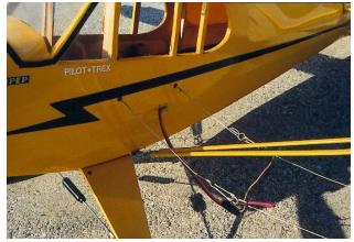
**Photograph 14.2** - Notice location of the bellcrank and landing gear location.
