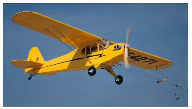
Plate #4- Fred Cronenwett's Fun Scale Hanger Nine Piper Cub 81" span, 9 lbs with Astro Geared 40 with 16-8 Propeller Astro Flight Super Gearbox, DSC electronic Controls This airplane can carry an 8mm video camera inside the cockpit!
