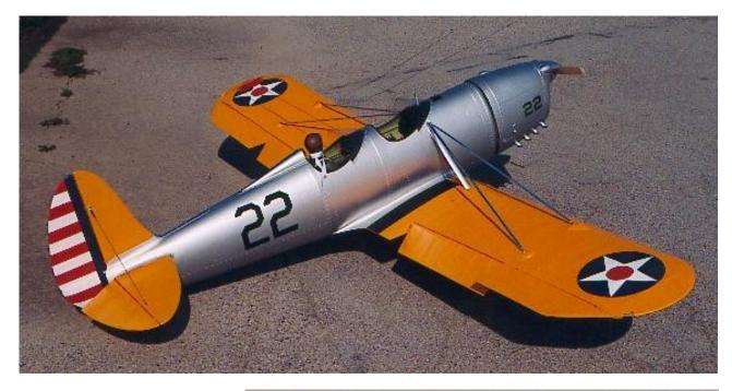
**Plate #21-** Steve Davis built this RYAN STA from the Byron Originals kit. 90" span, OS-90 four stroke for power. DSC electronic controls for flaps, brakes, steerable tailwheel and throttle control.
