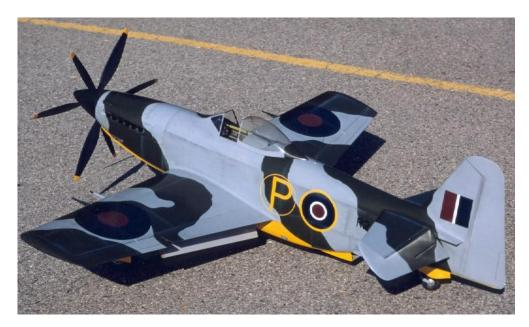
Plate #1 - Kieth Trostle's Precision Scale Martin Baker MB-5 Flaps, Throttle, Radiator Scoop, Rudder moves with Pedals Nationals 2000 Precision Scale Champion, 5 flying lines 55" span, .65 glow powered
