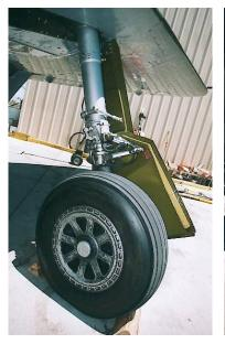
Inboard sides of landing gear leg showing wheel, strut and door detail
