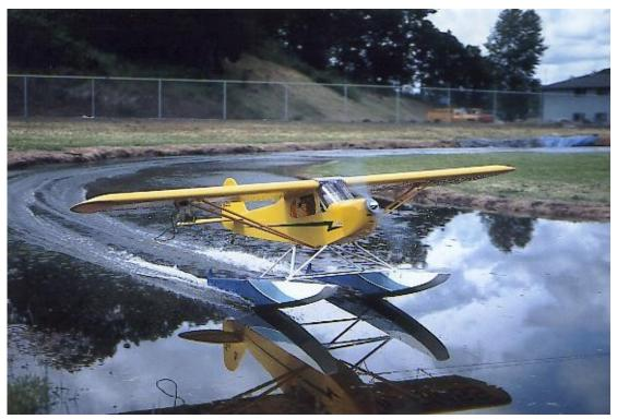
**Plate #19-** Grant Hiestand's Great Planes ARF cub taking off from the Roseburg, Oregon Floatpond powered with an Astro Flight 40 with super box and onboard video camera
