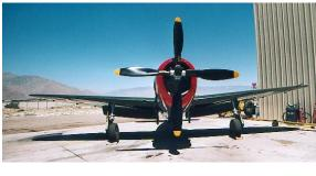
Propeller shape, wing dihedral, landing gear position can be determined by these photographs
