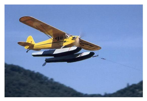
Plate #18- Author's Hanger Nine Cub with floats flying from the Roseburg, Oregon float pond. The floats were built from Great Planes float kit (balsa).
