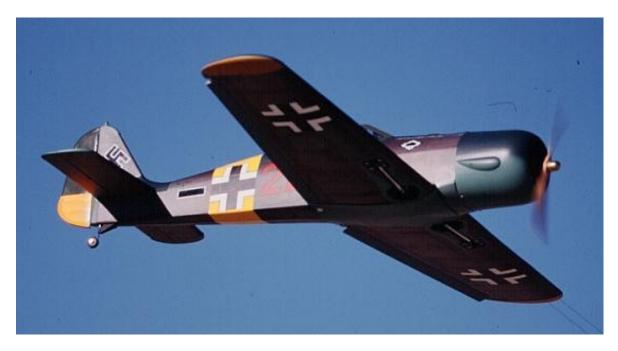
**Photograph 11.3** - Author's FW-190 from the Great Planes Almost Ready to Fly kit. This kit is no longer available. This model features flaps, bomb drop, throttle and retractable landing gear. Notice that the ailerons intended for radio control were used as flaps. This photo was taken when the model was being tested with an electric motor before the bomb drop unit and a .46 sized glow engine were installed.
