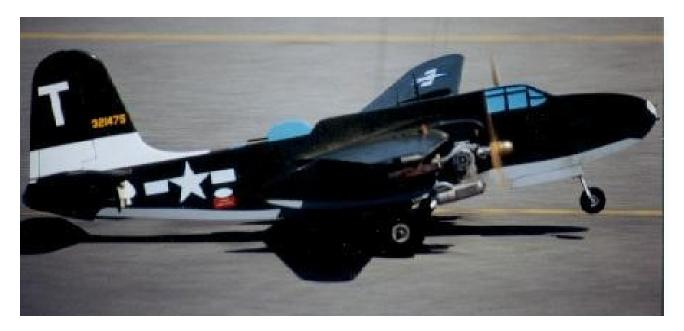
Photograph 17.1 - Author's 53" Span Scratch built Douglas A-20G Havoc Twin OS-20FP and Single Channel electronics Note main wheels touch first and then rotate to nose gear
