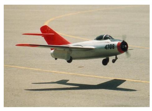
**Plate #12-** Flown by Merle Mohring, this Mig 15 was fast and a challenge to fly. You can see here is has a prop in the nose. You can't see the tuned pipe that runs thru the fuselage.
