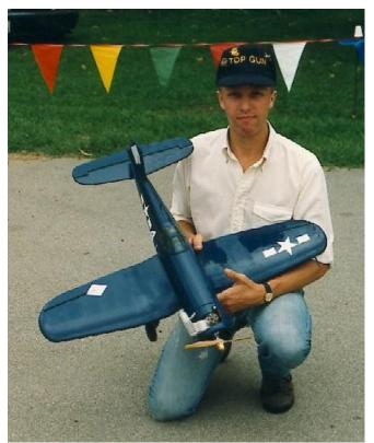
**Plate #10-** Fred Cronenwett with his 36" span Sterling Corsair in 1990, Single channel controls, monokote for covering. This model was powered with an OS-25FP. This model is so small the only thing that could be installed without making the model to heavy too fly was a throttle servo. The model weighed 3 lbs and flew on 52 foot lines
