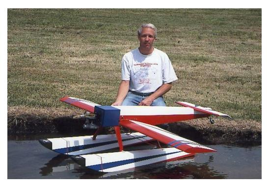
**Plate #6-** Fred Cronenwett with his scratch built Camera plane on floats. This model can be flown from water or land. 80" span, shown here with an ST-90, but has since been replaced with an OS-91 four stroke. DSC electronic controls. This is a wonderful test aircraft for motors, electronics, camera platform and other features.
