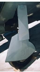
Outboard side of landing gear leg shows door detail
