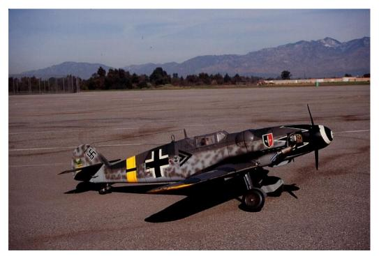
**Plate #5-** Merle Mohring's BF-109G built from the Innovative Kit with an OS-90 four stroke for power, retracts, flaps, throttle with multi-channel controls
