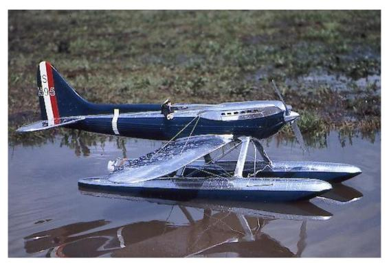
**Plate #16-** Supermarine S6B scratch built by Grant Hiestand. 51" span, F.A.I. 15 electric powered with DSC electronic controls. Grant carved his own plugs for the floats and fuselage to create the fiberglass fuselage and floats.
