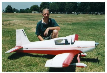
**Photograph 18.1** - Author's <sup>1</sup>/<sub>4</sub> scale Bravo flown in Sport Scale from the Sig kit. Powered with a Saito .91 four stroke, featured flaps and throttle using a converted Airtronics radio in as described in the Multi-channel chapter. This model weighed 17 lbs and spanned 87"
