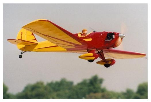
Plate #2 - Grant Hiestand's Precision Scale 1/3 Scale Spacewalker 103" span, Astro Flight 90 Geared Electric Motor, 18 lbs 1993 & 1995 Nationals Precision Scale winner 1995 NASA Flight achievement award winner
