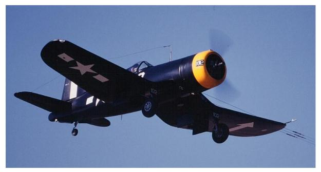
**Photograph 11.2** - Lynn Boss's F4U corsair built from the Royal Corsair SR kit that was intended and labeled as a Radio Control Kit. This model spans 63" and is powered with an OS-90 four stroke. This particular model uses a 3-line bellcrank for throttle control and features bomb drop with down elevator.
