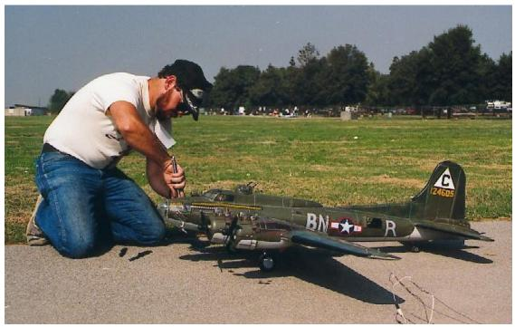
**Plate #8-** Merle Mohring is getting his Royal B-17F ready for flight. This model spans 77" and has four OS-26 four strokes for power. Multi-channel electronic control for throttle, retractable landing gear, rotating turrets and flaps.
