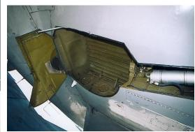
Interior of wheel bay also should be detailed, notice gear door and hydraulic piston that closes gear door.
