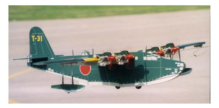
Plate #3- Merle Mohring's Scratch built Emily Flying Boat Control Line Profile Scale, OS-26 four strokes for power, 90" wing span Throttle & Flaps, Multi-Channel Electronic Controls
