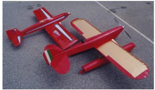
**Photograph 7.1** - Grant Hiestand's Venture 60 electric powered airplanes, the stock Venture 60 is on the left, the highly modified version was kit bashed to look like a Macchi MC-72 Schnieder cup Air Racer. Both models are powered with an Astroflight 40 electric motor and use electronic controls.
