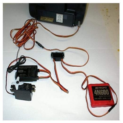
Typical DSC Set-up before going into the model airplane
